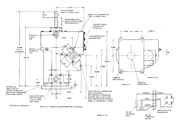
Typical Outline Drawing of 7.25-inch Hydraulic Amplifier (Do not use for construction)
