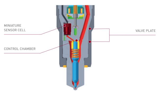
LOCAL INTELLIGENCE IS INTEGRATED INTO THE INJECTOR – WITH SIGNAL CONDITIONING AND PROCESSING COMPONENTS LOCATED ON OR CLOSE TO THE INJECTOR.
