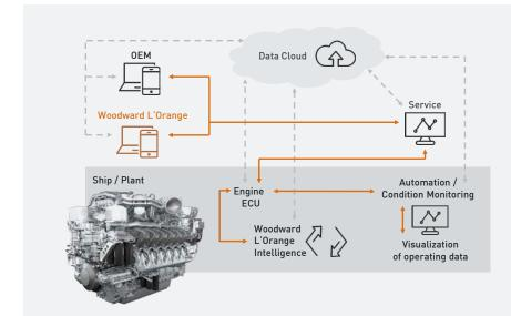
INCORPORATION OF AN INTELLIGENT INJECTOR INTO AN OVERALL SYSTEM: IT BEGINS WITH CONDITION MONITORING, AND ITS POTENTIAL FOR ENHANCED PERFORMANCE IS CLOSE TO ENDLESS.
