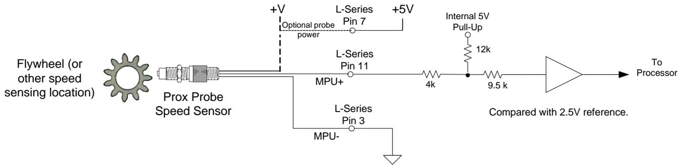
Figure 3-4. Proximity Probe Speed Sensing Input
