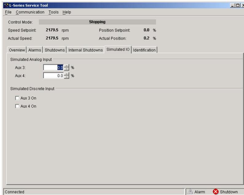
Figure 5-7. Service Tool—Simulated I/O Tab
