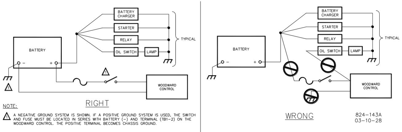
Figure 3-2. Correct and Incorrect Wiring to Power Supply
