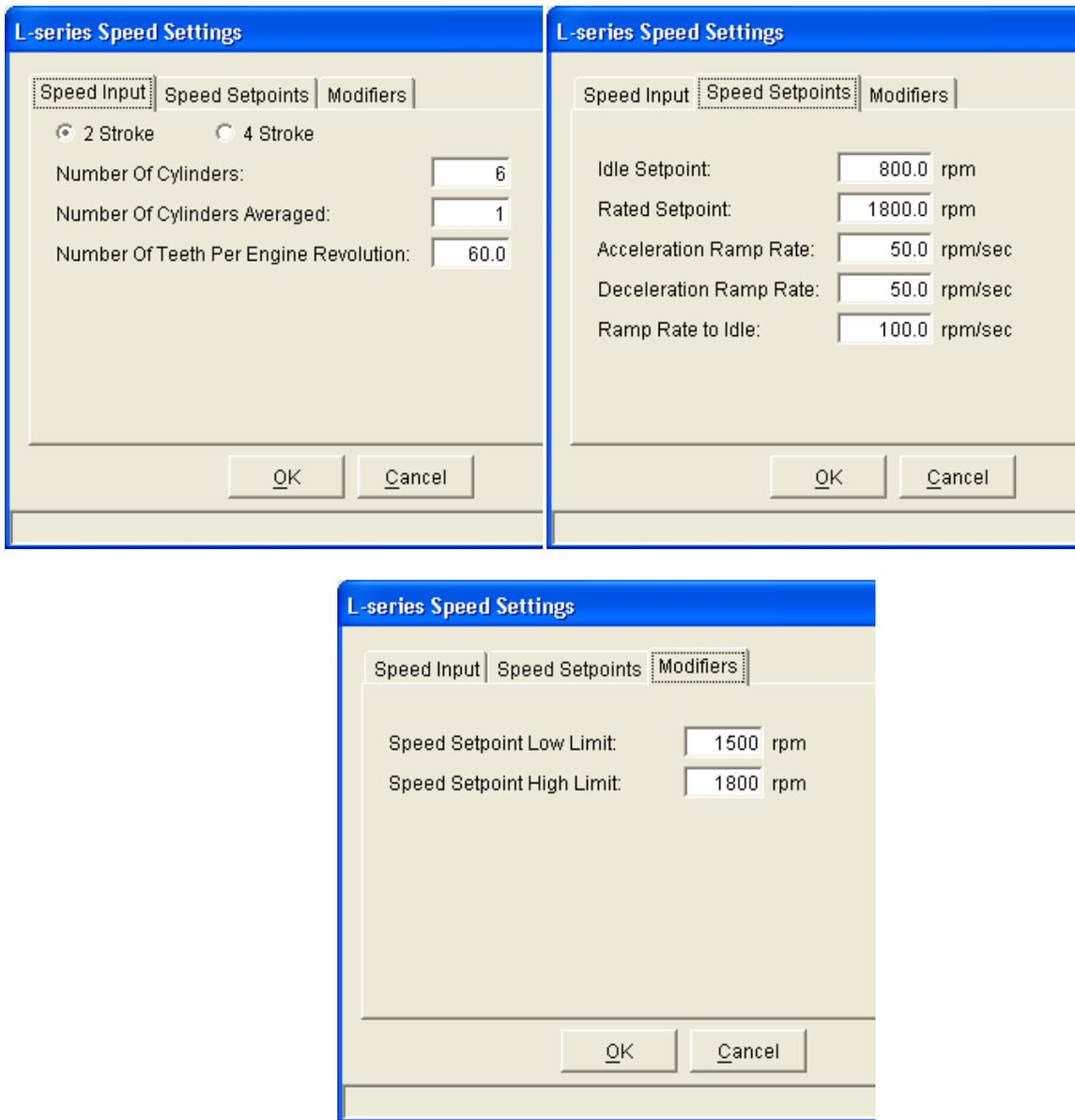
Figure 7-2b. Speed Input Window (5418-1680 software version)
