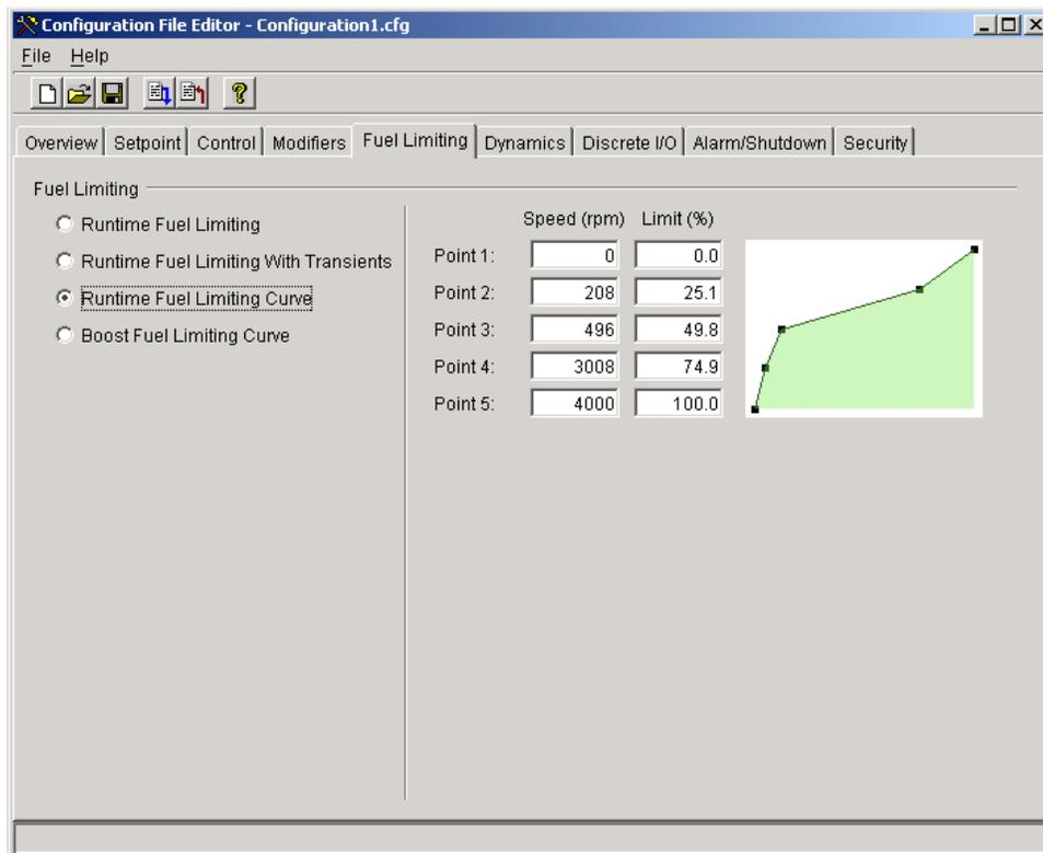
Figure 6-6a. Configuration Editor—Fuel Limiting Tab
