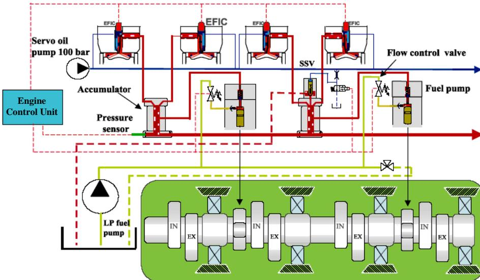
The Woodward LCR (large common rail) fuel system is modular, with sub-systems designed to serve engines with from four to 18 cylinders. The system is based on a camshaft-driven high-pressure pump and an accumulator for every two cylinders. The accumulators are connected together by the common high-pressure fuel rail, and connections from every accumulator feed the injectors of two cylinders.
