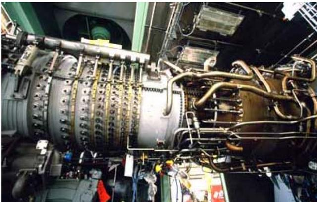
The 40,500 shaft horsepower LM2500+ is GE's newest aeroderivative gas turbine. Based on the design of the GE LM2500, this machine delivers up to 25% more power at a simple-cycle thermal efficiency in excess of 39%. It is designed to achieve reliability equal to the
