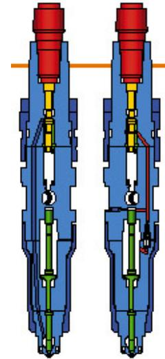
Pressurized engine oil is used in the injectors to generate the necessary forces for high-pressure injection. This injector design is capable of operating at fuel pressures of 2000 bar, while providing crisp injection starts and stops.
