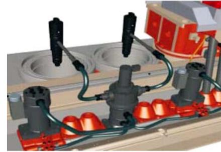
Each cylinder has a solenoid-operated fuel injector that is electronically controlled to match injection pressures, timing, and profile to the speed and load of the engine. Combustion is optimized under each loading condition to minimize emissions and smoke, and increase engine fuel efficiency.
