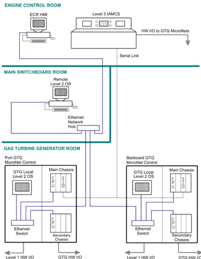
As in other commercial marine applications, the MicroNet controls on the QM2 use an aggressive control algorithm developed by Woodward especially for gas turbine-powered cruise ships, giving the gas turbines the responsiveness needed to meet the load acceptance and rejection requirements of the classification societies.
