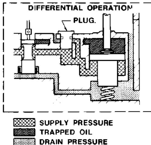
Figure 3-2. Schematic of Hydraulic Amplifier
