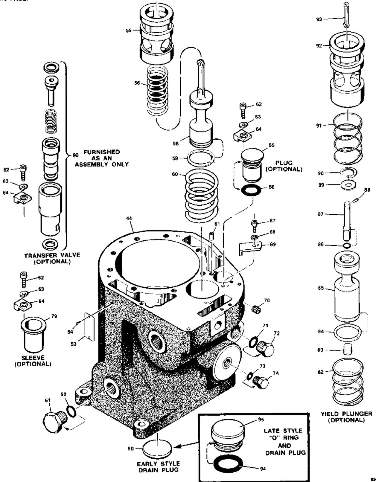
Figure 5-1b. Parts for Electrically Controlled Hydraulic Amplifier (sheet 2)
