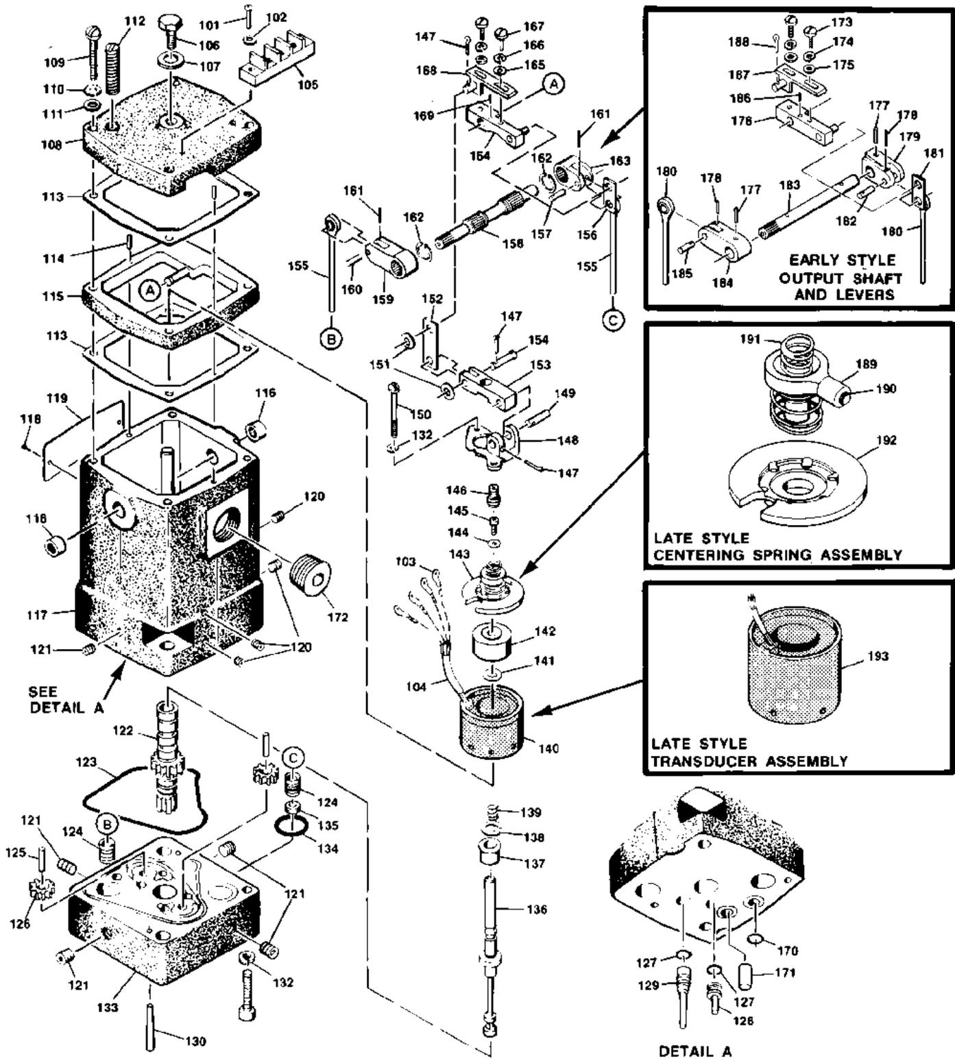
Figure 5-2. Parts for EG-3P Actuator
