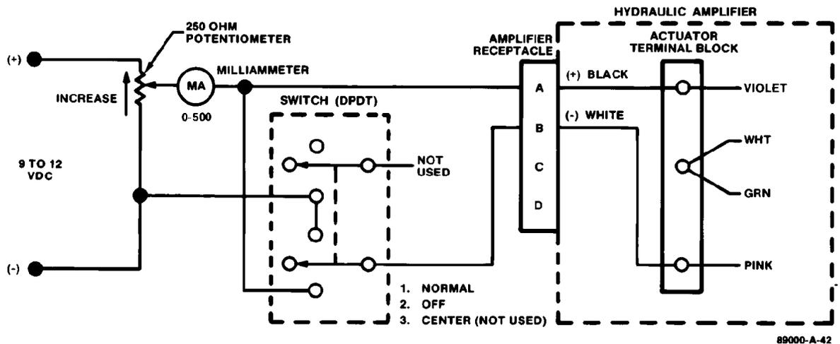
Figure 4-1. Test Circuit for the Hydraulic Amplifier
