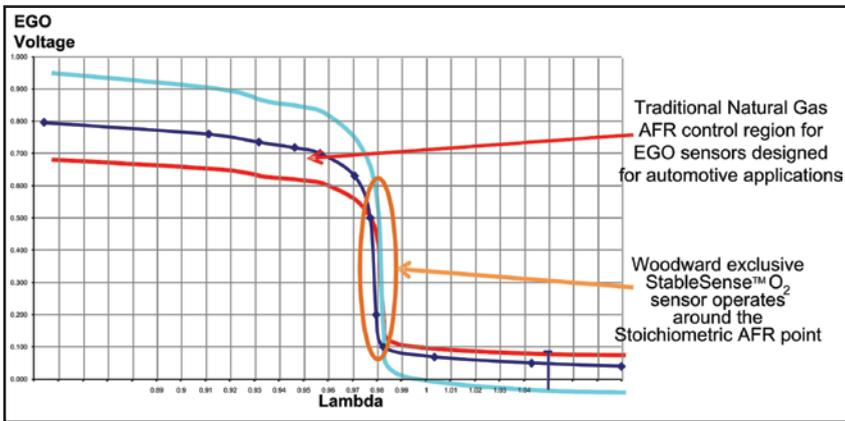
Figure 6. With StableSense, the operating point for emission control is on the vertical part of the sensor's voltage curve.
