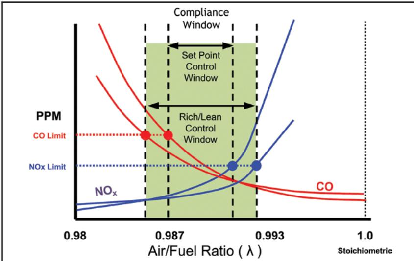
Figure 7. Better oxygen management allows an engine to stay in compliance for years without readjustments.
