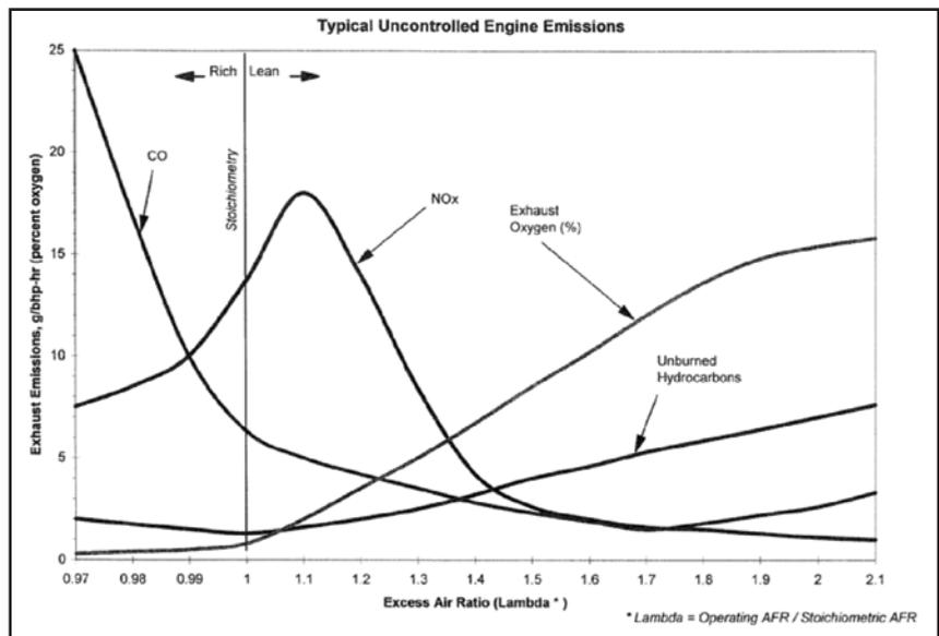
Figure 1. Components of engine exhaust compared to  $\lambda$
