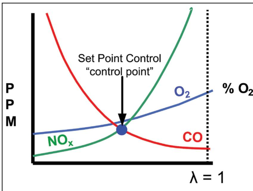
Figure 3. The control setpoint is established at the intersection of the CO and NO<sub>x</sub> curves.
