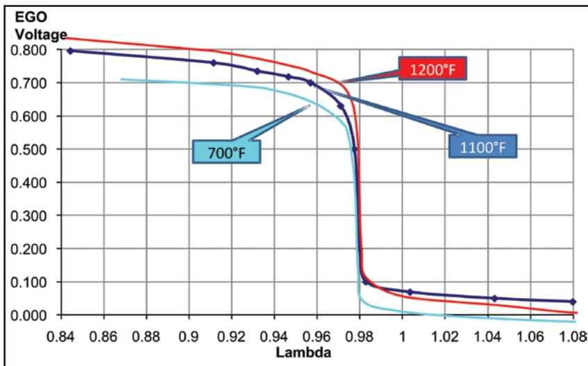
Figure 4. Lambda can vary depending on the exhaust gas temperatures.
