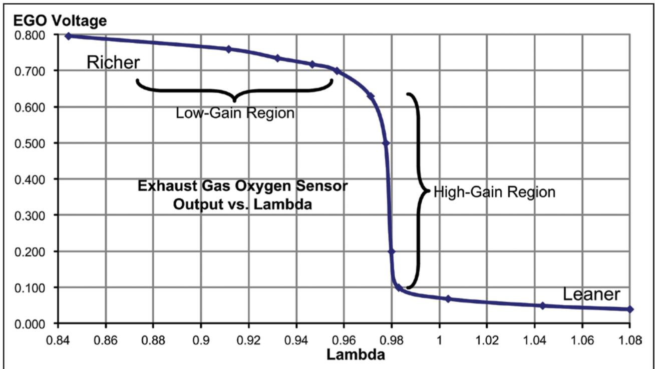
Figure 2. Oxygen in exhaust gas, scaled in lambda, as a function of the output voltage
