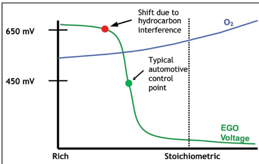
Figure 5. Methane in exhaust can cause sensing point to shift.
