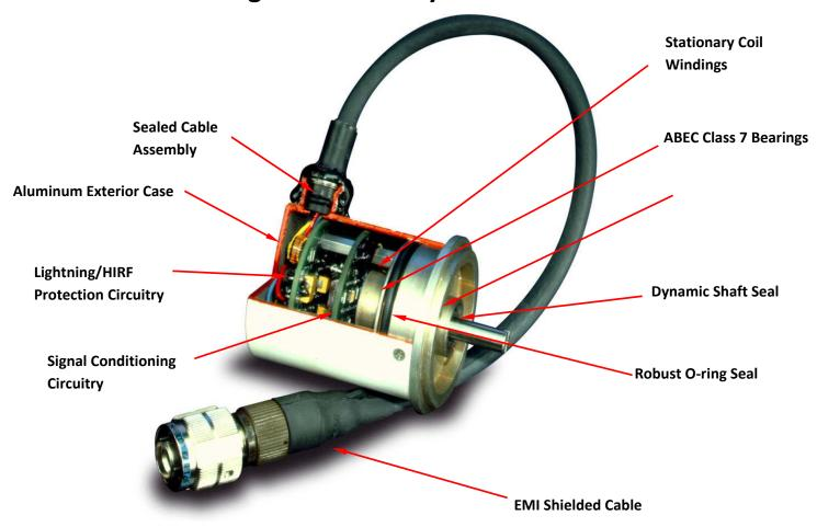
Woodward's RVDT-based position sensors were developed for control surface and flight control input applications as drop-in replacements for failure-prone potentiometer and RVIT-type sensors. The no-wear, solid-core construction of Woodward's RVDT sensors have been proven in numerous demanding flight control applications as having uncompromising reliability—resulting in reduced down time and life-cycle costs.
