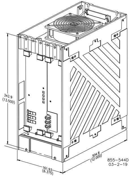
MicroNet TMR® Power Supply Chassis (Do not use for construction)
