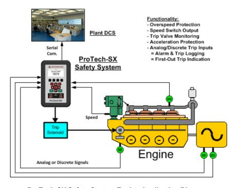
**ProTech-SX Safety System Engine Application Diagram**
