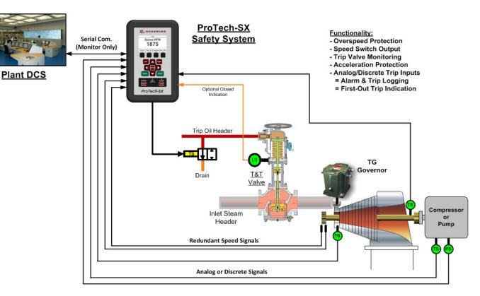
**ProTech-SX Safety System Turbine Application Diagram**
