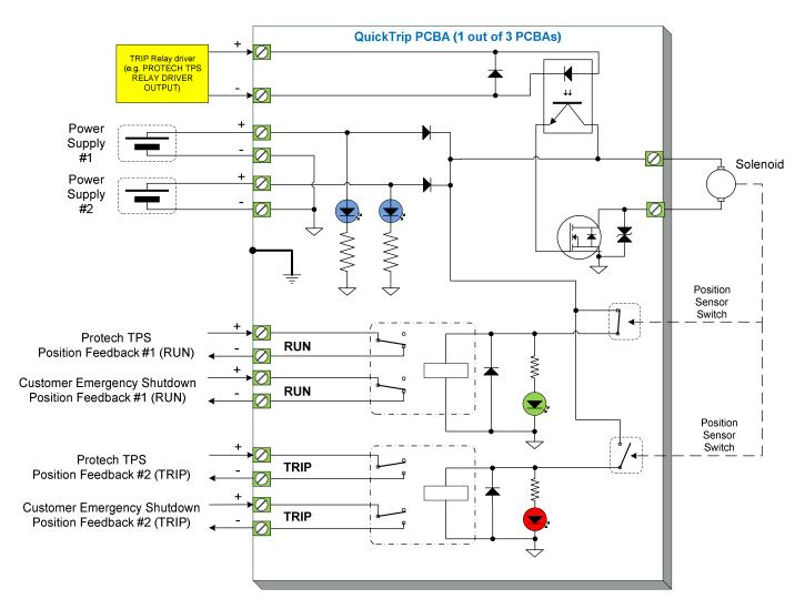
Figure 4. QuickTrip Module Electrical Schematic
