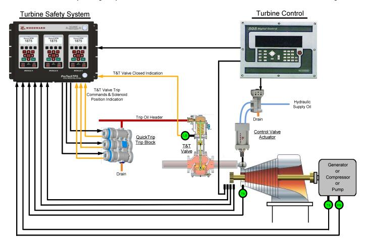
Figure 1. Typical QuickTrip Application
