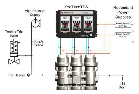
Figure 3. Turbine Safety System Interconnection Diagram
