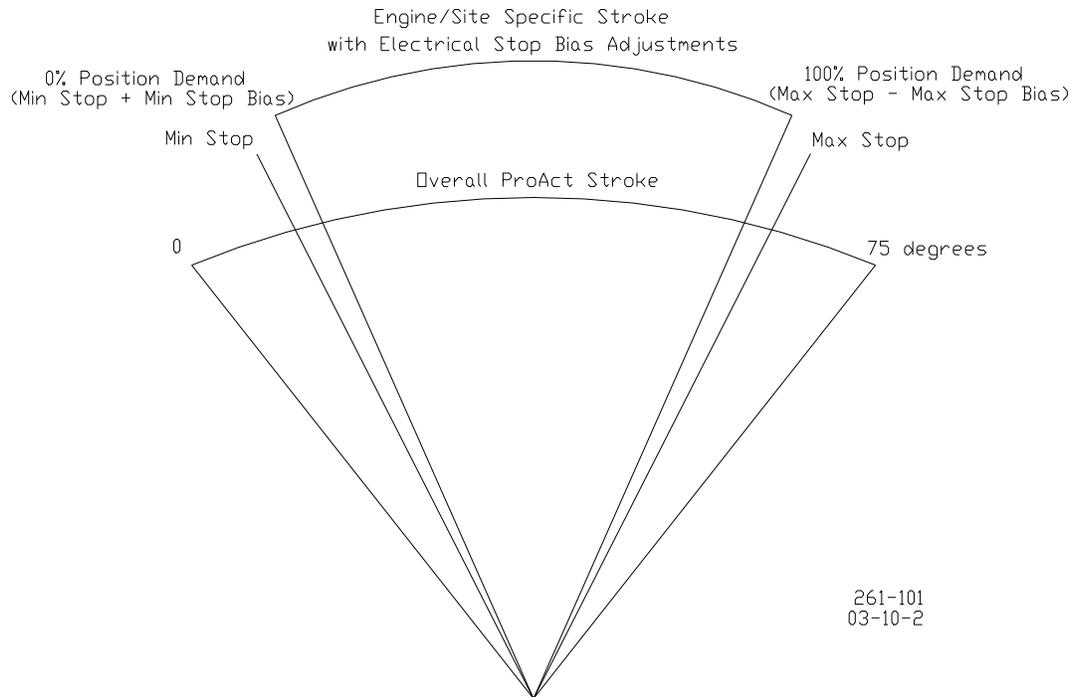
Figure 7-1. Electrical Stop Adjustments Relative to the Mechanical Min and Max Stops
