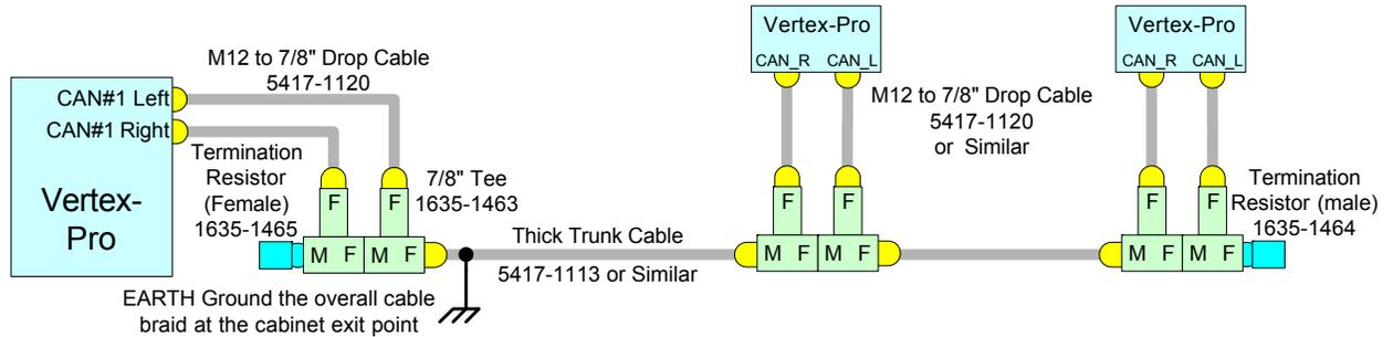
Figure 5-11—CAN Communication Connection Example
