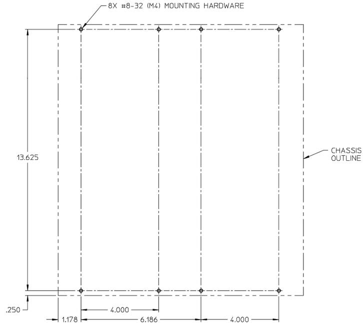
Figure 3-4—Mounting Template of MicroNet Plus 8-Slot I/O Chassis
