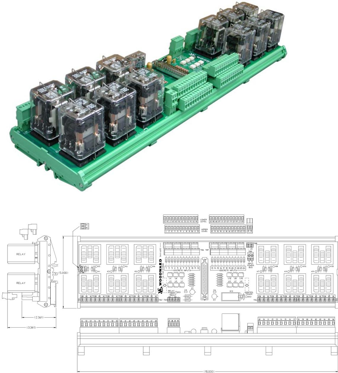
Figure 8-5—24/12 Discrete Module Outline Dimensions
