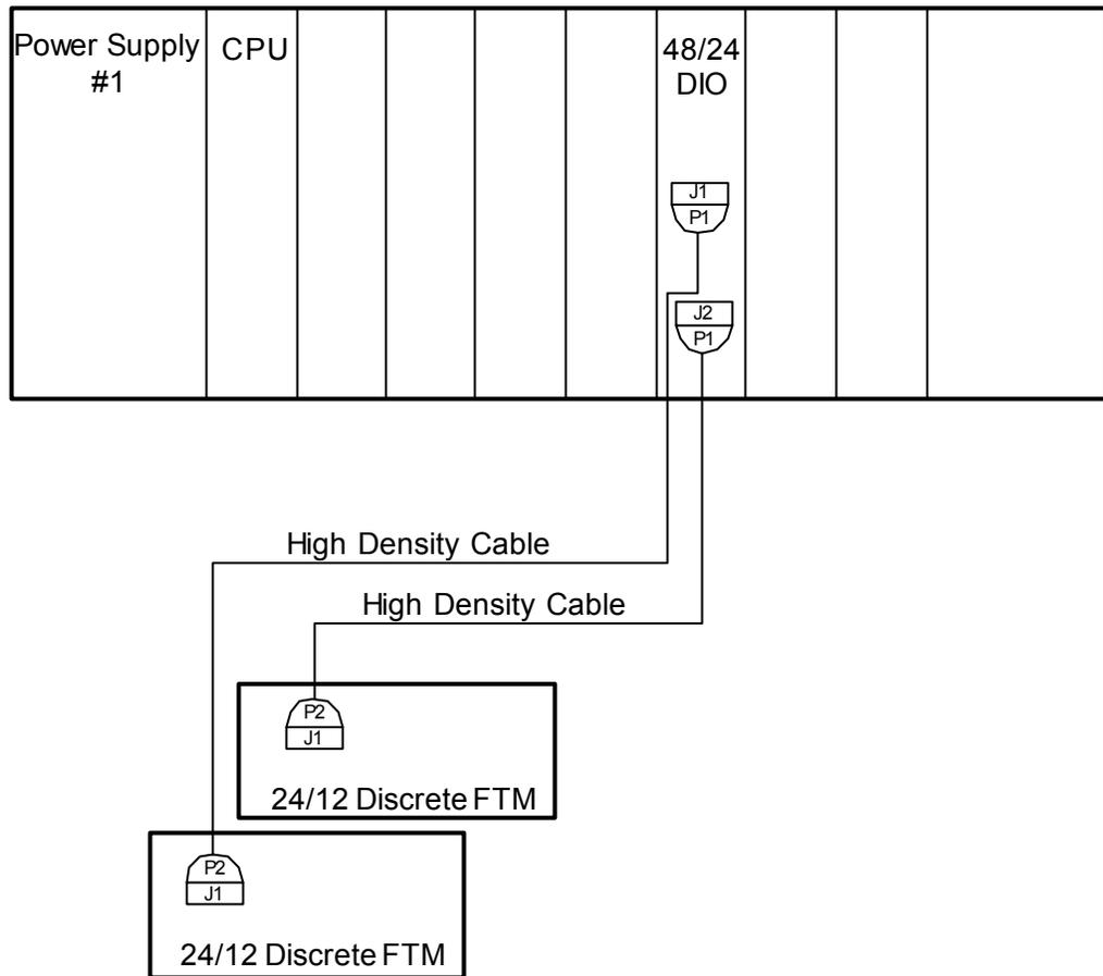
Figure 6-2—Configuration 2, Two 24/12 Discrete FTMs
