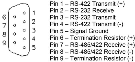
Figure 5-3—CPU Communications Port (DB9F)
