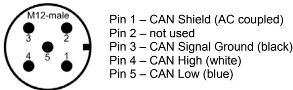
Figure 5-10—CAN Communication Ports (M12 male)
