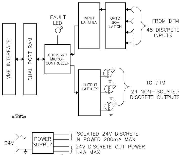
Figure 6-5—48/24 Discrete Combo Module Block Diagram
