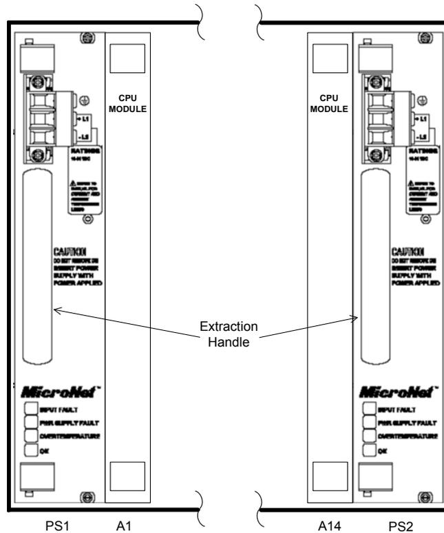
Figure 9-1—MicroNet Power Supply
