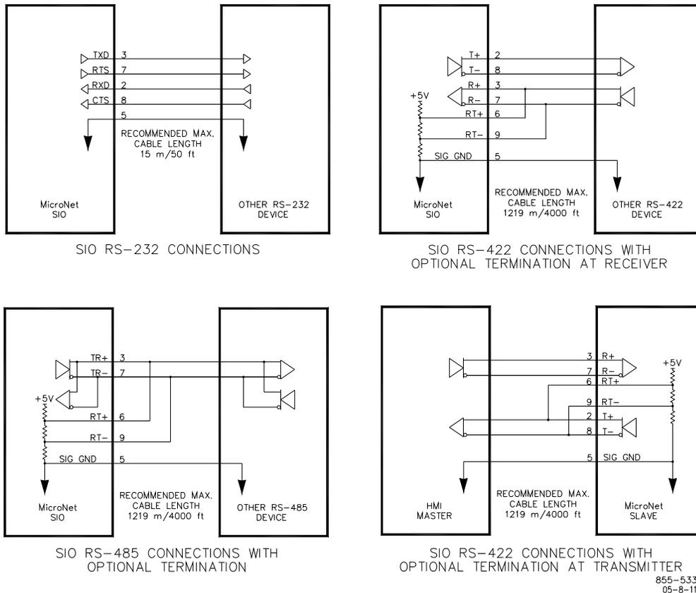
Figure 5-6—Termination and Cable Connection Examples
