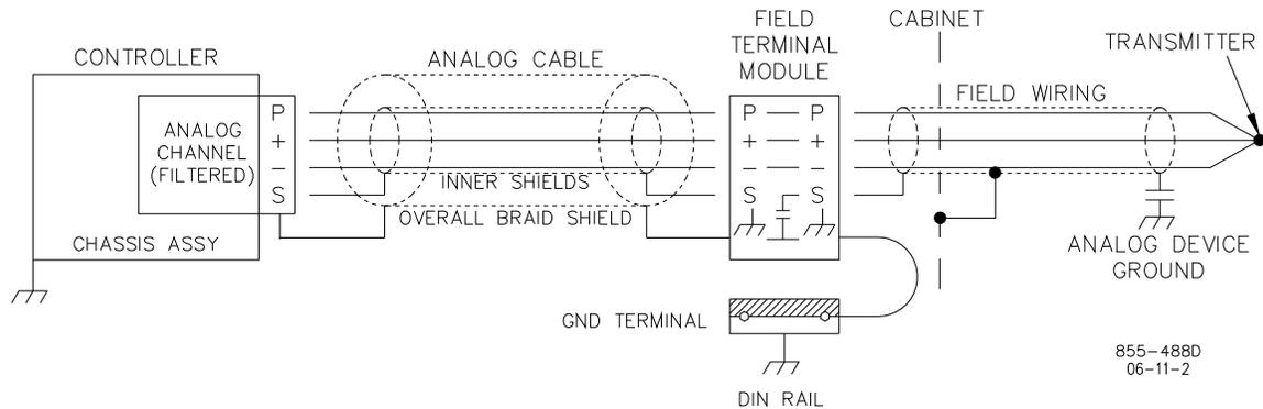
Figure 9-3—Shield Termination Diagram Example
