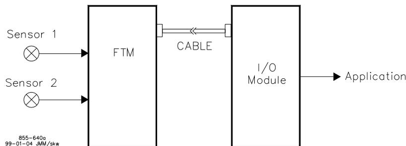
Figure 2-3—Redundant Sensors
