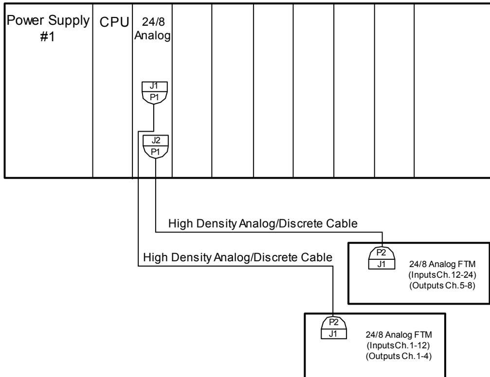
Figure 7-2—Simplex System Configuration Example
