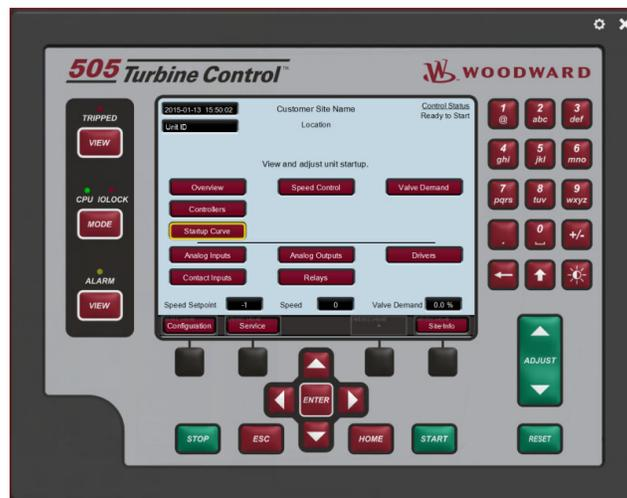
Figure 5-22. HOME Menu Showing "Startup Curve" IN-Focus
