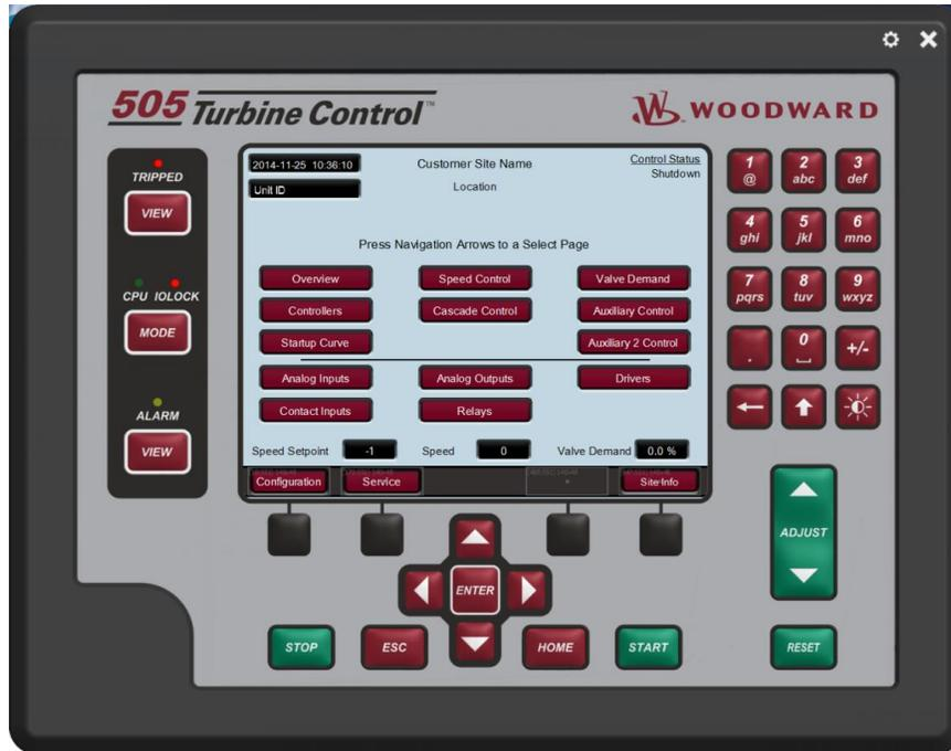
Figure I-17. Remote View Tool (Default Setting) after Opening from the Configuration Window
