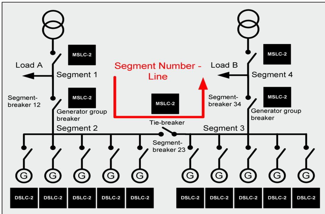
Figure 3-5. Isolated / Utility Parallel Operation with Multiple Generators, Tie-Breakers and Generator Group Breaker
