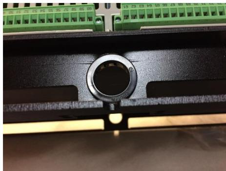
Figure 1-5. Grommet for Wire Thru-Hole
