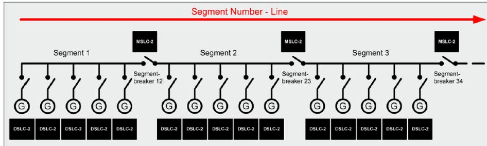
Figure 3-3. Multiple Generators in Isolated Operation with Tie-Breaker
