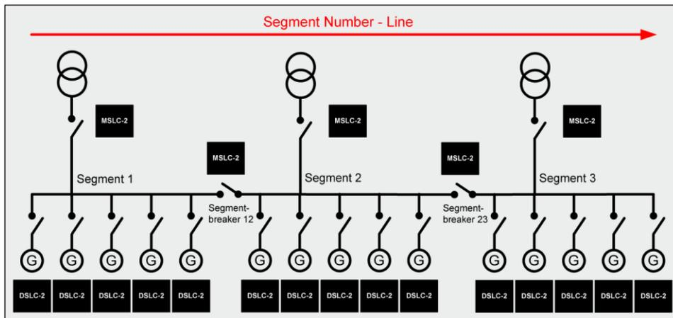
Figure 3-4. Multiple Generators in Parallel Operation with Multiple Utility Ties and Tie-Breakers
