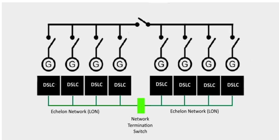
Figure 3-2. Multiple Generators in Isolated Operation with Tie-Breaker
