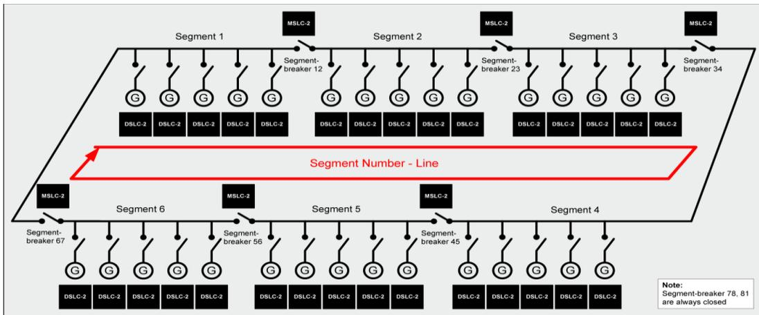
Figure 3-6. Isolated Operation with Multiple Generators and Tie Breakers (Ring Option)
