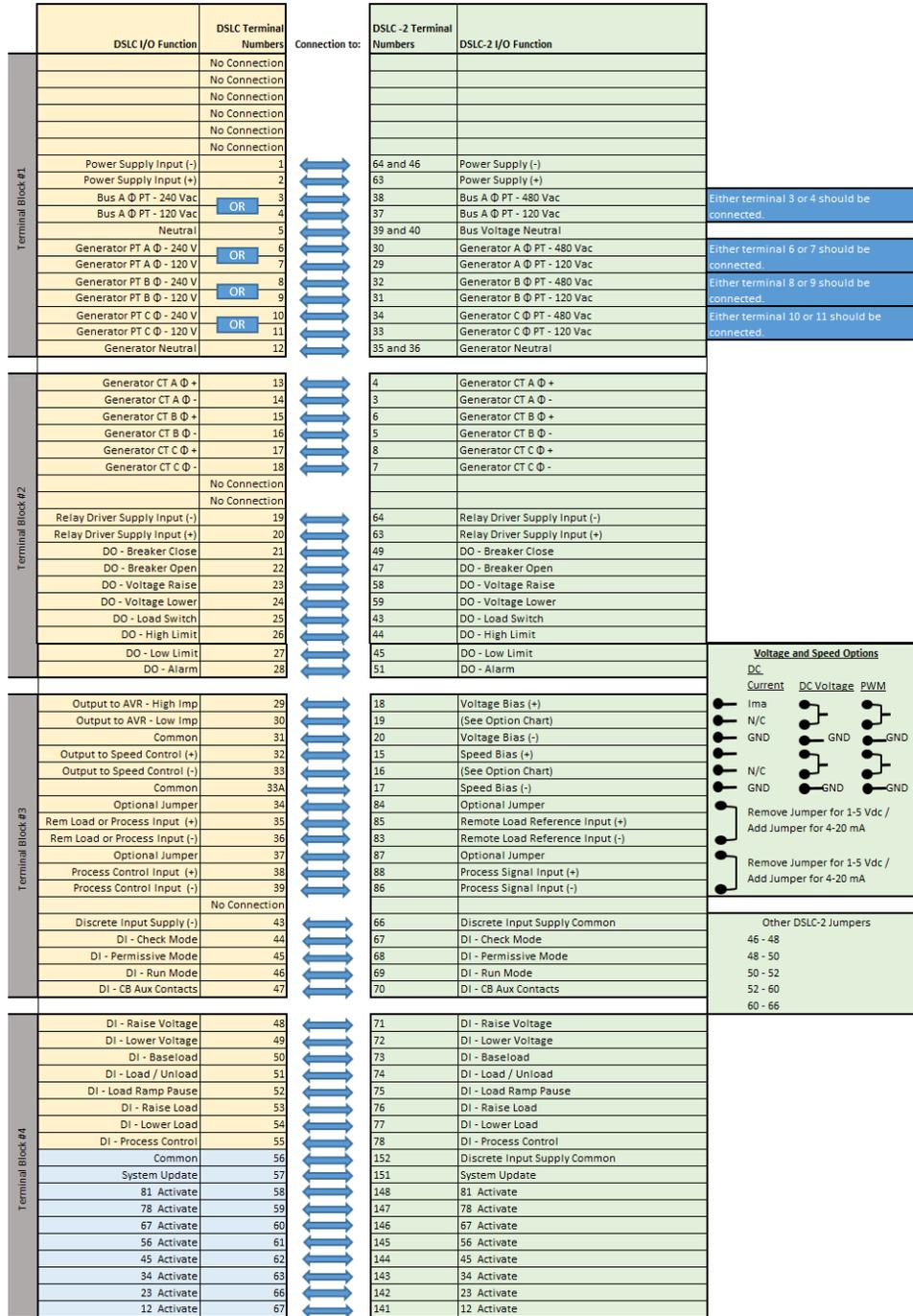
Figure 2-2. DSLCL 120 V or 240 V WYE Connected Version
