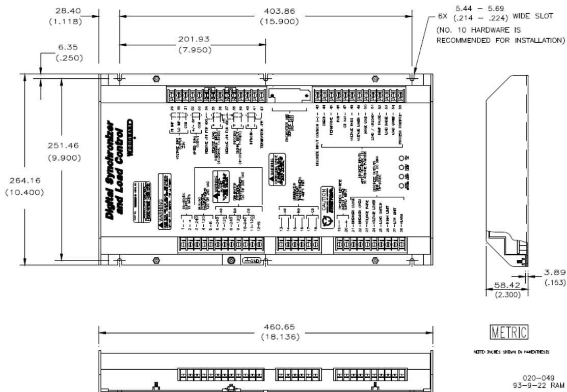
Figure 2-1. Mounting Hole Pattern and Dimensions of Original DSLCL
