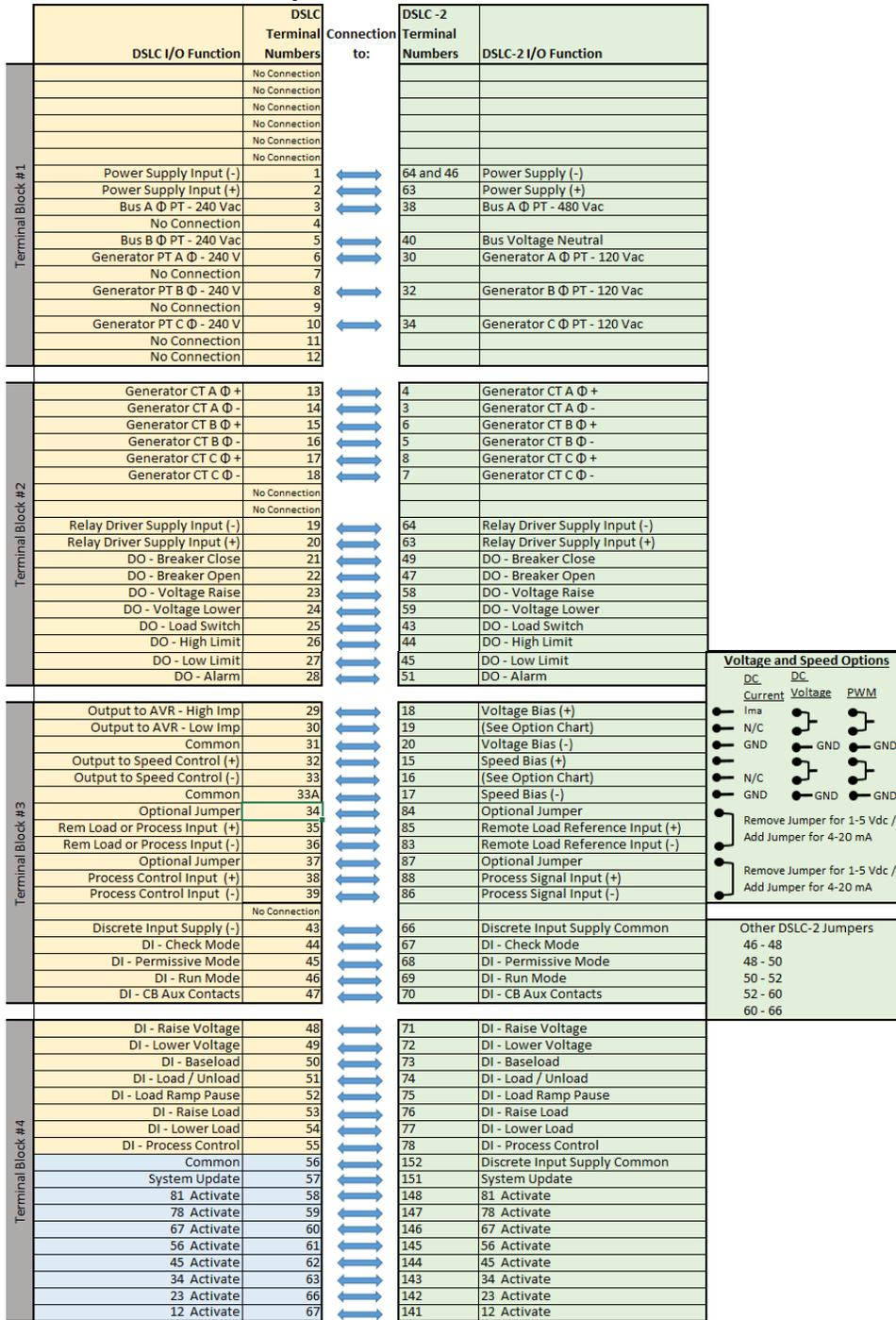
Figure 2-4. DSLCL 240 V Open Delta Connected Version
