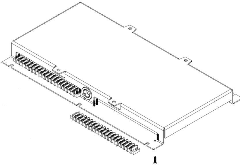
Figure 1-2. Sheet Metal Layout with Terminal Blocks
