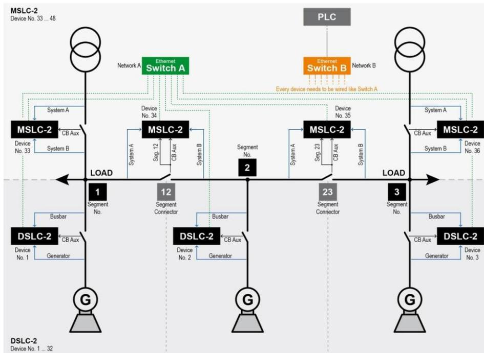
Figure 3-1. One Line Diagram with Network Switches Example
