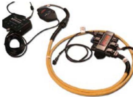
6. The boot key is not needed for normal programming or calibration so it can be set aside. Errors in configuration, logic and/or other programming made during program development (via .srz file) can cause a persistent loss of CAN communications with the module under development. If this happens, apply the boot key to force the module into reboot mode, reloading the module with functional program code (a known, valid .srz file) in order to allow resumption of module communication.
