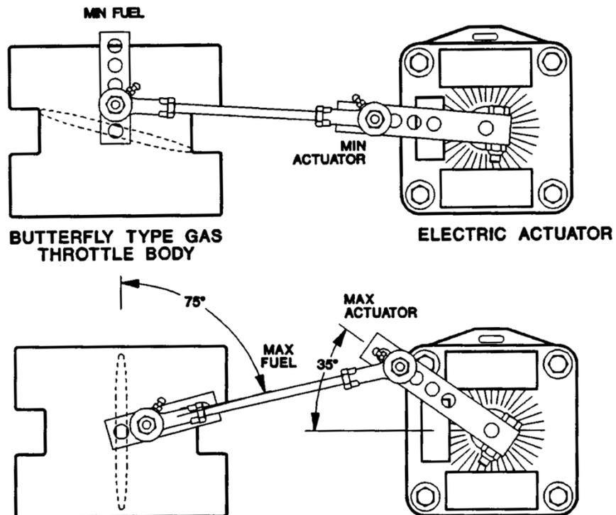
Figure 3-3. Linkage for Non-linear Installations
