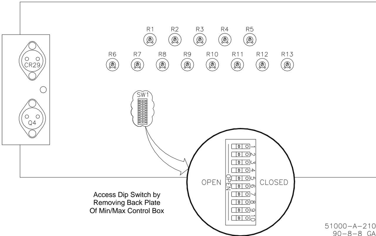
Figure 3-1. DIP Switch Location on Other Side of Printed Circuit Board
