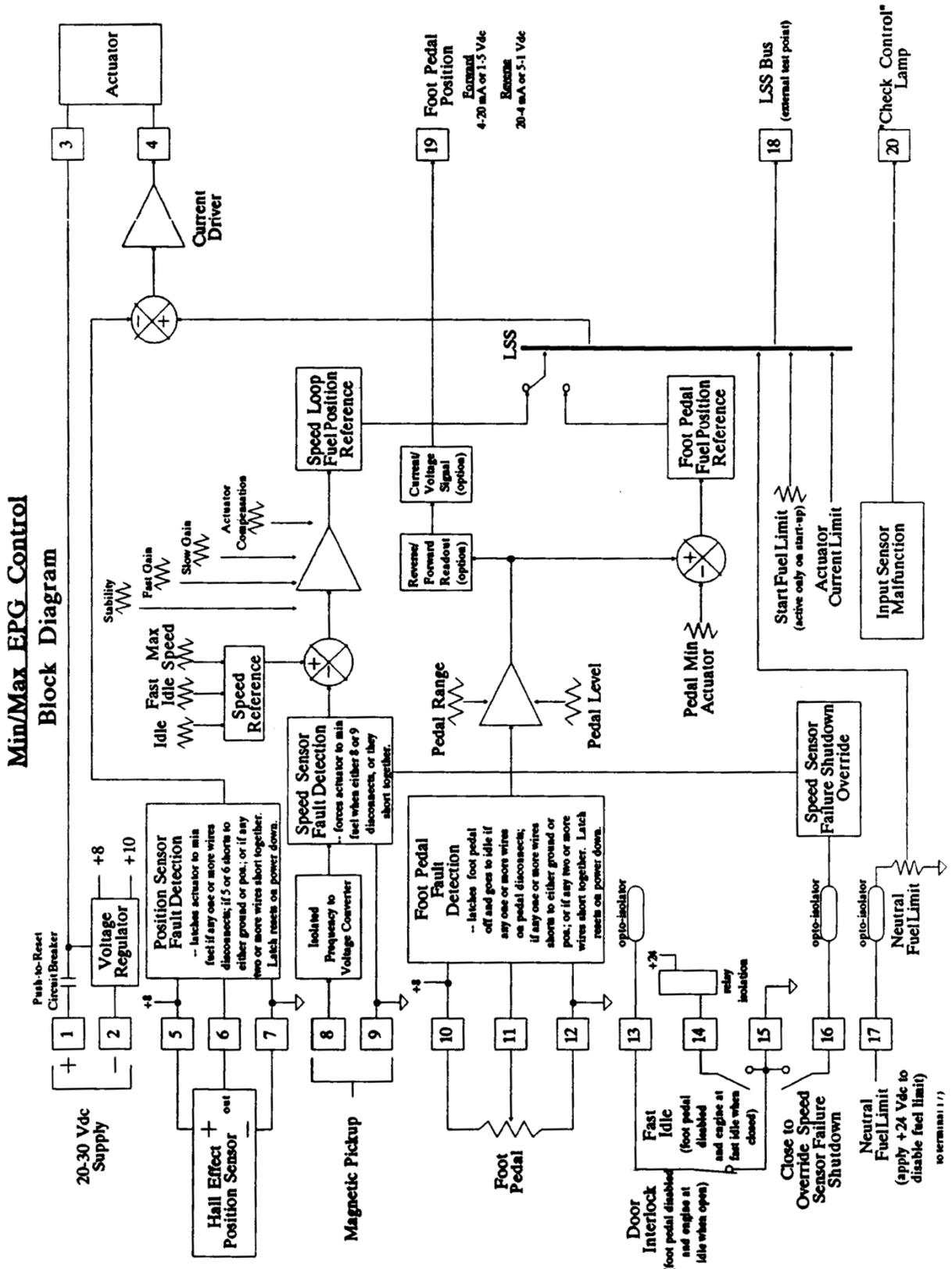
Figure 5-1. Min/Max Control Block Diagram
