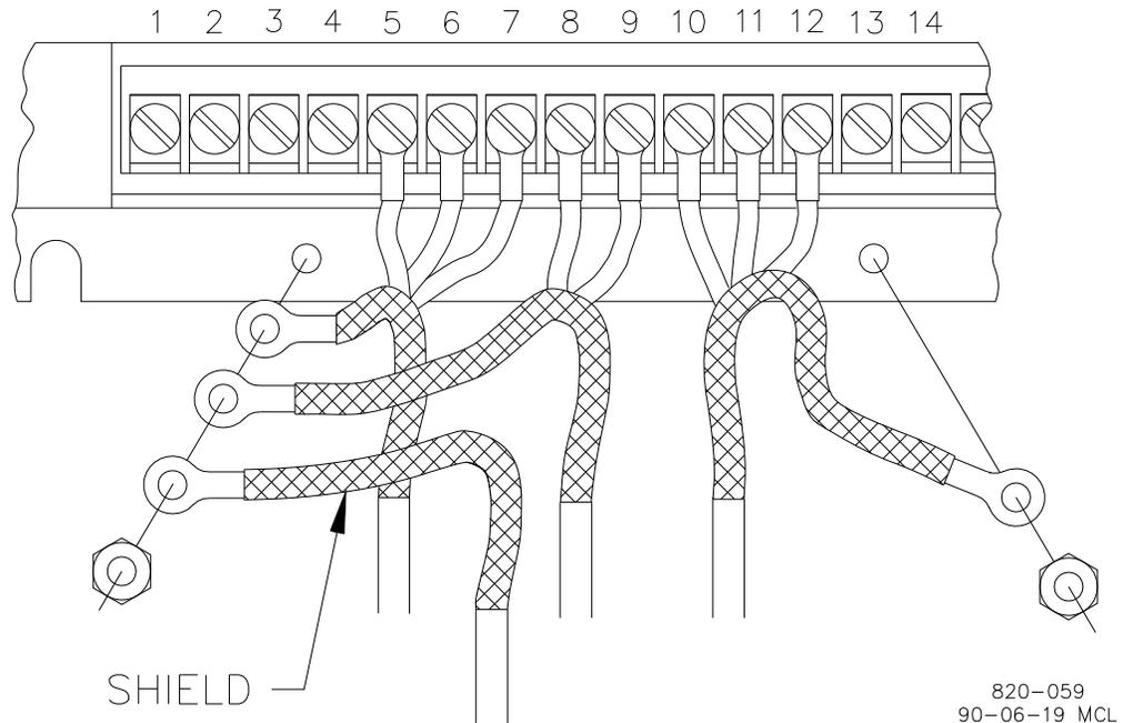
Figure 3-4. Proper Preparation of Shielded Wires
