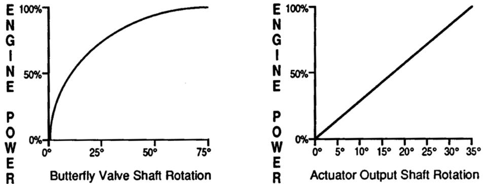
Figure 3-2. Effect of Butterfly Linkage
