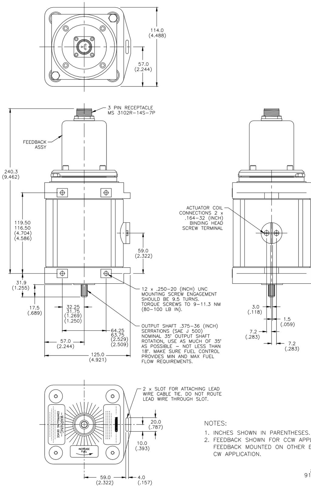
Figure 3-7. 1724 Electric Actuator
