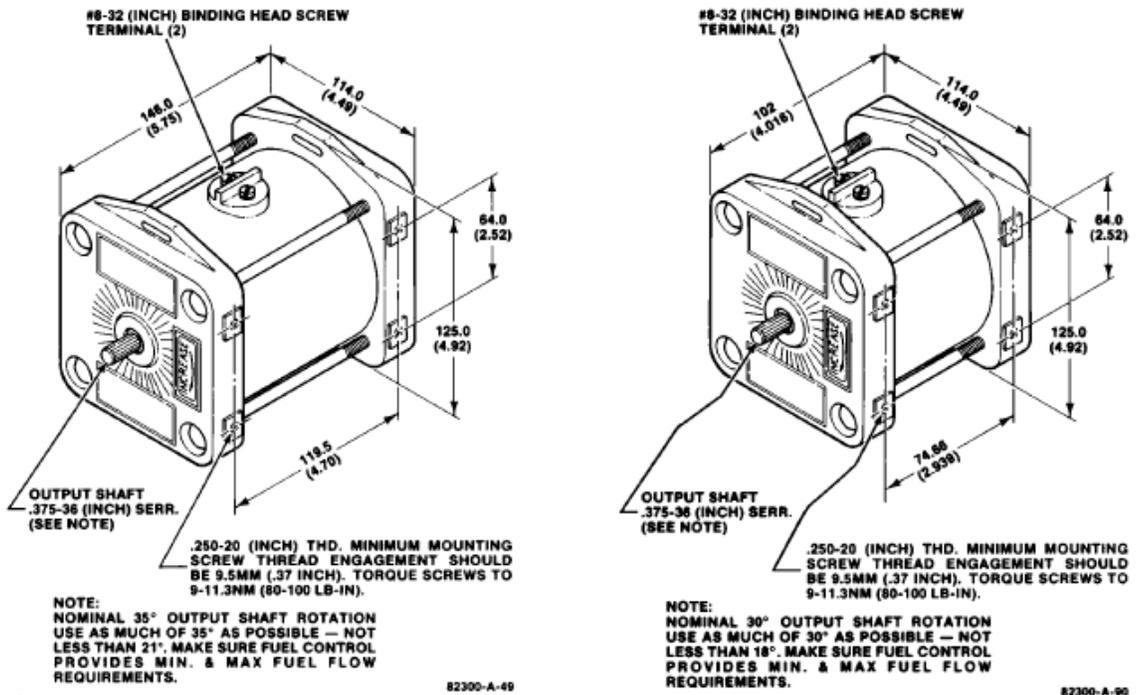
Figure 1-3. Outline Drawing for EPG 1712/1724 and 512/524 Actuators
