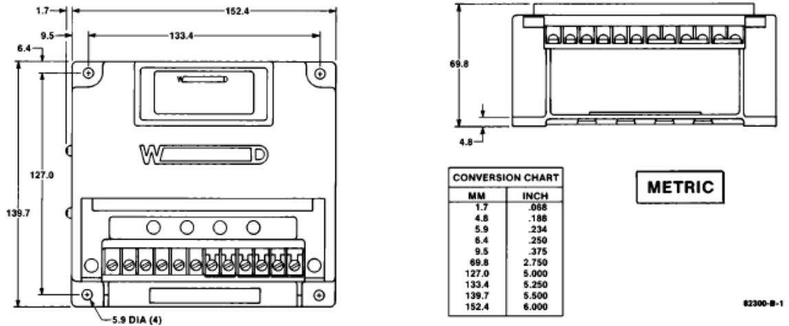
Figure 1-2. Outline Drawing for EPG 512/1712 and 524/1724 Speed Controls
