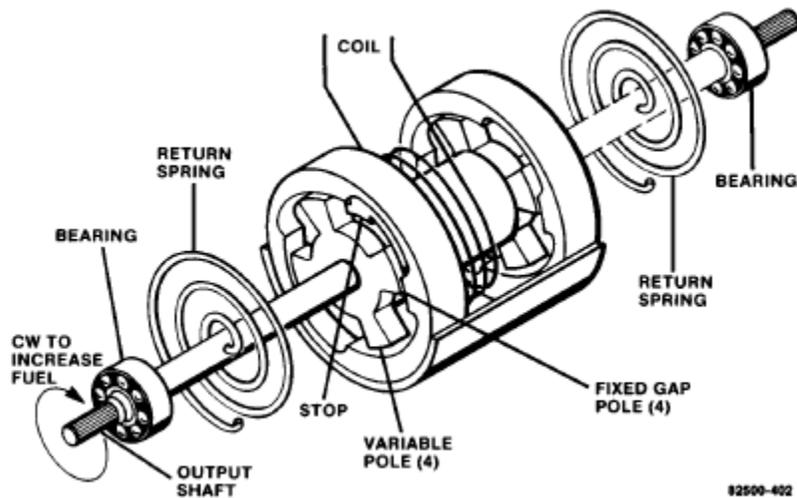
Figure 4-2. Actuator Schematic
