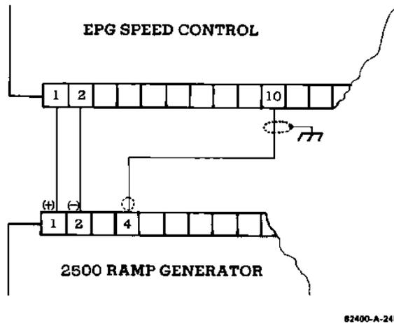
Figure 2-7. Typical Wiring to 2500 Ramp Generator
