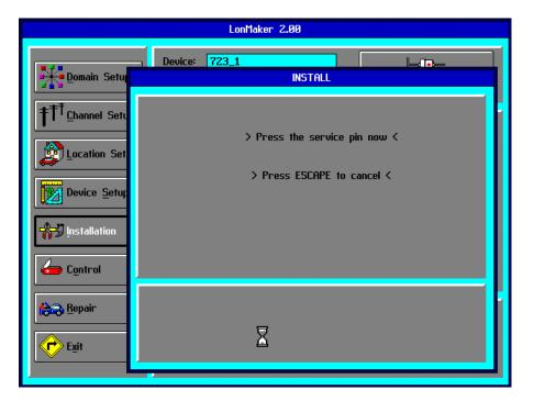
Go to the control and select the service pin. On a 723, the service pin can be found in the service menus. Refer to the corresponding 723 manual for details on the service pin location. The 723 service pin will have to be tuned to TRUE and then back FALSE. The service pin on a DSLC control is in menu 5, and the configuration key will have to be set to 49. The LSIM has a physical service button located above terminal 11.
