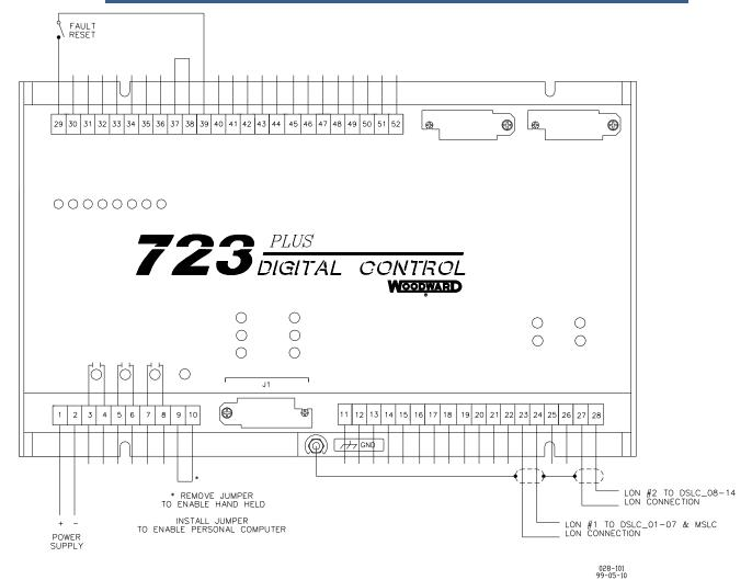
Figure 1-5. Typical 723PLUS Connections
