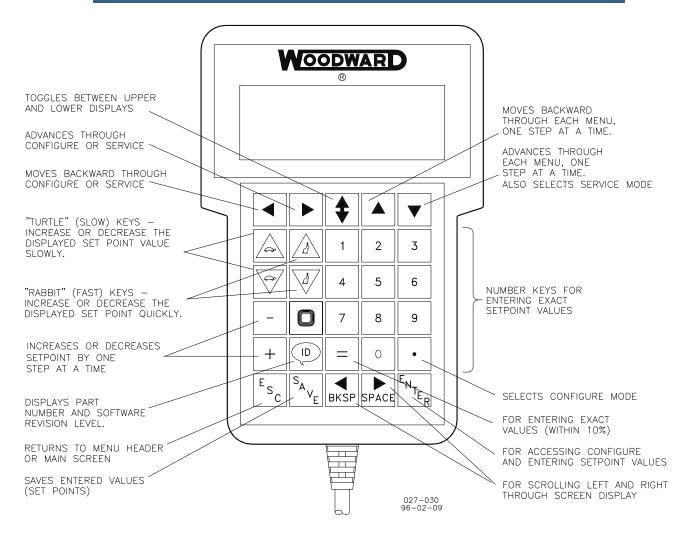
Figure 3-1. Hand Held Programmer Functions
