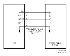
Figure A-1. 723PLUS RS-232 Connections
