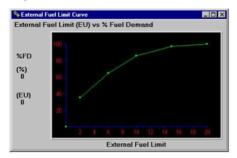
The above screen shows that the External Fuel Limit curve is a 2D curve with five breakpoints. It is set to limit maximum fuel demand at various External Fuel Limit inputs (e.g., Air Manifold Pressure). A digital display of the current x (curve input) and y (curve output) values in engineering units is included. Y in this example is the fuel limit (as a % fuel demand) based on External Fuel Limit X is engineering units.
