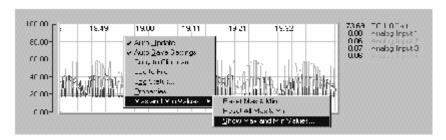
The axis provides another piece of information, the maximum and minimum value of its respective pen. This is indicated by two tick marks on the right side of the axis. When the program is first started, it initializes the values to 0, so it might be necessary to reset the Max and Min values once the program is running. This is accomplished by right clicking on the graph and selecting *Max and Min Values* and then selecting *Reset All Max and Min*.
