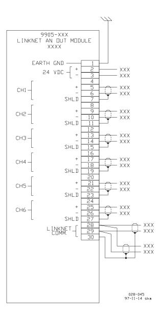
Figure B-14. 4–20 mA Output Module Wiring Diagram
