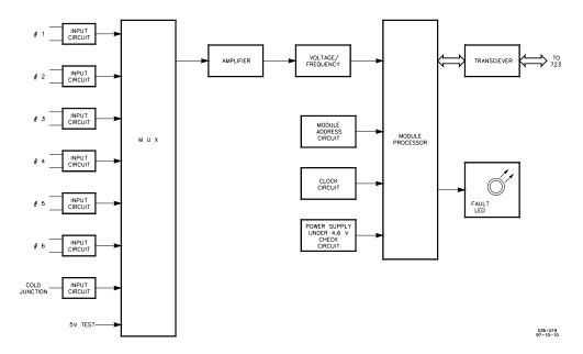
Figure B-7. Thermocouple Input Module Block Diagram
