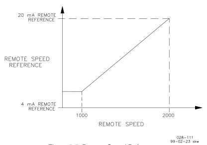
Figure 5-5. Remote Speed Reference
