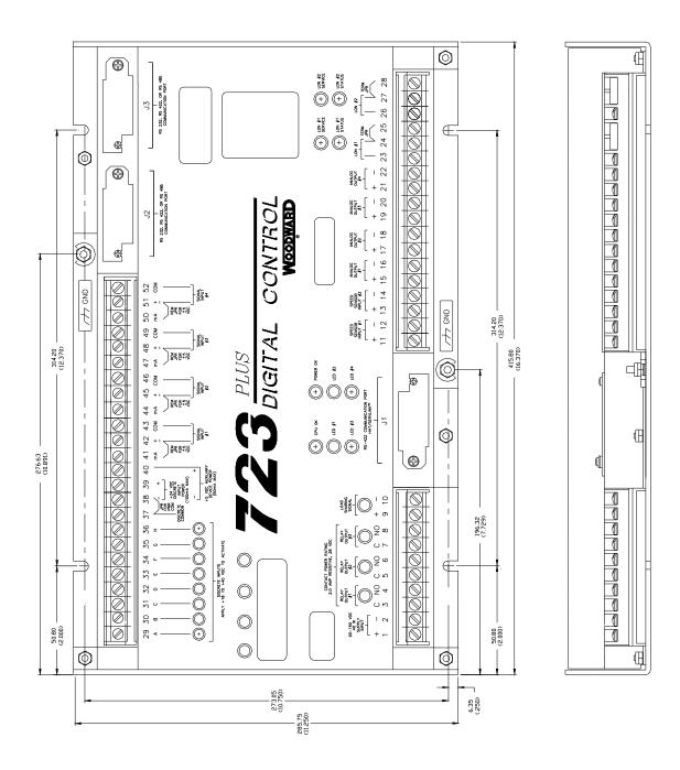
Figure 1-2. 723PLUS Digital Speed Control
