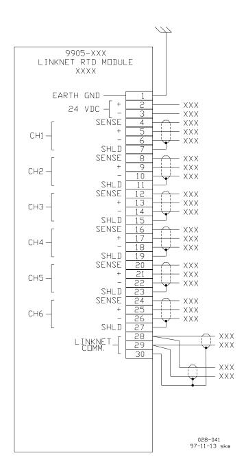
Figure B-10. RTD Input Module Wiring Diagram
