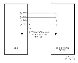
Figure A-1. 723PLUS RS-232 Connections
