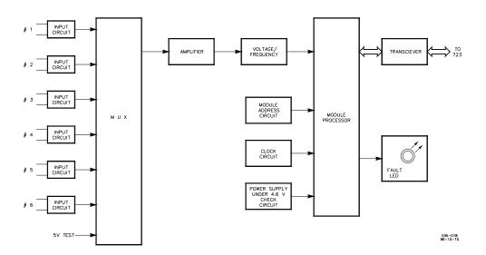
Figure B-5. 4-20 mA Input Module Block Diagram
