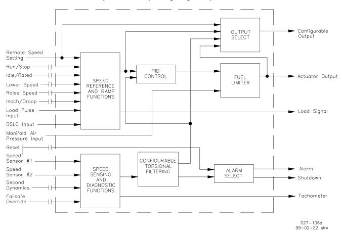
Figure 5-1. Simplified Block Diagram
