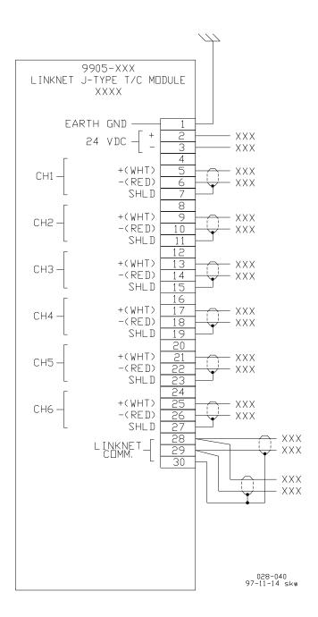
Figure B-8. Thermocouple Input Module Wiring Diagram
