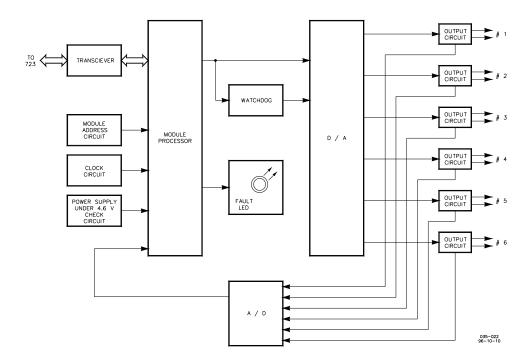
Figure B-13. 4–20 mA Output Module Block Diagram
