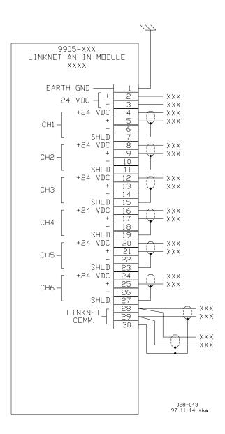
Figure B-6. 4–20 mA Input Module Wiring Diagram
