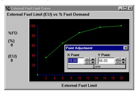
Adjustments to both the x and y breakpoint values can be made, as described earlier, by using the "turtle" and "rabbit" arrows or by typing in values and pressing the = key for the selected point. All breakpoints of all curves can be adjusted in this manner from the curve graph screens.
