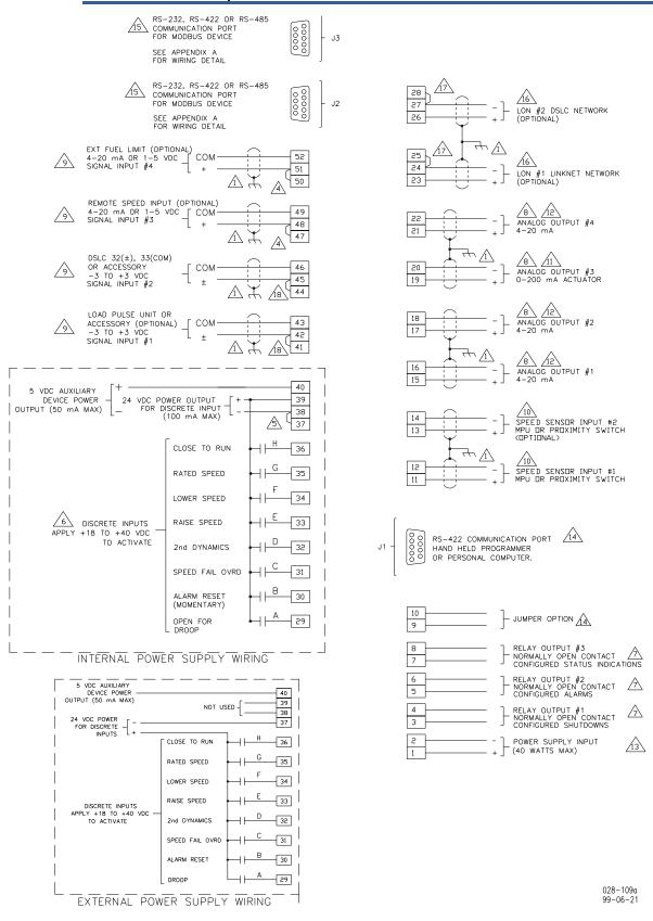
Figure 1-5a. Control Wiring Diagram
