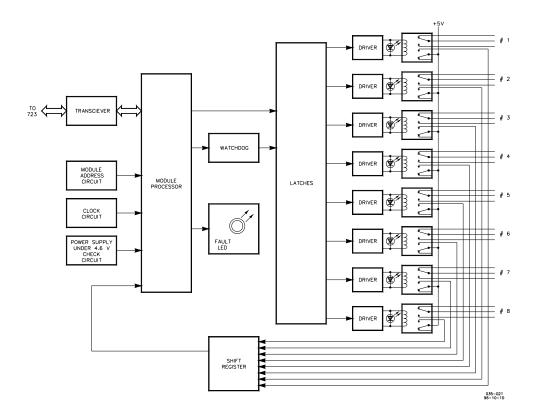
Figure B-11. Relay Output Module Block Diagram
