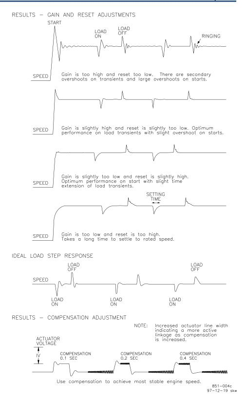
Figure 3-4. Typical Transient Response Curves
