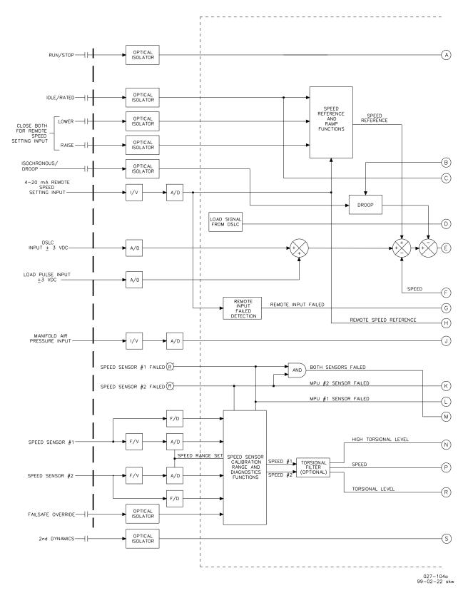
Figure 5-2a. Detailed Block Diagram
