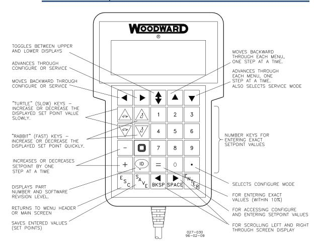
Figure 3-1. Hand Held Programmer Functions
