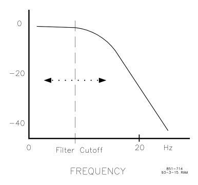
Figure 3-5. Speed Filter
