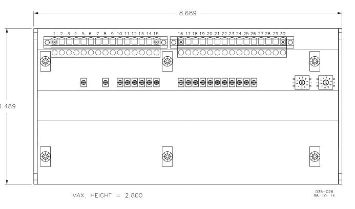
Figure B-2. Outline Drawing of I/O Module
