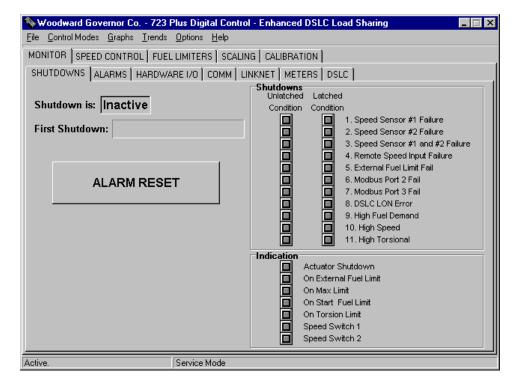
This shows the Monitor Shutdown screen and displays current status of all shutdowns. An Alarm Reset button is provided to reset any control alarms and shutdowns that have been cleared.
