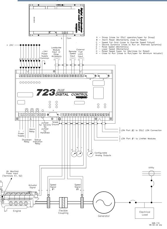
Figure 1-6. Typical 723PLUS Connections
