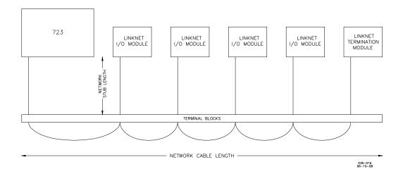
Figure B-17. Network Wired Via Stubs
