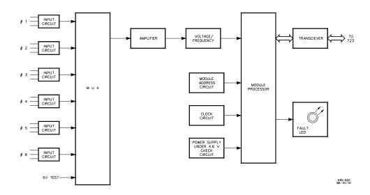
Figure B-9. RTD Input Module Block Diagram
