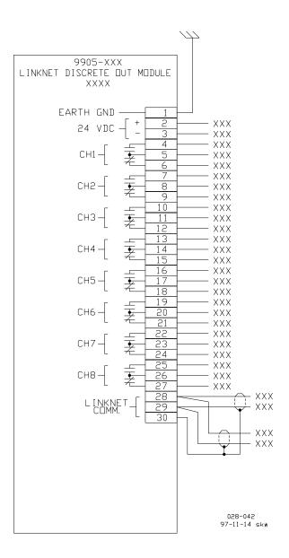
Figure B-12. Relay Output Module Wiring Diagram
