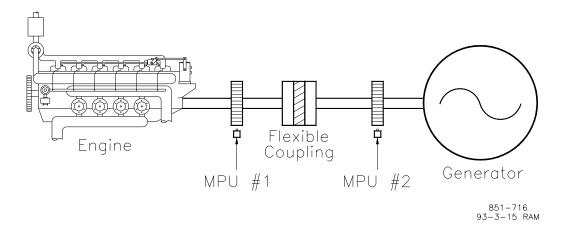
Figure 1-1. Flexible Coupled Generator Set
