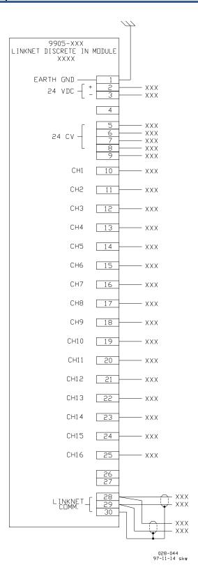
Figure B-4. Discrete Input Module Wiring Diagram
