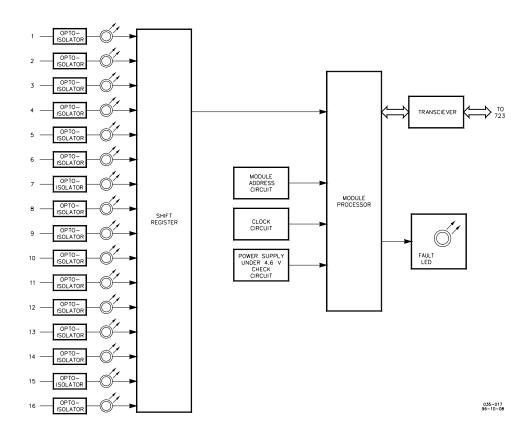
Figure B-3. Discrete Input Module Block Diagram
