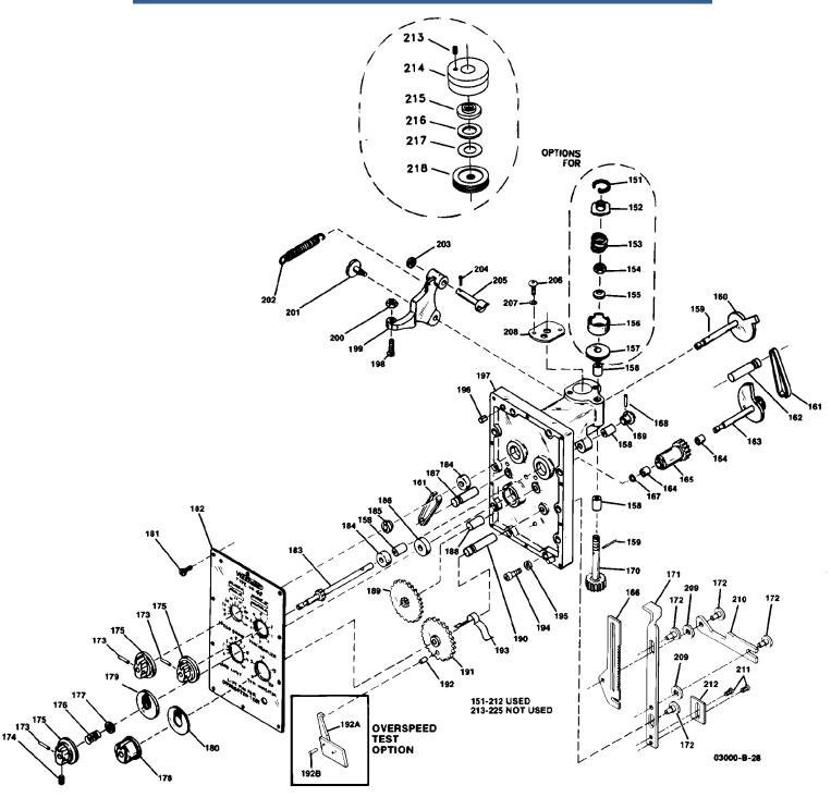
Figure 6-4. UG-40 Front Panel Parts Illustration
