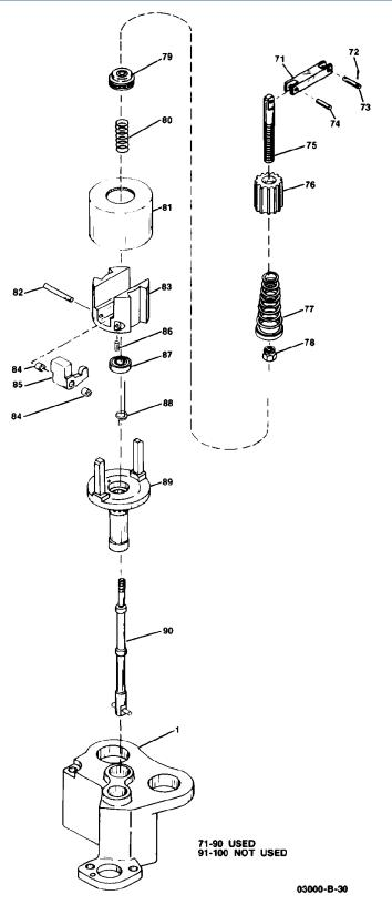
Figure 6-2. UG-40 Ballhead Parts Illustration
