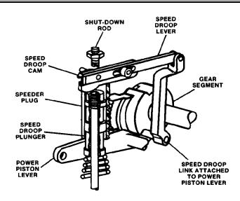
Figure 3-2. Lever Governor Speed Droop Assembly
