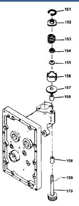
Figure 4-1. Friction Clutch
