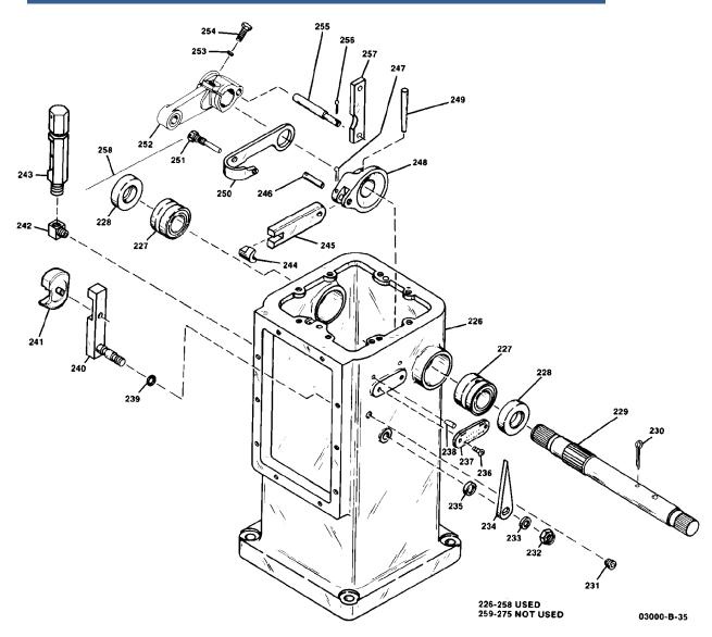
Figure 6-5. UG-40 Case Parts Illustration
