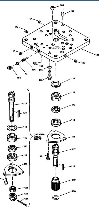
Figure 6-3. UG-40 Base Parts Illustration
