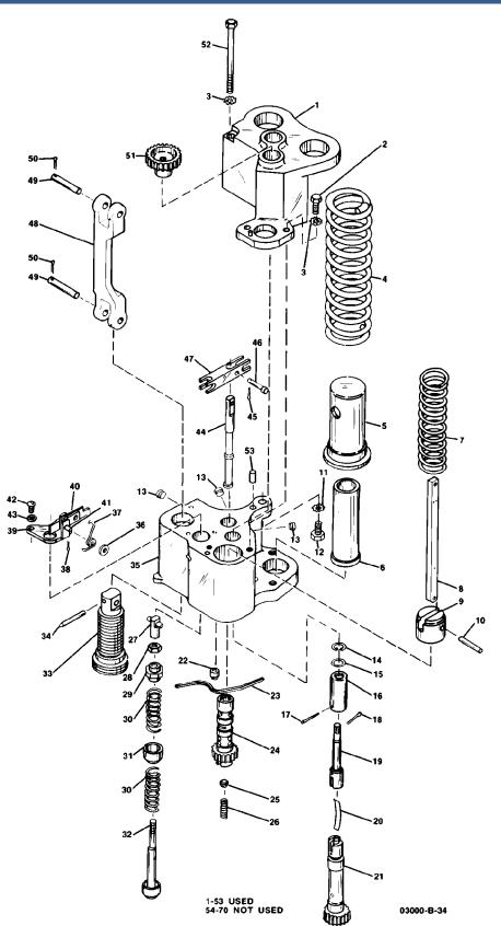
Figure 6-1. UG-40 Controlet Parts Illustration
