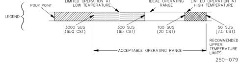
Table 2-1. Viscosity and Operating Temperature of Oils
