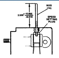
Figure 3. Speed Setting Plug
