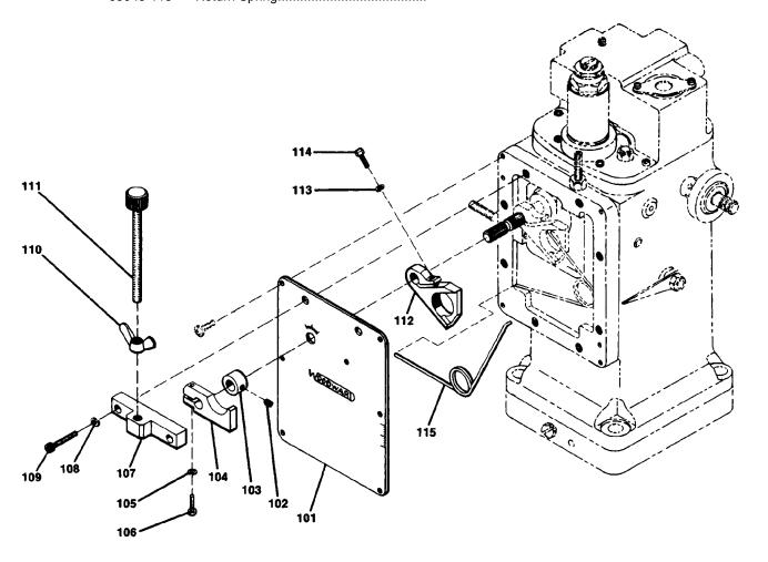
Figure 7. Parts for UG-8 Manual Speed Adjustment
