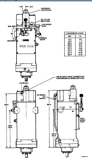
Figure 1. Outline of UG-8 Lever Governor with Pneumatic Speed Adjustment and Manual Speed Setting Screw
