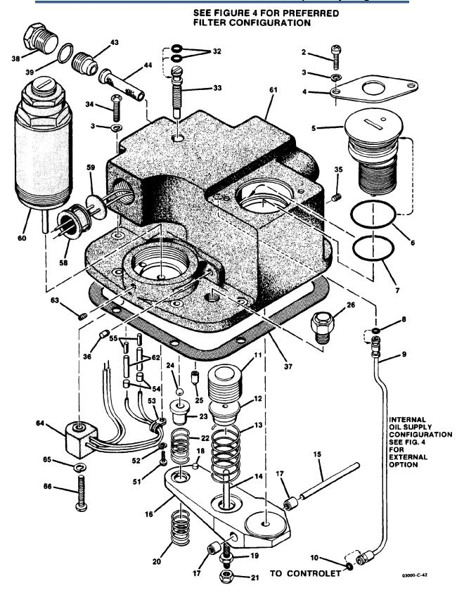
Figure 6. Parts for UG-8 Pneumatic Speed Adjustment with Solenoid Shutdown
