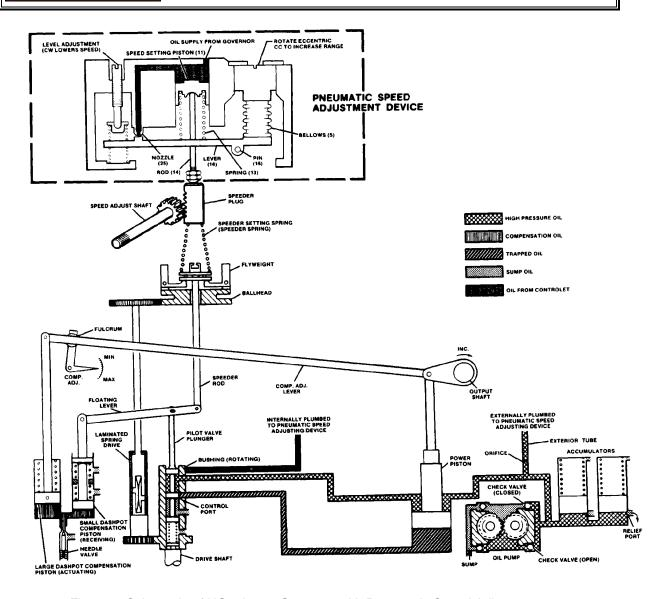
Figure 2. Schematic of UG-8 Lever Governor with Pneumatic Speed Adjustment
