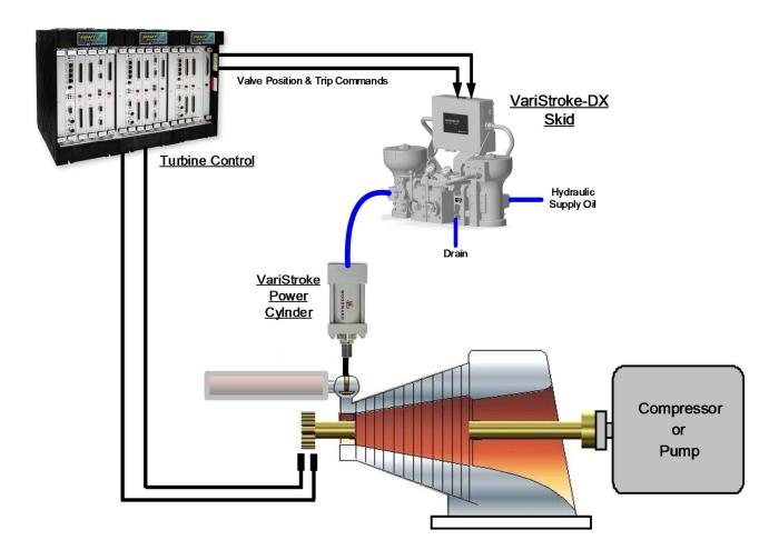
Figure 1. Typical VariStroke-DX Skid Applications
