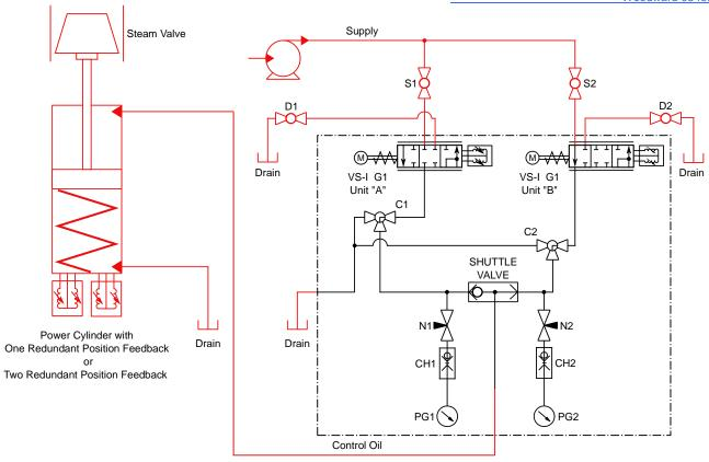
Figure 5. VariStroke-DX Skid Functional Diagram
