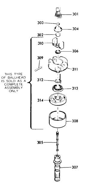
Figure 5-8. Spring driven, Oil-Damped Ballhead Parts
