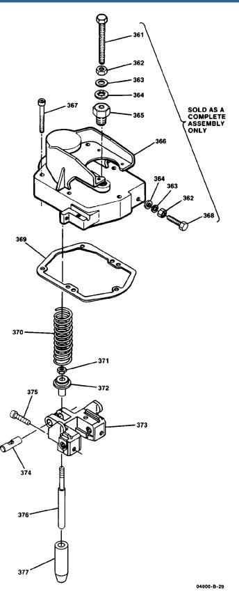
Figure 5-5a. Vertical Return Spring Cover and Installation Parts
