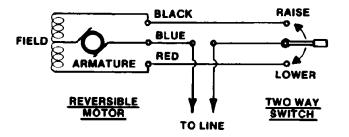
Figure 3-5. Wiring Diagram for Bodine Motor (Switch not furnished)
