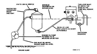
Use a supply system similar to Figure 3-1 for applications requiring quick starts.
