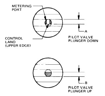
Figure 4-3. Centering Pilot Valve Plunger
