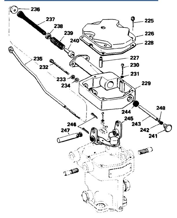
Figure 5-6. Subcap Assembly Parts (linear output)
