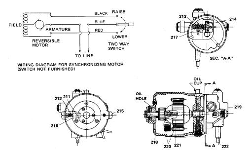
Figure 5-4. Speed Adjusting Motor Parts
