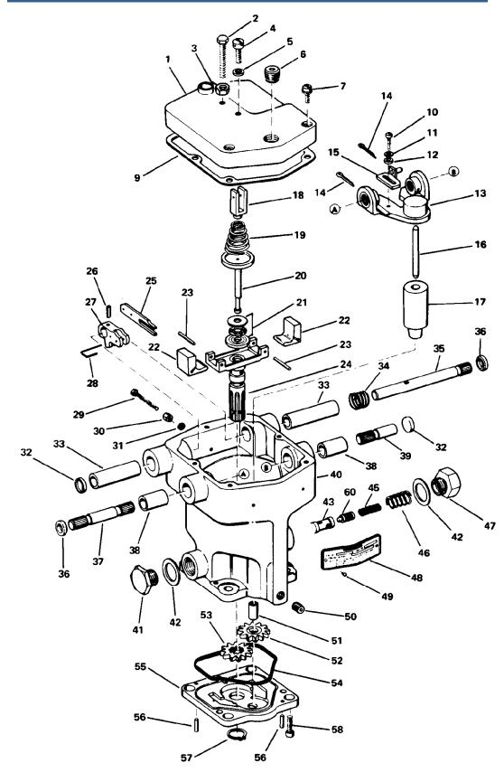
Figure 5-1. Typical SG Governor Parts (later models)
