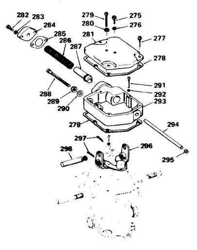
Figure 5-7. Subcap Assembly Parts (internal return spring)
