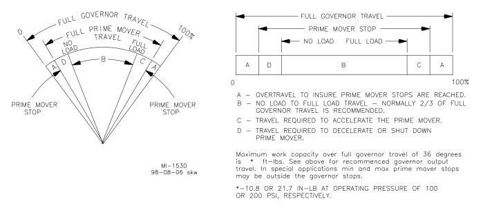
Figure 3-7. Recommended Governor Terminal Shaft Travel
