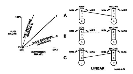
Figure 3-8. Linear Linkage Arrangement
