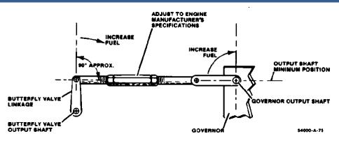
Figure 3-9. Non-linear Linkage Arrangement
