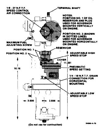
Figure 3-3. SG Governor Outline with Reverse Pneumatic Speed Setting
