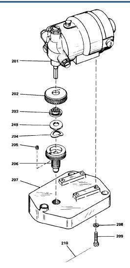
Figure 5-3. Bodine Speed Adjusting Motor and Installation Parts
