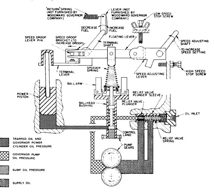
Figure 2-1. Schematic Diagram of a Typical SG Governor
