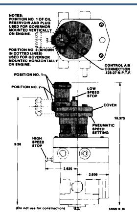
Figure 3-2. SG Governor Outline with Direct Pneumatic Speed Setting
