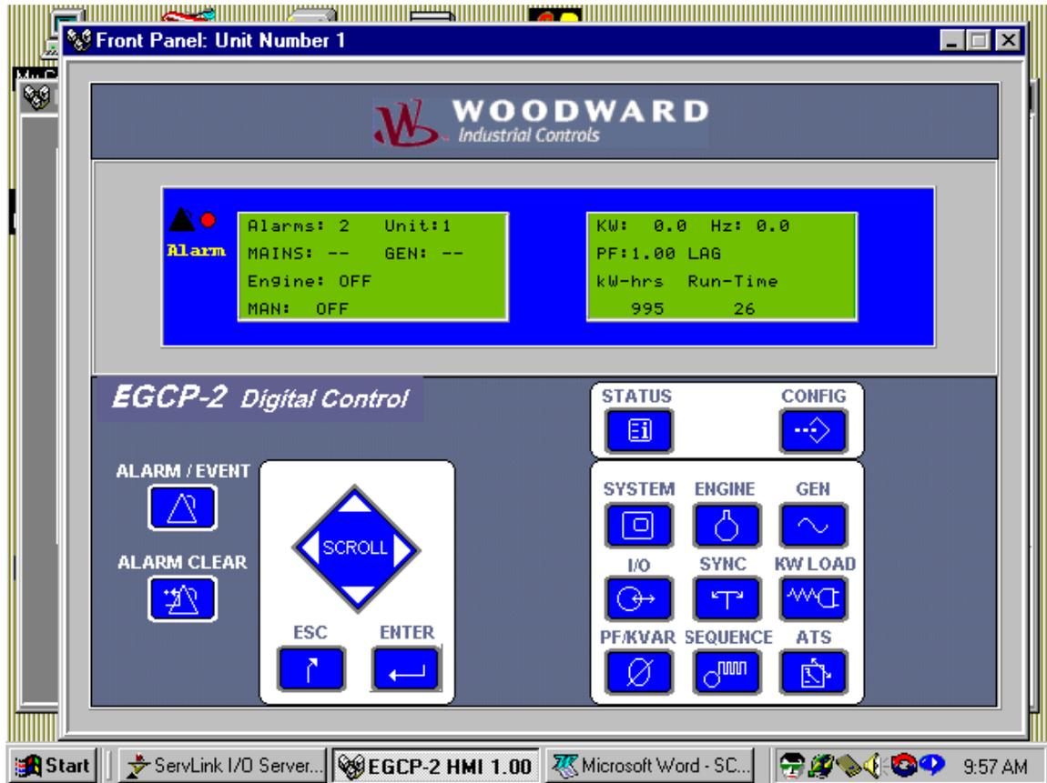
The front panel display for Unit 1 indicates two alarms in the System Status menu. Clicking the Alarm/Event button with the left mouse button will display the Alarm / Event Log of the control to the right hand LCD display as shown below:
