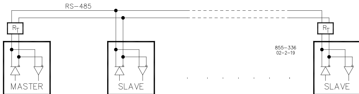
Figure 6-13. RS-485 Terminator Locations
