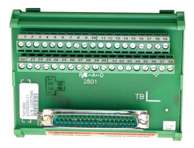
Figure 12-34. Position Controller FTM
