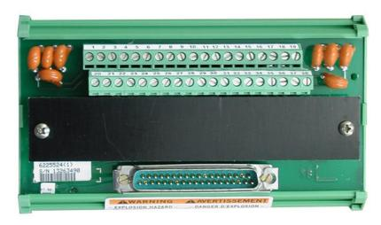
Figure 12-28. Non-Standard Analog Input FTM
