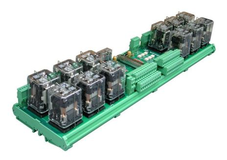
Figure 12-37. 24/12 Discrete Module
