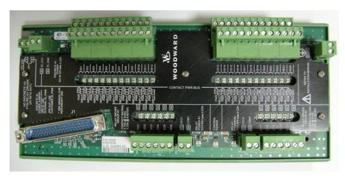
Figure 12-49. 24/12 Discrete I/O (with LEDs) FTM
