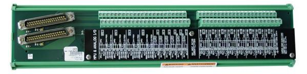
Figure 12-25. Analog Combo FTM
