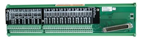
Figure 12-1. 34Ch HDVIM FTM (AI/RTD/TC)
