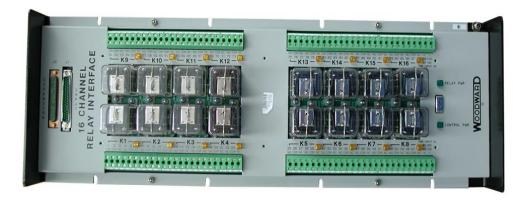
Figure 12-57. 16 Channel Relay Module
