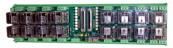
Figure 12-53. 16 Channel Relay Module (Phoenix Contact)
