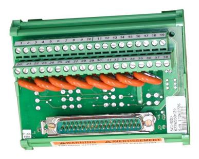
Figure 12-19. Analog Input FTM
