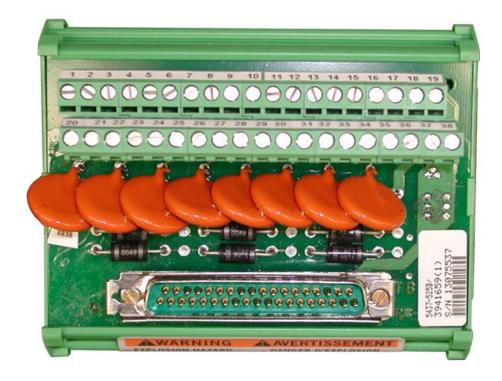
Figure 12-13. Four Channel Actuator Driver FTM
