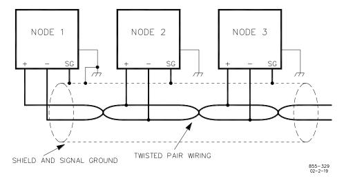
Figure 3.23. Alternate Multipoint Wiring Using Shielded Twisted-Pair Cable without a Separate Signal Ground Wire
