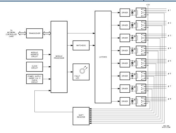
Figure 10-24. Relay Output Module Block Diagram
