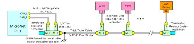
Figure 2-7. MicroNet to Valve CAN Interface
