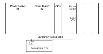
Figure 7-39. 8Ch Current Output (4-20 mA) Module Configuration
