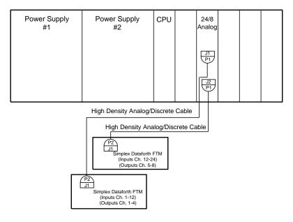
Figure 7-6. Simplex Dataforth Configuration Example
