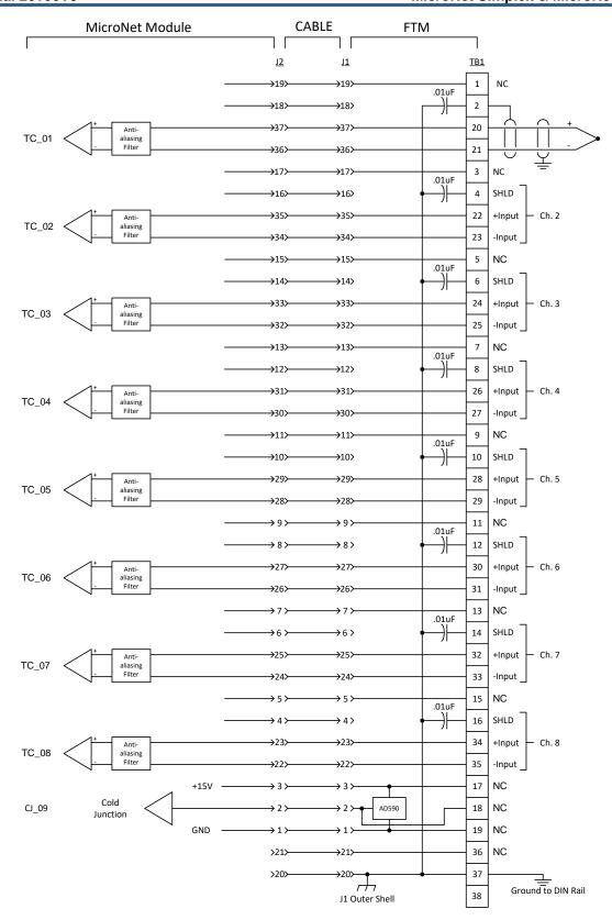
Figure 7-50. 8Ch TC Input (Fail Low) Module Field Wiring
