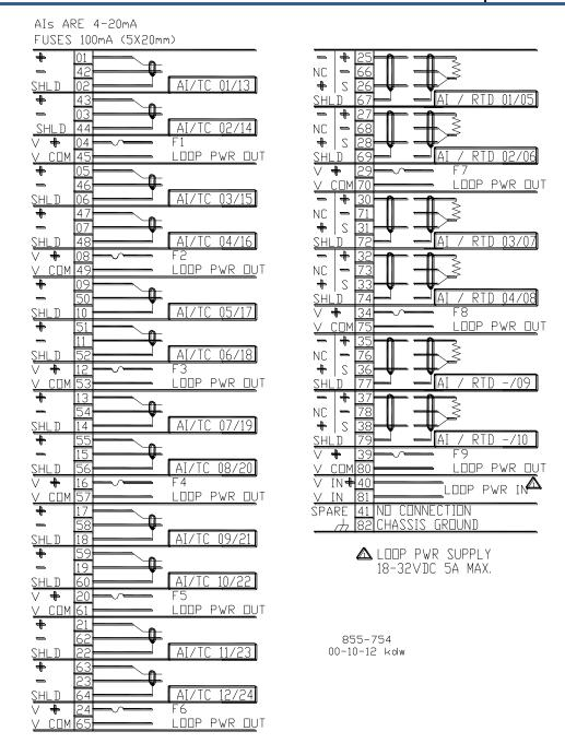
Figure 7-22. Wiring Diagram for 34Ch HDVIM FTM
