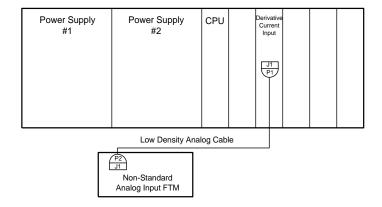
Figure 7-32. Non-Standard 8Ch Current Input (4-20 mA) Module Configuration
