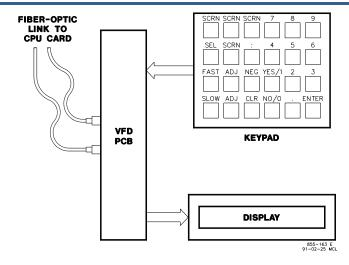
Figure 9-2. Service Panel Block Diagram
