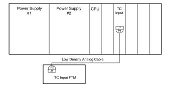
Figure 7-49. 8Ch TC (Fail Low) Module Configuration
