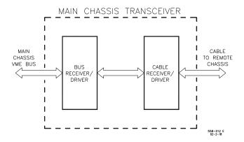
Figure 3-1. Main XCVR Module Block Diagram
