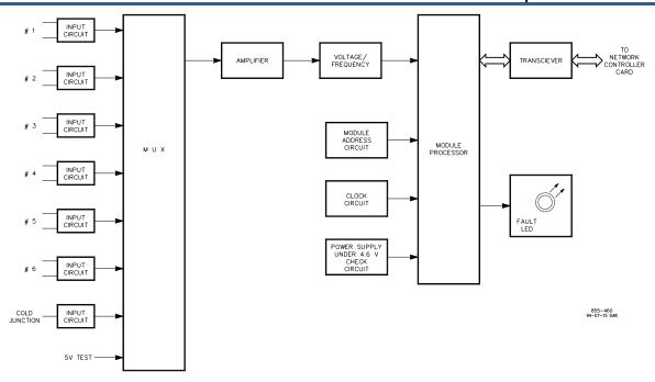
Figure 10-11. Thermocouple Input Module Block Diagram
