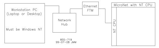
Figure 2-13. Network Block Diagram
