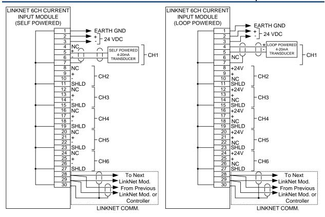
Figure 10-13. LINKnet 6CH Current Input Module Wiring
