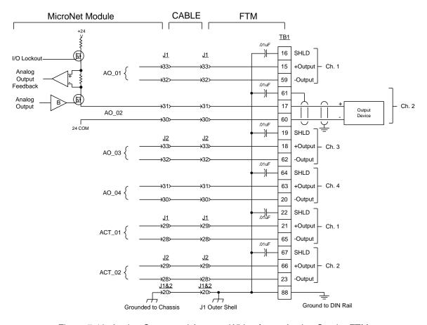
Figure 7-19. Analog Output and Actuator Wiring for an Analog Combo FTM
