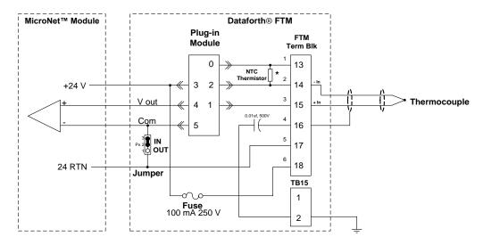
Figure 7-7. Thermocouple Wiring to Simplex Dataforth FTM
