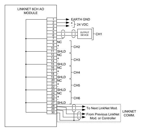
Figure 10-19. LINKnet 6 Channel AO Module Wiring
