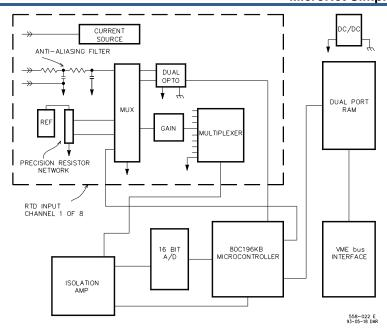
Figure 7-56. RTD Input Block Diagram
