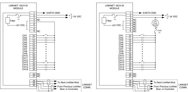
Figure 10-16. LINKnet 16CH DI Module Wiring
