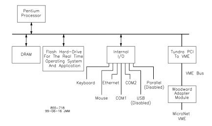
Figure 2-9. Windows NT CPU Block Diagram
