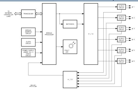
Figure 10-20. 4-20 mA Output Module Block Diagram
