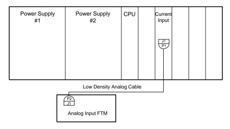
Figure 7-28. 8Ch Current Input (4-20 mA) Module Configuration
