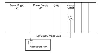
Figure 7-44. 8Ch Voltage Output (0-5 Vdc) Module Configuration
