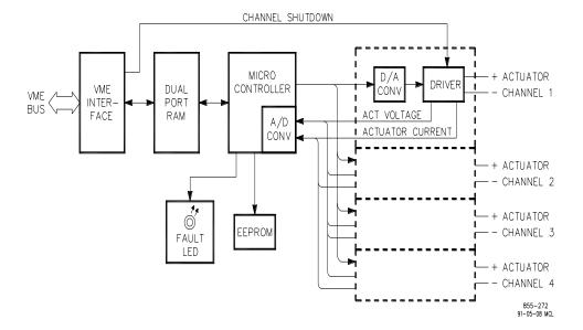
Figure 8-2. Four Channel Actuator Driver Module Block Diagram
