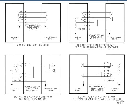
Figure 3.21. Termination and Cable Connection Examples
