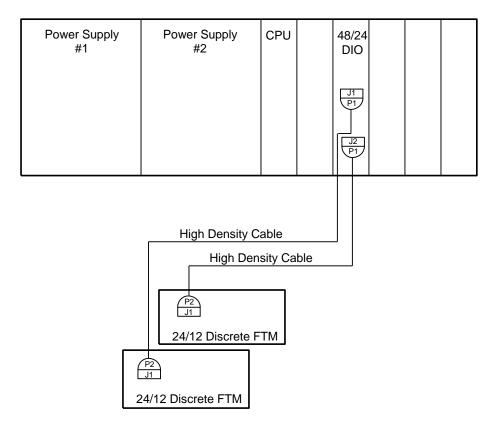
Figure 6-7. Configuration 2, Two 24/12 Discrete FTMs
