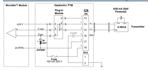
Figure 7-10. Self-powered 4-20 mA Signal Wiring to Simplex Dataforth FTM
