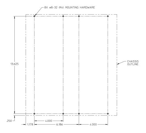
Figure 4-3. Mounting Template of MicroNet 6-Slot I/O Chassis
