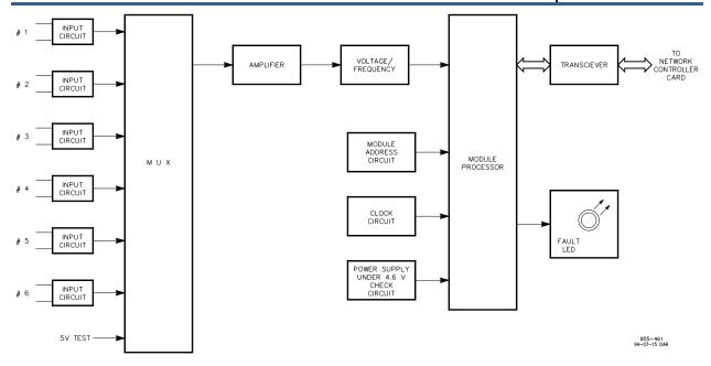
Figure 10-14. 4-20 mA Input Module Block Diagram
