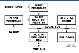
Figure 7-63. Digital Speed Sensor Module Block Diagram
