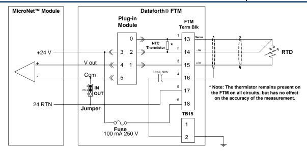
Figure 7-8. RTD Wiring to Simplex Dataforth FTM
