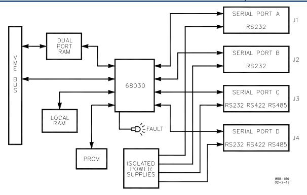
Figure 3-17. SIO Module Block Diagram
