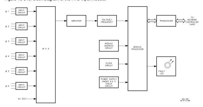
Figure 10-8. RTD Input Module Block Diagram
