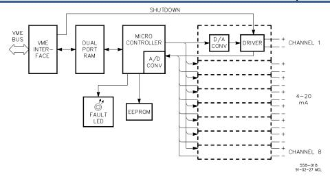
Figure 7-41. Current Output (4-20 mA) Module Block Diagram
