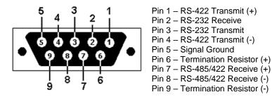
Figure 2-4. CPU Communications Port (DB9F)
