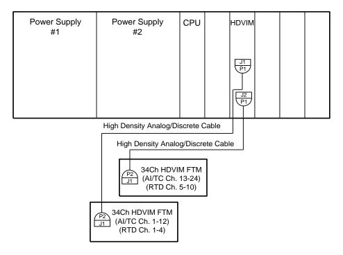
Figure 7-21. Simplex System Configuration Example
