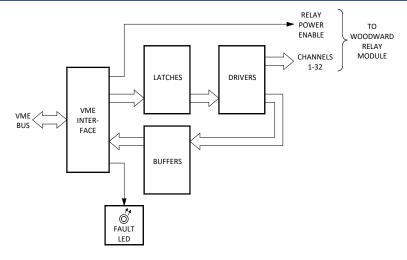
Figure 6-15. Discrete Output Module (32 Channel) Block Diagram
