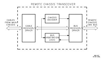
Figure 3-3. Remote XCVR Module Block Diagram
