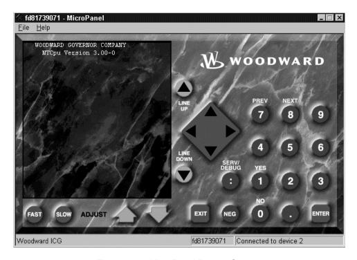
Figure 2-10. MicroPanel Display Screen
