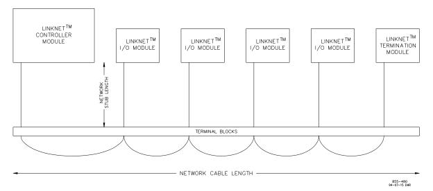
Figure 10-3. Network Wired Via Stubs
