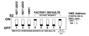
Figure 3-11. VME Address Configuration
