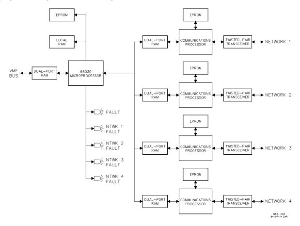
Figure 10-5. 4Ch LINKnet Module Block Diagram
