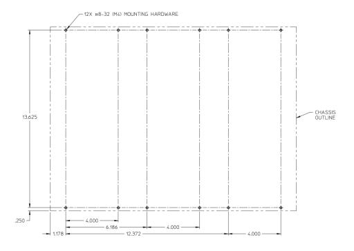
Figure 4-6. Mounting Template of MicroNet 12-Slot I/O Chassis
