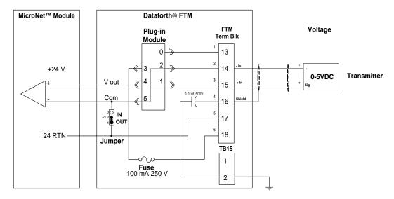
Figure 7-11. 0-5 Vdc Signal Wiring to Simplex Dataforth FTM
