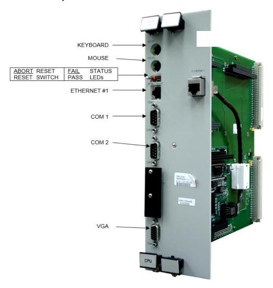
Figure 2-14. NT CPU (Pentium with Dual Ethernet) Module
