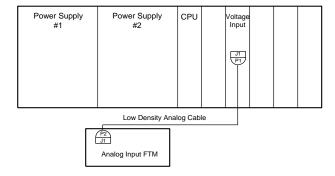
Figure 7-35. 8Ch Voltage Input (0-10 Vdc) Module Configuration
