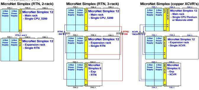
Figure 3-12. MicroNet Simplex System Diagrams
