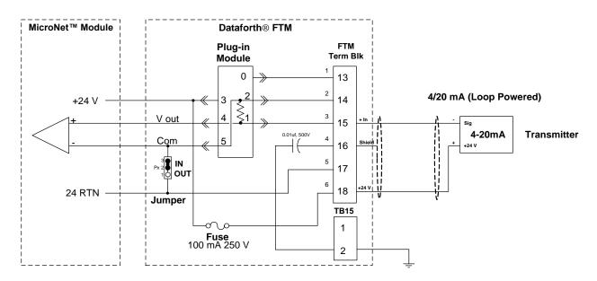
Figure 7-9. Loop powered 4-20 mA Signal Wiring to Simplex Dataforth FTM
