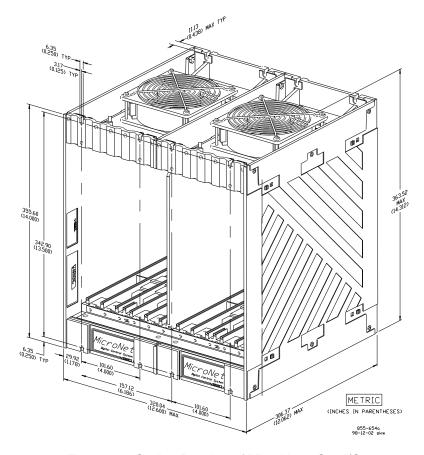
Figure 4-2. Outline Drawing of MicroNet 6-Slot I/O
