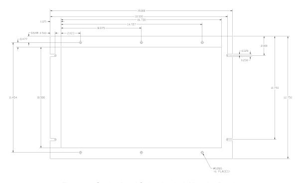
Figure 9-5. Service Panel Optional 19 Inch Mounting Panel
