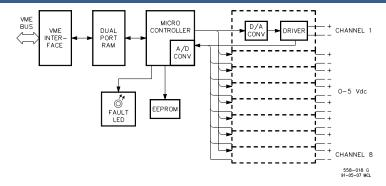
Figure 7-46. 8Ch Voltage Output (0-5 Vdc) Module Block Diagram
