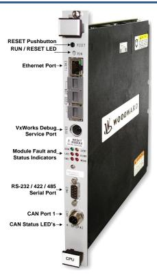
Figure 2-1. CPU5200L Module
