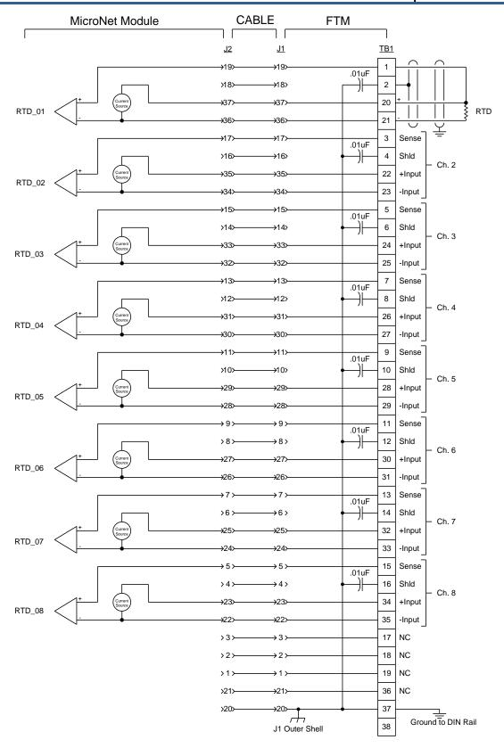
Figure 7-55. 8Ch RTD Input Module Field Wiring
