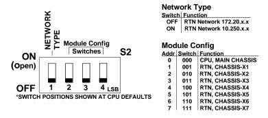
Figure 2-3. CPU5200L Module Hardware Configuration
