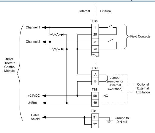
Figure 6-8. Discrete Input Interface Wiring to a 24/12 Discrete FTM
