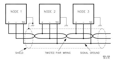
Figure 3-22. Preferred Multipoint Wiring Using Shielded Twisted-Pair Cable with a Separate Signal Ground Wire
