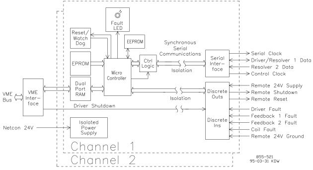
Figure 8-5. Position Controller Module Block Diagram
