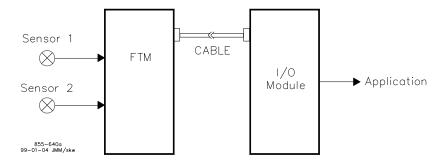
Figure 3-15. Redundant Sensors
