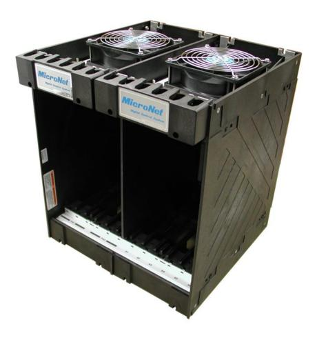
Figure 4-1. Simplex MicroNet 6-Slot I/O
