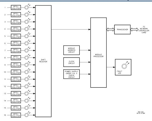
Figure 10-17. Discrete Input Module Block Diagram
