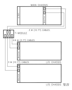
Figure 3-8. Expansion I/O Chassis
