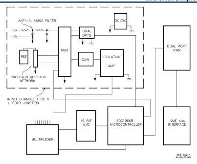
Figure 7-51. Thermocouple Input Block Diagram
