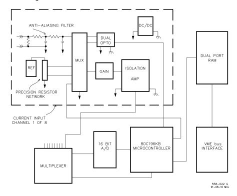
Figure 7-30. 8Ch Current Input (0-25 mA) Module Block Diagram
