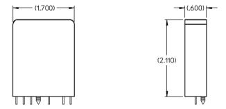
Figure 7-13. Dataforth Plug-in Modules
