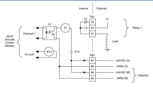
Figure 6-9. Relay Output Interface Wiring to a 24/12 Discrete FTM
