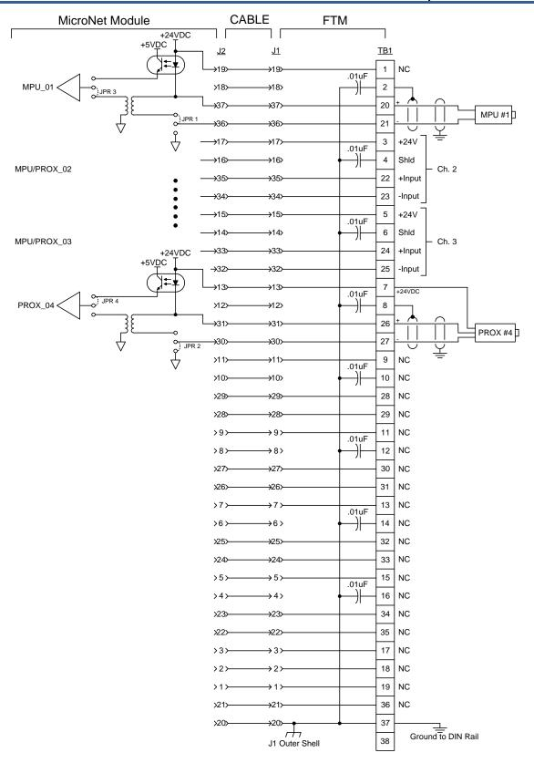
Figure 7-62. MPU and Proximity Probe Interface Wiring
