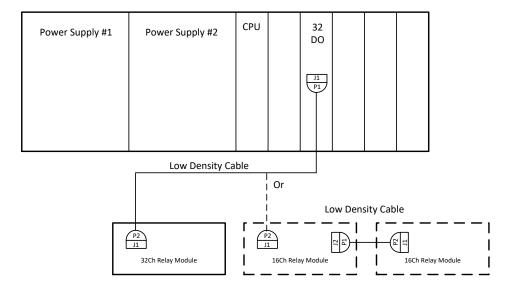
Figure 6-12. 32Ch DO Module with Relay Modules
