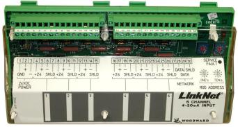
Figure 10-12. Both LINKnet 6Ch Current Input Modules
