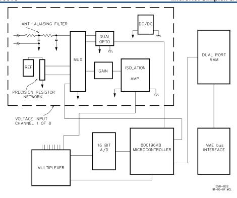
Figure 7-37. 8Ch Voltage Input (0-10 Vdc) Module Block Diagram
