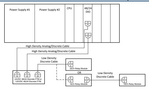
Figure 6-2. Configuration 1, One 48/24 Discrete FTM with Relay Module(s)
