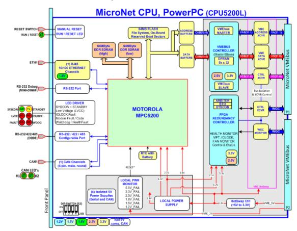
Figure 2-2. CPU5200L Module Block Diagram
