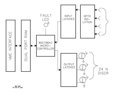
Figure 6-10. 48/24 Discrete Combo Module Block Diagram
