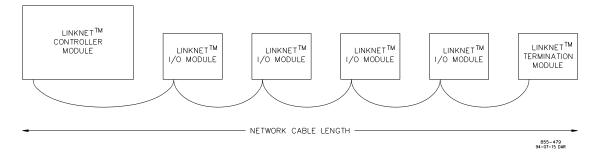
Figure 10-2. Direct Wired Network
