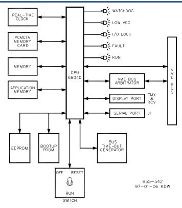
Figure 2-22. CPU Module Block Diagram
