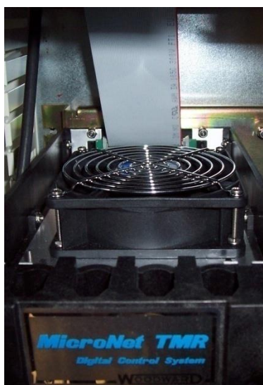
Figure 4-3. TMR PS Chassis PS Ribbon Cable (5416-977) Connections
