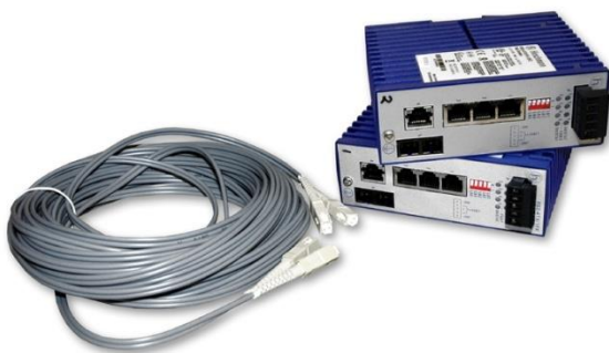
Figure 6-7. MicroNet RTN Module Fiber Optic Cable Specification
