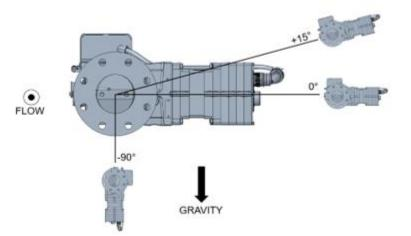
Figure 2-1b. Allowable Actuator Orientations
