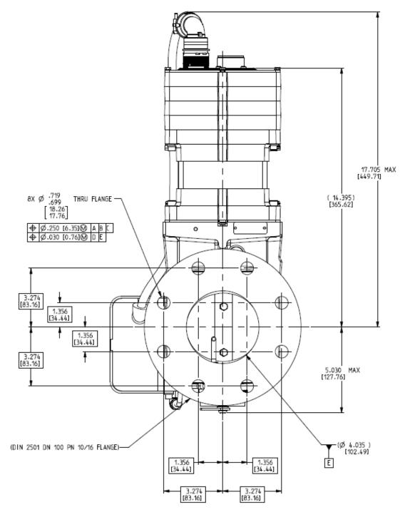
Figure 2-2d. Valve Inlet View
