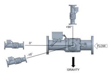
Figure 2-1c. Allowable Bore Orientations
