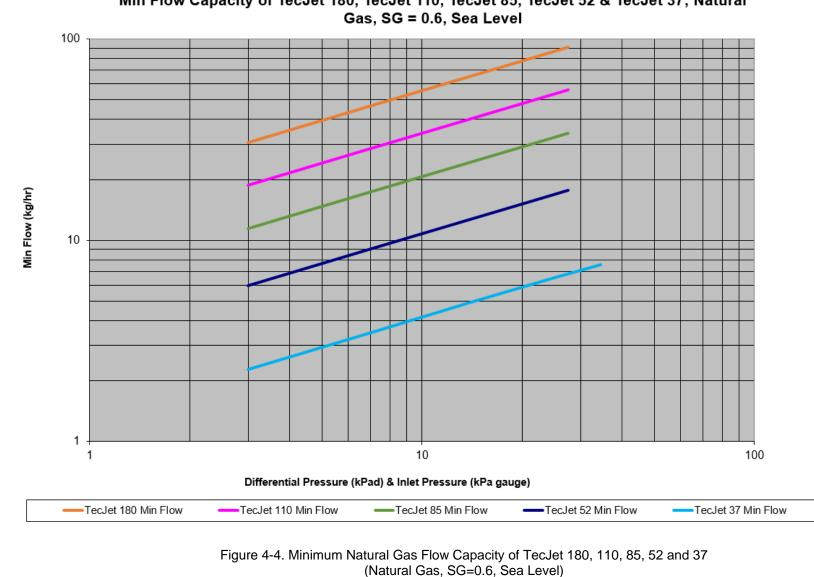
Min Flow Capacity of TecJet 180, TecJet 110, TecJet 85, TecJet 52 & TecJet 37; Natural
