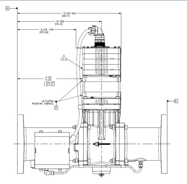
Figure 2-2c. Valve Outlet to Actuator Mounting View
