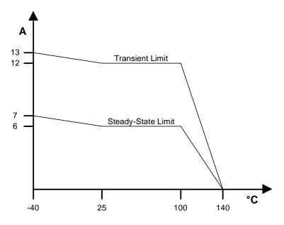
Figure 3-1. Current Limiting Based on Temperature
