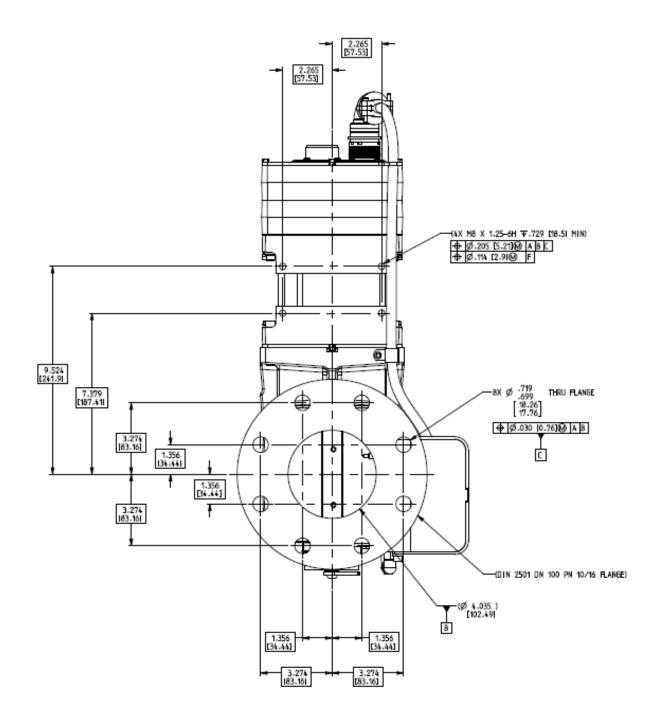
Figure 2-2b. Valve Outlet Flange and Actuator Mounting View
