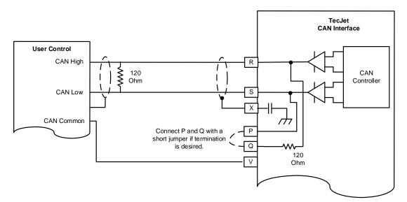
Figure 2-5. TecJet 110 CAN Wiring for Non-isolated Systems
