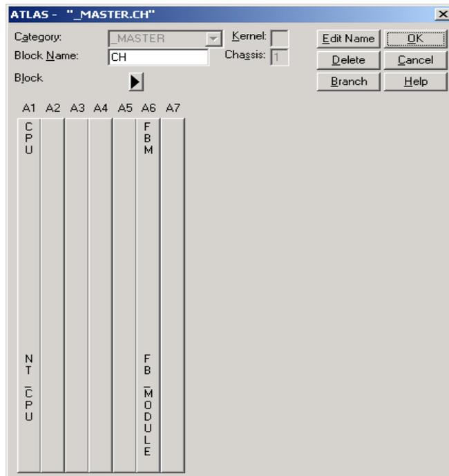
2. Select a FB\_EQUIP Block for every node in the Network and assign the FB\_MODULE as its Parent Block. Every FB\_EQUIP block must have its EQUIP\_NO set to the MACID of its respective node.
