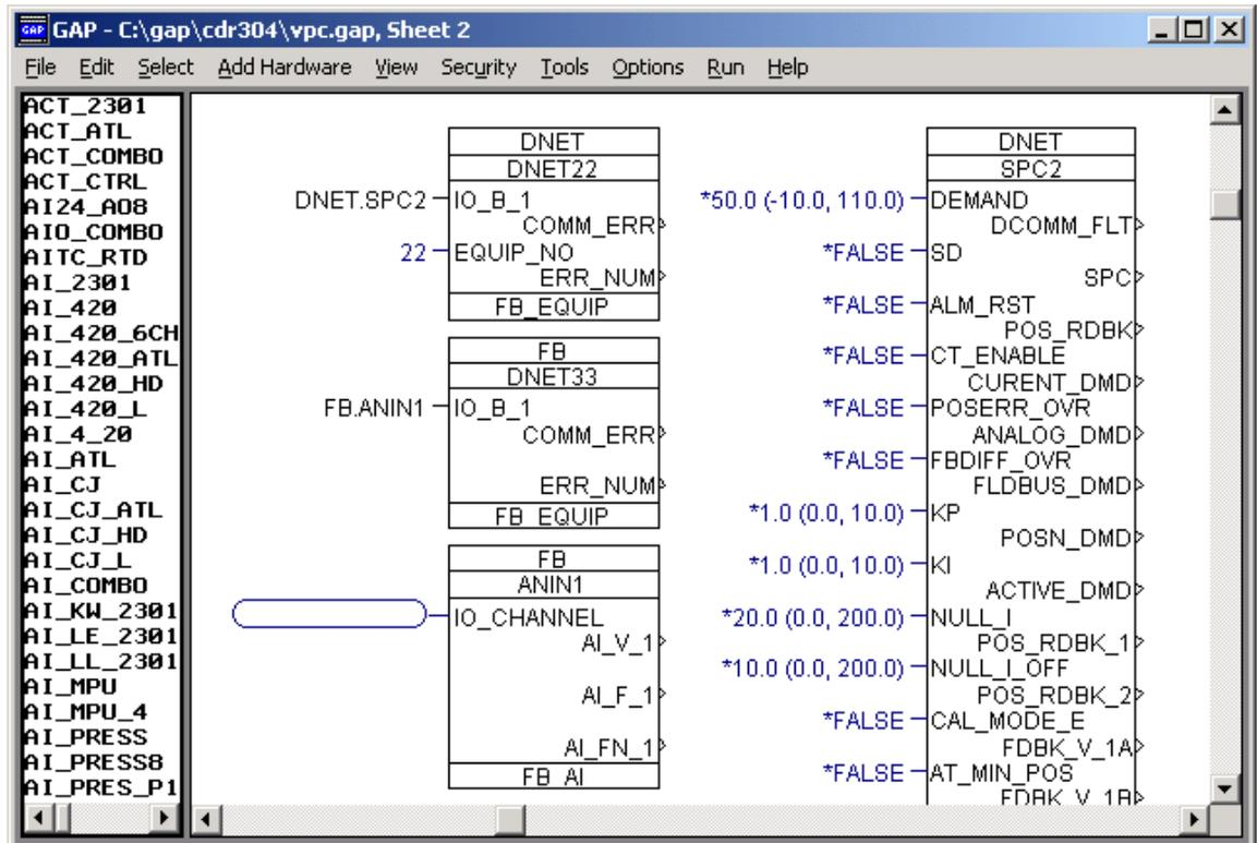
4. The coded GAP application must be compiled, filename.OUT, downloaded to the AtlasPC control using AppManager.
