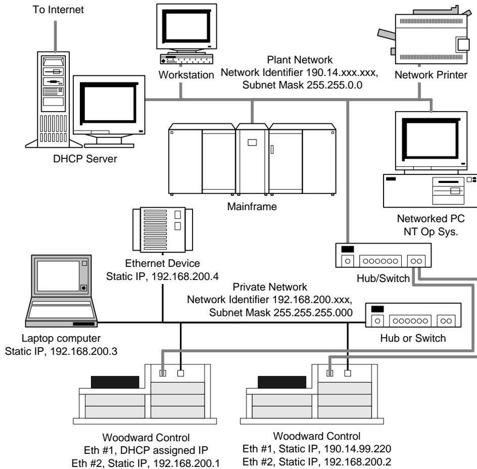
Figure 2-1. Setup Example for Controls with Dual Ethernet
