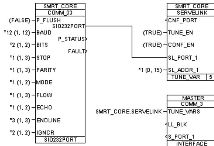
Reference This SIO232PORT block in a parent, hardware block, like the SMARTCOR\_S.
