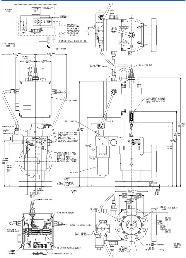
Figure 1-4a. Outline Drawing (3" Control Valve with Single-Entry Box)
