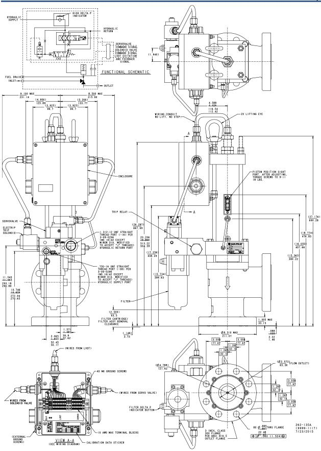
Figure 1-5a. Outline Drawing (3" Control Valve with Dual-Entry Box)
