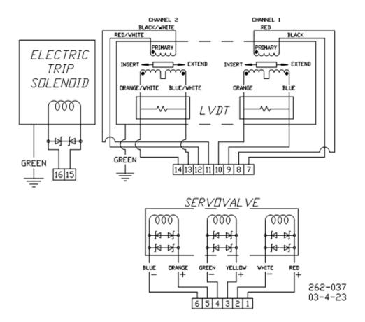
Figure 1-11a. Wiring Diagram – Single-Entry Conduit Box
