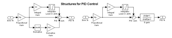
Figure 3-5. Structures for PID Control
