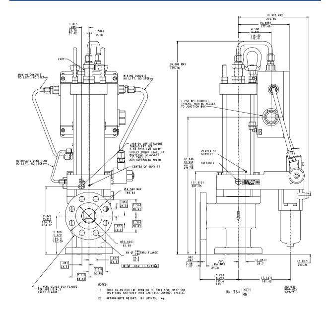
Figure 1-2b. Outline Drawing (2" Control Valve with Single-Entry Box)
