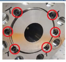
Figure 3-1. Illustration of Diverging Sleeve Screws
