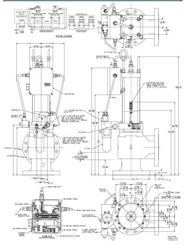
Figure 1-8a. Outline Drawing (6" Control Valve with Single-Entry Box)
