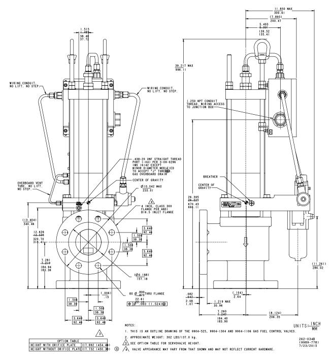
Figure 1-6b. Outline Drawing (4" Control Valve with Single-Entry Box)
