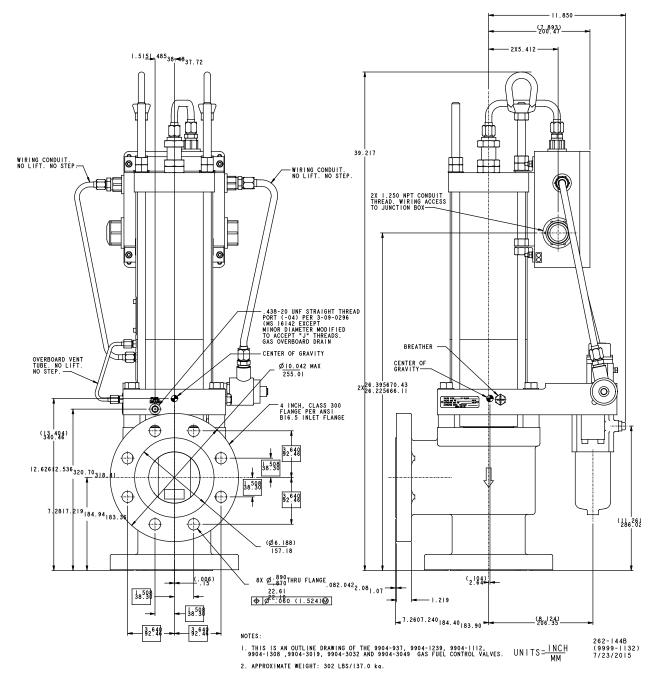
Figure 1-7b. Outline Drawing (4" Control Valve with Dual-Entry Box)
