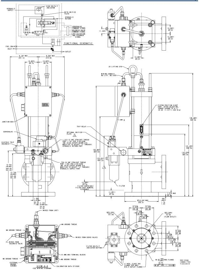
Figure 1-6a. Outline Drawing (4" Control Valve with Single-Entry Box)
