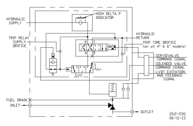
Figure 1-10. Hydraulic Schematic Circuit
