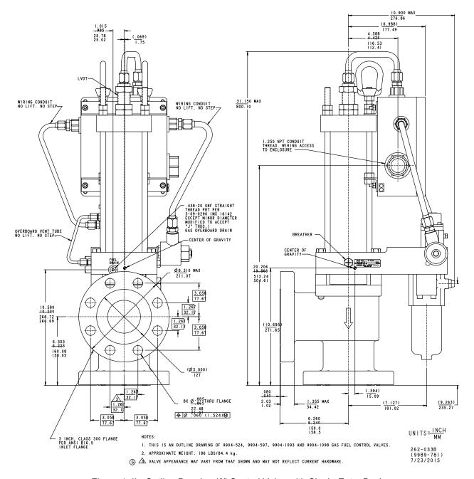
Figure 1-4b. Outline Drawing (3" Control Valve with Single-Entry Box)
