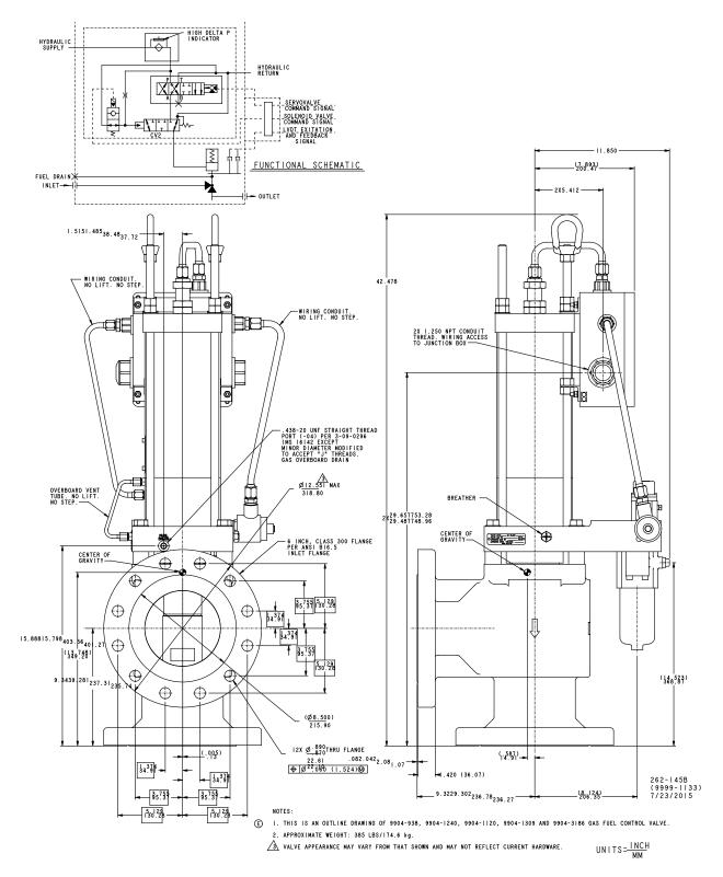
Figure 1-9b. Outline Drawing (6" Control Valve with Dual-Entry Box)
