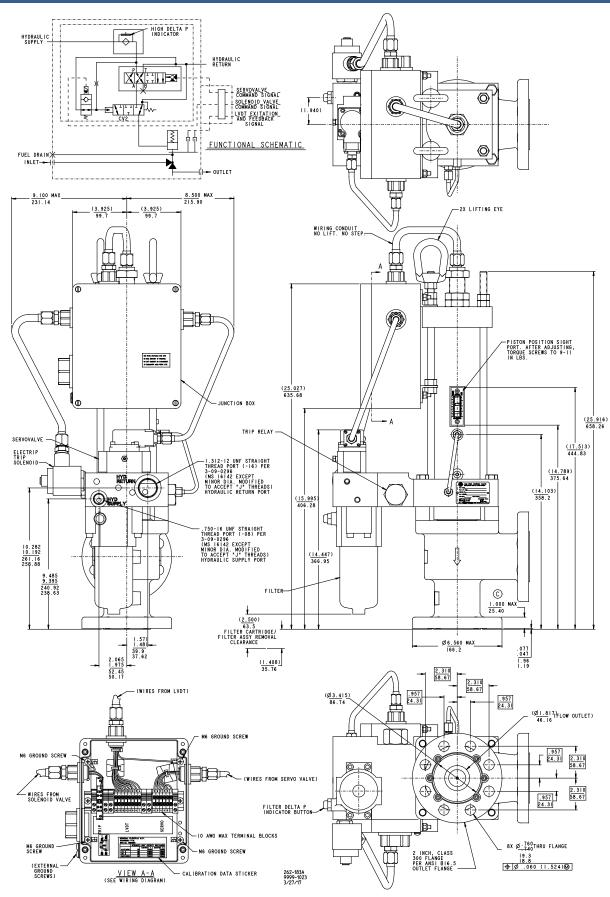
Figure 1-2a. Outline Drawing (2" Control Valve with Single-Entry Box)
