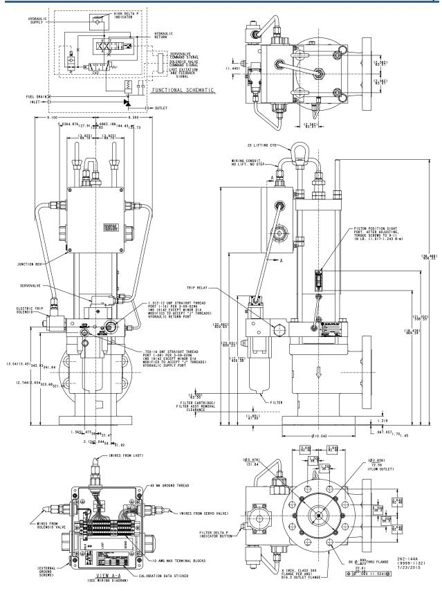
Figure 1-7a. Outline Drawing (4" Control Valve with Dual-Entry Box)
