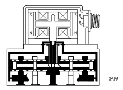
Figure 2-1. Servo Valve Cutaway
