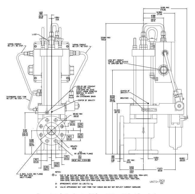
Figure 1-3b. Outline Drawing (2" Control Valve with Dual-Entry Box)
