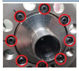
DIVERGING SLEEVE SCREWS -DO NOT PRESSURE LOAD!
