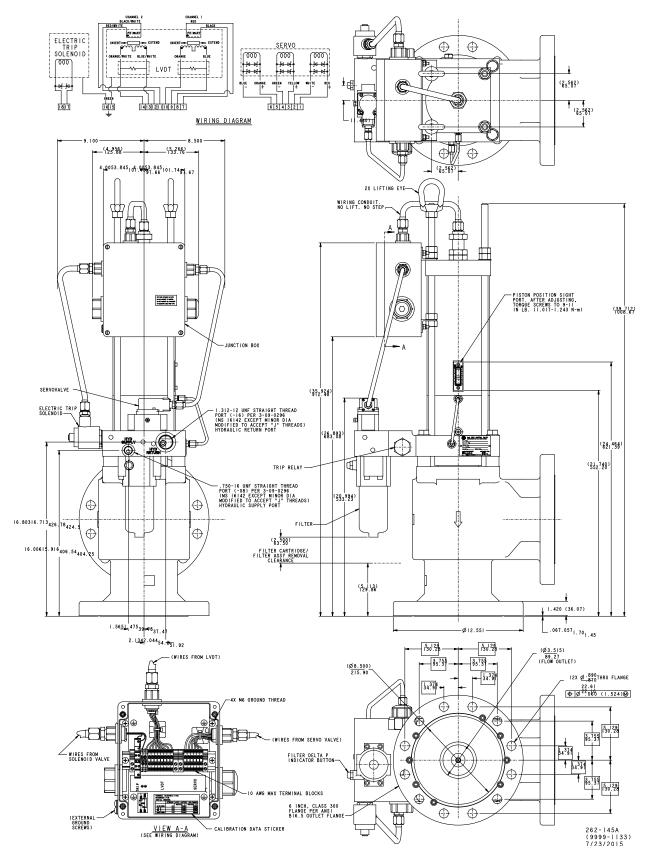
Figure 1-9a. Outline Drawing (6" Control Valve with Dual-Entry Box)
