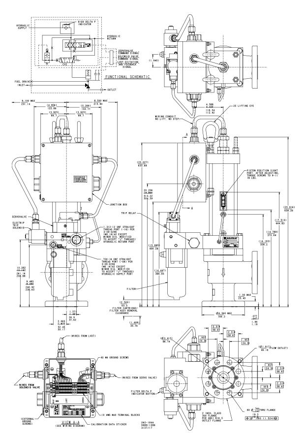
Figure 1-3a. Outline Drawing (2" Control Valve with Dual-Entry Box)
