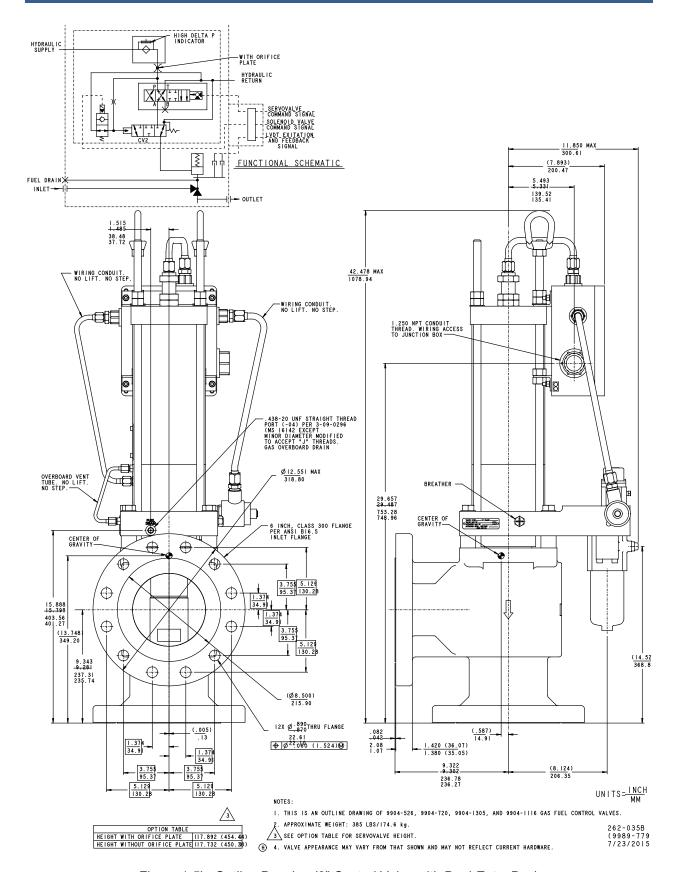
Figure 1-5b. Outline Drawing (3" Control Valve with Dual-Entry Box)
