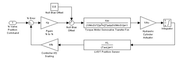
Figure 3-4. Gas Fuel Control Valve Block Diagram
