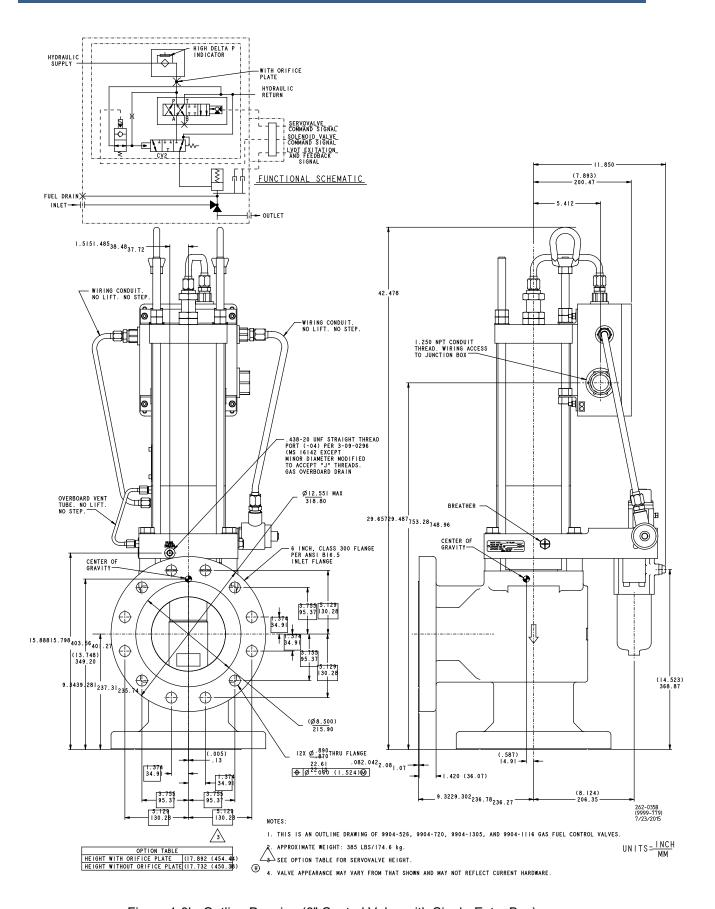
Figure 1-8b. Outline Drawing (6" Control Valve with Single-Entry Box)
