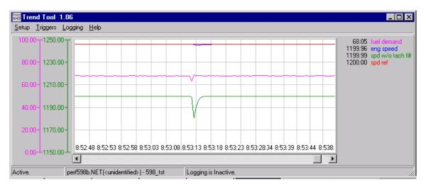
15. **Bump** the actuator (it is okay to use a larger bump this time) to test control response. The above trace shows the expected response.
