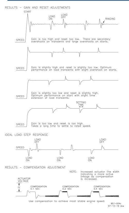
Figure 3-4. Typical Transient Response Curves
