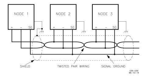
Figure A-4. Preferred Multipoint Wiring Using Shielded Twisted-pair Cable with a Separate Signal Ground Wire
