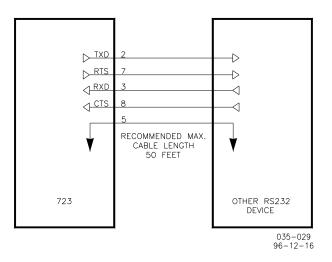
Figure A-1. 723PLUS RS-232 Connections
