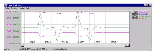
This trace shows the transient response with the Gain Ratio and Window Width disabled. In this example Gain is 1.235; Reset is 0.28, and Compensation is 0.88. Load step is ~15%.
