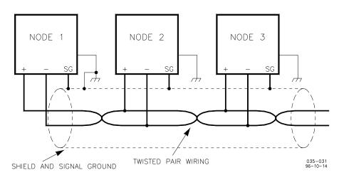
Figure A-5. Alternate Multipoint Wiring Using Shielded Twisted-pair Cable without a Separate Signal Ground Wire
