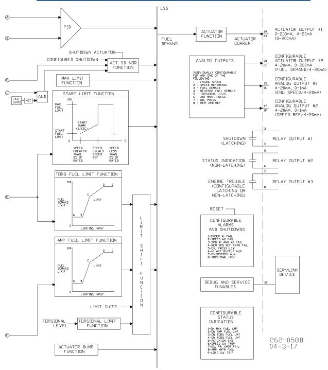
Figure 1-6. 723PLUS Block Diagram
