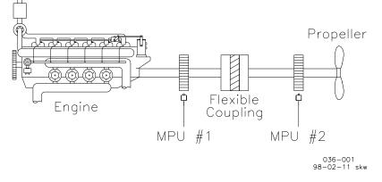
Figure 1-1. Flexible Coupled Propeller
