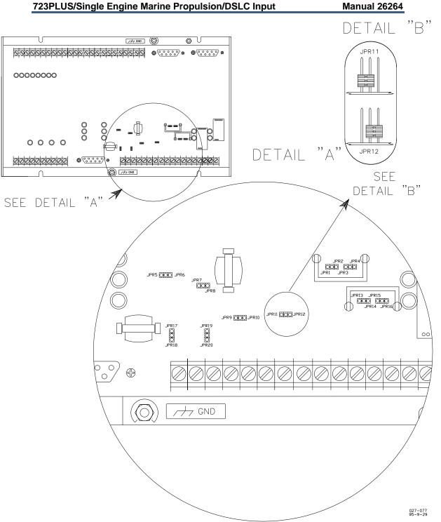
Figure 2-1. 723PLUS Control Internal Jumpers
