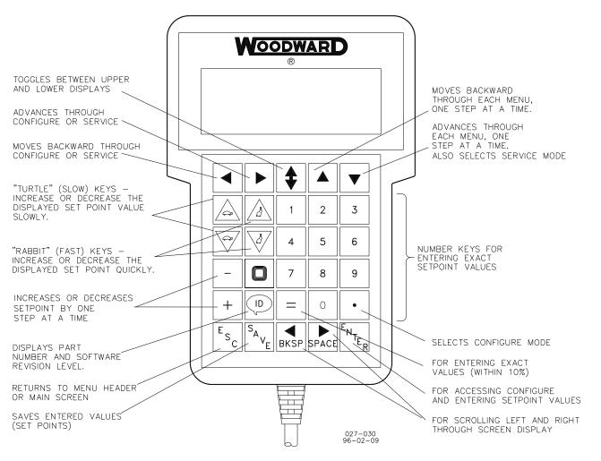
Figure 3-1. Hand Held Programmer Functions
