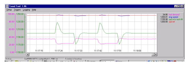
This trace shows results of just increasing Gain from 1.235 to 3.0. Gain Ratio and Window Width remain disabled. Peak rpm is reduced approximately 10–12 rpm.
