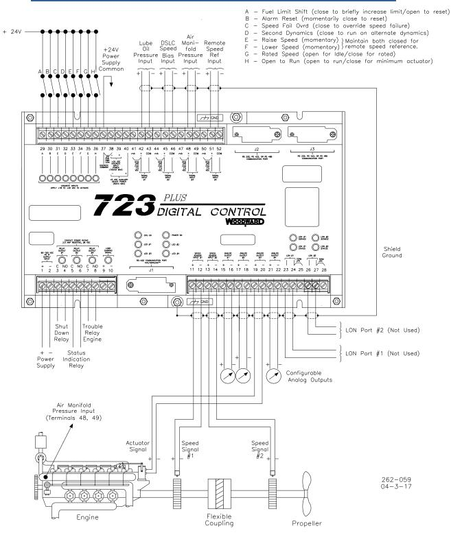
Figure 1-7. Typical 723PLUS Connections
