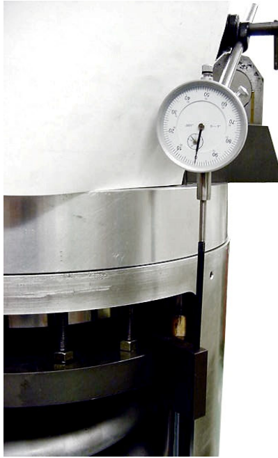
Figure 5-2. Stroke Measurement Attachment Bar
