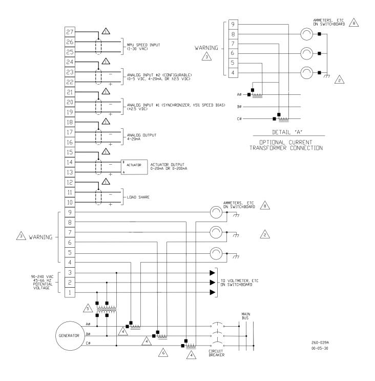
Figure 1-2a. 2301D Plant Wiring Diagram (sheet 1)
