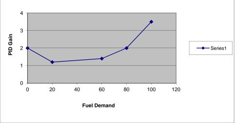
Figure 4-8. Linearized Gain Plot
