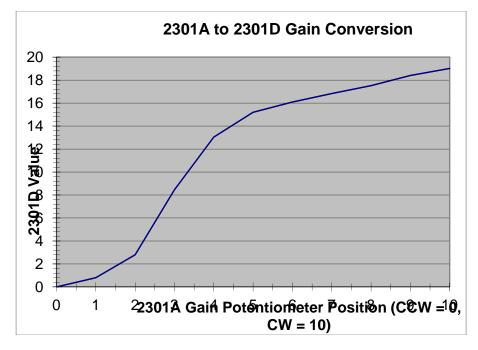
Figure B-1. Gain Potentiometer Conversion Chart
