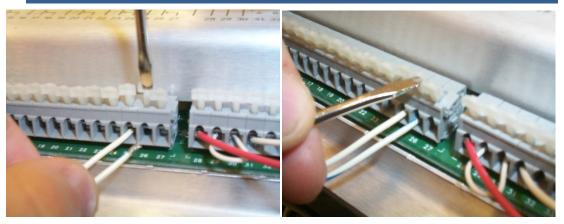
Figure 2-1. Installation of Wiring into Terminal
