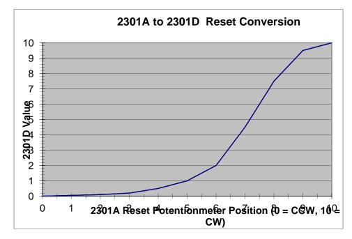
Figure B-2. Reset Potentiometer Conversion Chart
