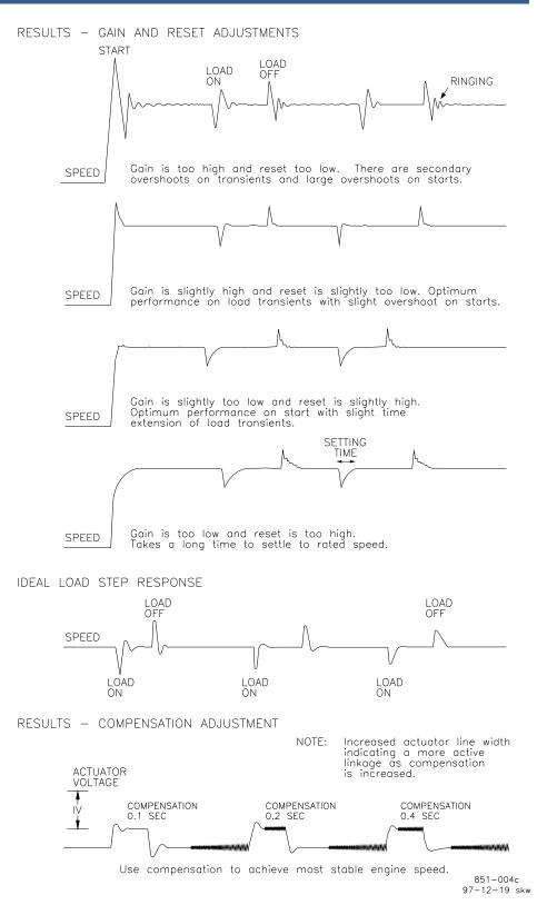
Figure 4-5. Typical Transient Response Curves
