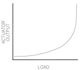
041-090 93-4-8 RAM Figure 4-6. Non-linear Valve Power Curve
