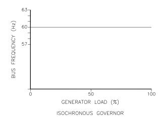
Figure 3-6. Isochronous Mode
