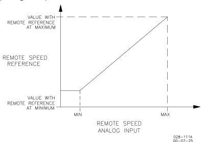
Figure 3-3. Remote Speed Reference
