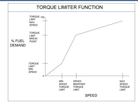
Figure 4-11. Torque Limiter Function
