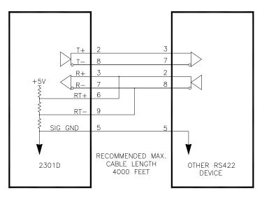
Figure 2-4. Typical RS-422 Communications Connections
