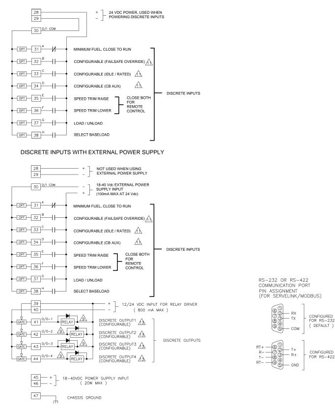
Figure 1-2b. 2301D Plant Wiring Diagram (sheet 2)
