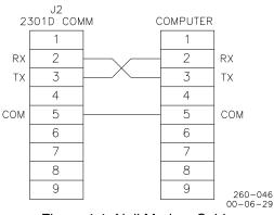
Figure 4-1. Null Modem Cable
