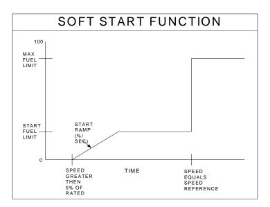
Figure 4-10. Soft Start Fuel Limit Function
