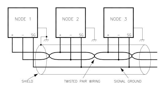
Figure 2-6. Preferred Multipoint Wiring Using Shielded Twisted-pair Cable with a Separate Signal Ground Wire
