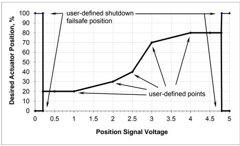
Figure 2-7. Analog 0–5 V Non-Linear Demand to Position
