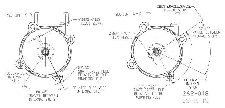
Figure 3-3b. L-Series Shaft Types
