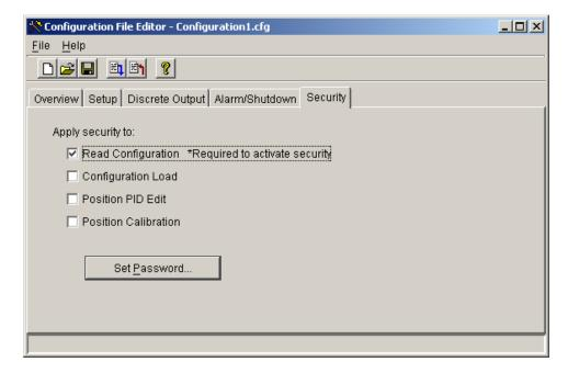
Figure 4-8. Configuration Editor— Security Tab
