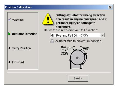
Figure 4-19. Service Tool—Manual Position Calibration
