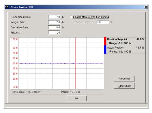
Figure 4-16. Service Tool—PID Tuning Window
