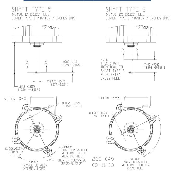
Figure 3-3c. L-Series Shaft Types
