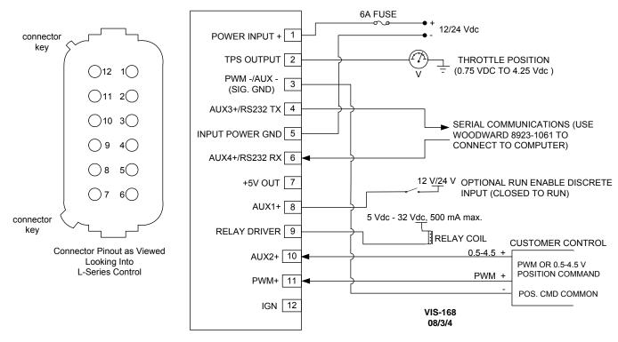
Figure 3-4. Typical L-Series Position Control Application Wiring
