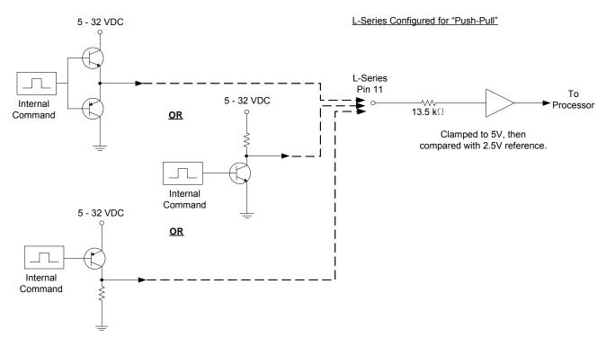
Figure 3-5. Acceptable PWM Input Types
