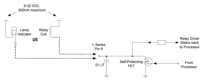
Figure 3-6. Relay Driver Output
