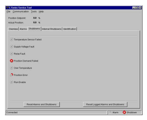
Figure 4-13. Service Tool – Shutdowns Tab
