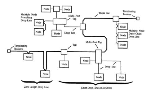
Figure 3-8 CAN System Wiring Example
