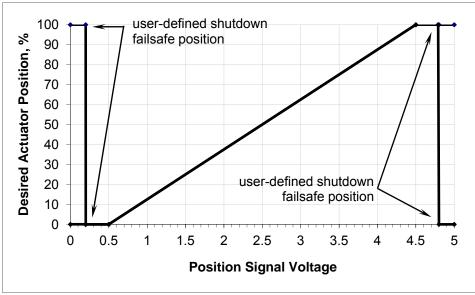
Figure 2-6. Analog 0–5 V Linear Demand to Position
