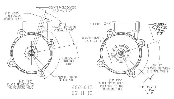
Figure 3-3a. L-Series Shaft Types
