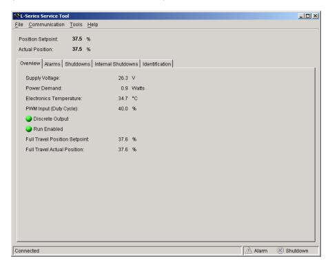
Figure 4-1. Example Service Tool Screen
