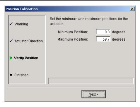
Figure 4-20. Service Tool—Manual Position Calibration Settings
