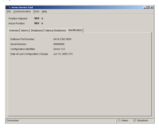
Figure 4-15. Service Tool—Identification Tab
