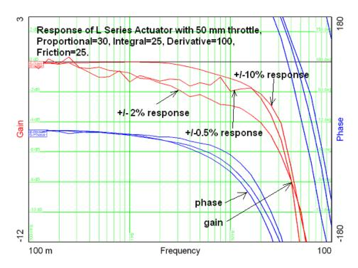
Figure C-1. Bode Plot of L-Series Response
