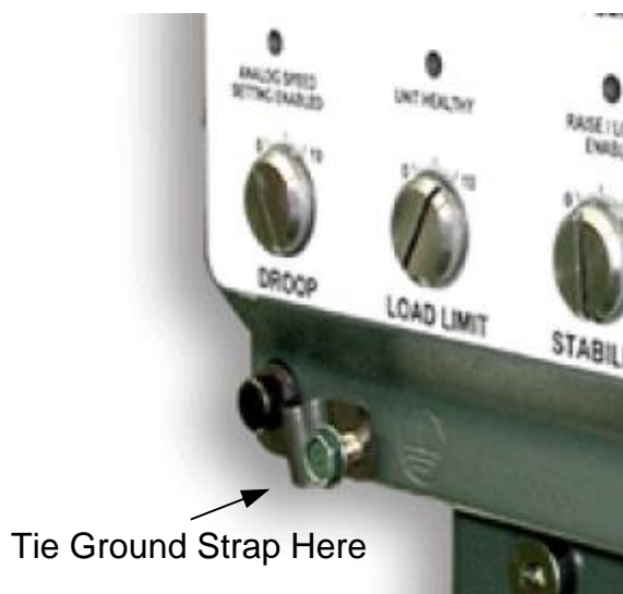
Figure 3-1. Location of Ground Strap
