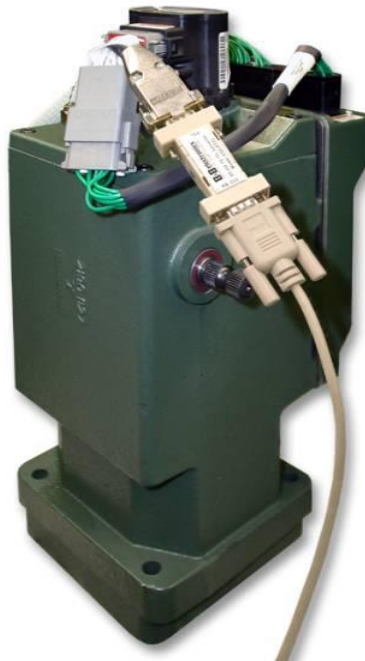
Figure 5-2a. Programming Harness Connection
