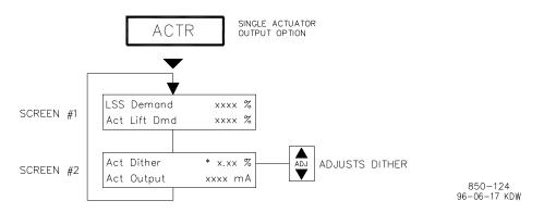
The asterisk (\*) denotes a tunable parameter. To adjust this parameter the "@" symbol must be on the display line containing the asterisk. The @ symbol is moved with the SELECT key.
