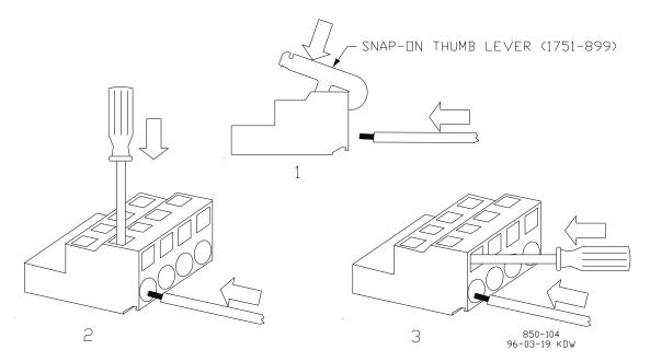
Figure 2-5. CageClamp Terminal Blocks
