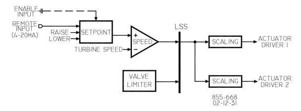
Figure 1-4. Single or Split-Range Turbine Configurations (Speed PID with Remote Set Point)
