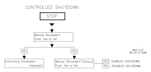
The speed setpoint moves to the minimum (zero) at the fast rate. Once at the minimum, the valve limiter moves to its minimum position. At the minimum valve limiter position, a trip is issued. The shutdown relay will de-energize and the actuator outputs are pulled to zero. The front panel displays the following:
