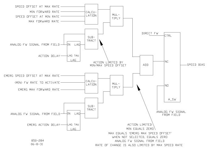
Figure 3-11. Typical Anti-surge Valve and Speed Feed-Forward Logic Trend
