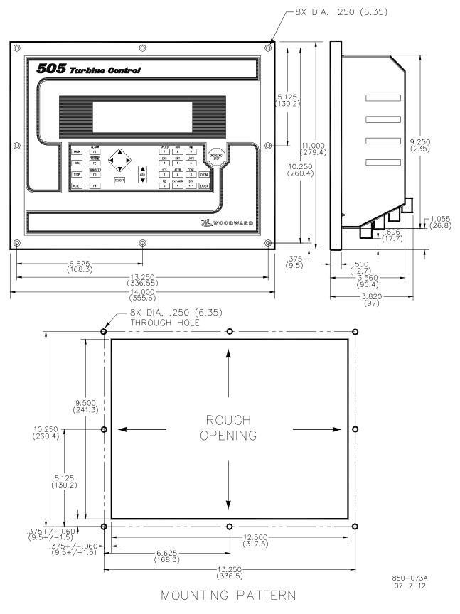
Figure 2-1. 505 Control Layout (Standard Enclosure)
