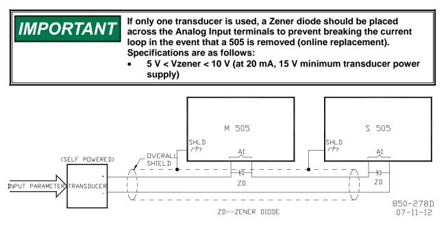
Figure 2-15j. One Transducer Driving Both 505 Inputs
