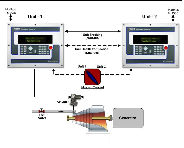
Figure 3-14. Redundant 505 Configuration Diagram
