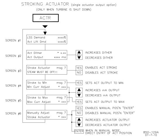
Screen 3 shown only when the unit is shut down. Screens 4, 5, & 6 shown only when Stroke Actuator is set to YES.
