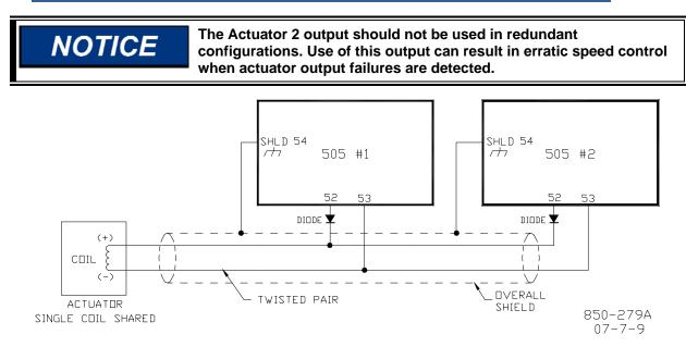
Figure 2-15k. Single Shared Coil Applications
