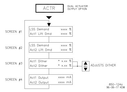
The asterisk (\*) denotes a tunable parameter. To adjust this parameter the "@" symbol must be on the display line containing the asterisk. The @ symbol is moved with the SELECT key.
