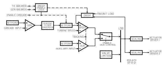
Figure 1-6. Single or Split-Range Turbine Configurations (Auxiliary PID Configured as a Controller)
