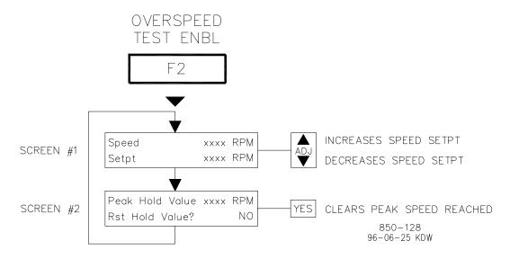
Figure 5-6. Overspeed Test Enable Key Screens
