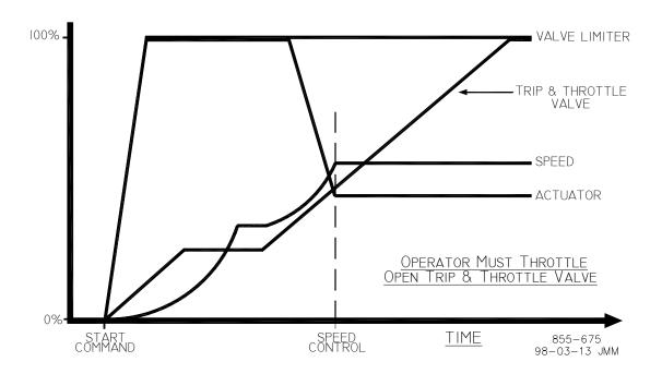
Figure 3-1. Manual Start Mode Example
