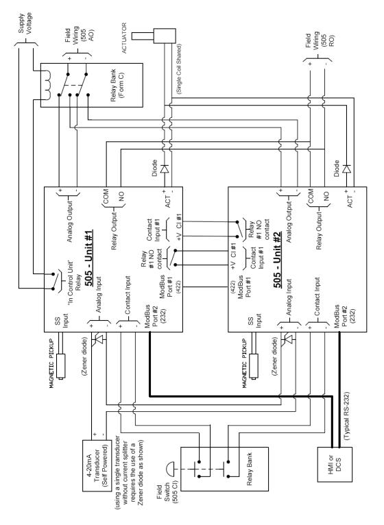
Figure 2-15b. Typical Redundant Diagram
