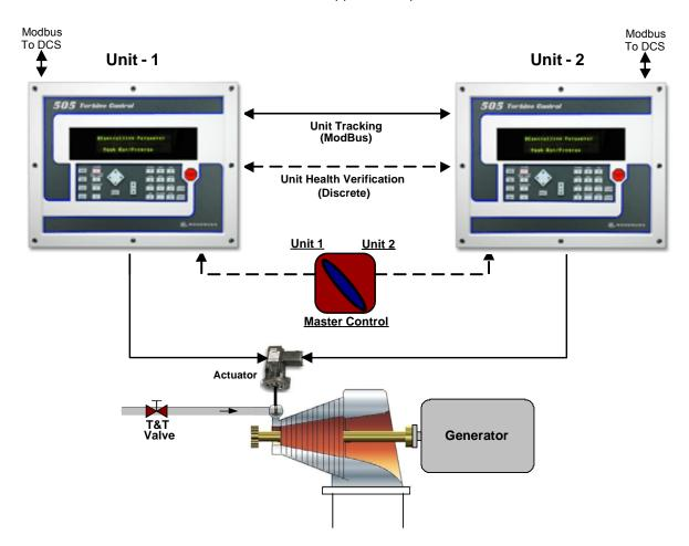
Figure 1-7. Typical Redundant 505 Application Configuration
