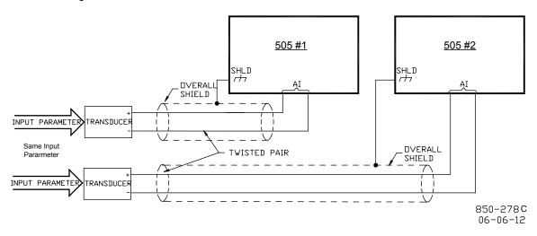
Figure 2-15h. Two Transducers with One Transducer for each 505 Unit
