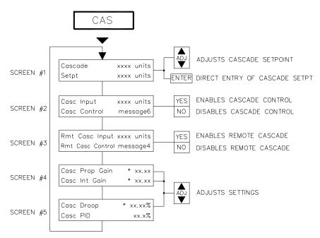
Screen 3 shown only if Remote Cascade control is configured. Screen 4 shown only if dynamics adjustments are used.
