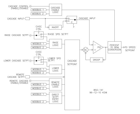
Figure 3-12. Cascade Functional Diagram
