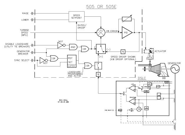
Figure 3-10. Load Sharing Logic
