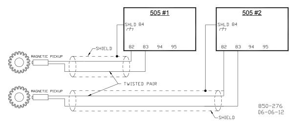
Figure 2-15c. Optional Speed MPU Input Diagram – Different Probes
