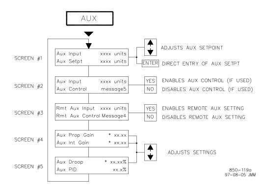
Screen 3 shown only if Remote Auxiliary control is configured. Screen 4 shown only if dynamics adjustments are used.
