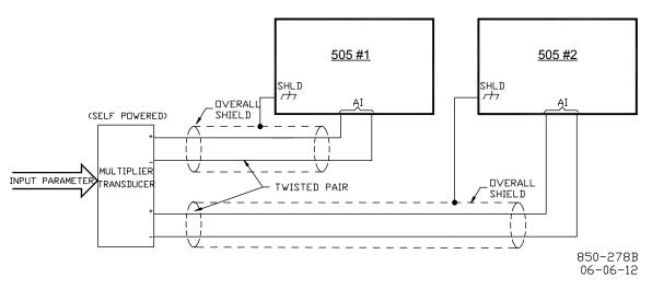
Figure 2-15i. One Transducer Using a Current Splitting/Isolation Device
