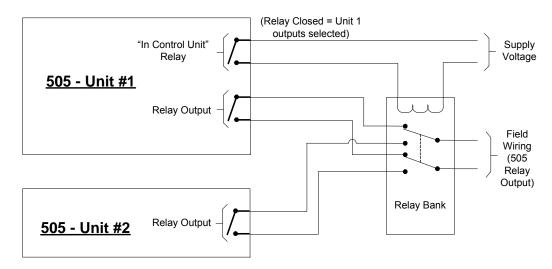
Figure 2-15p. Relay Output Switching Diagram
