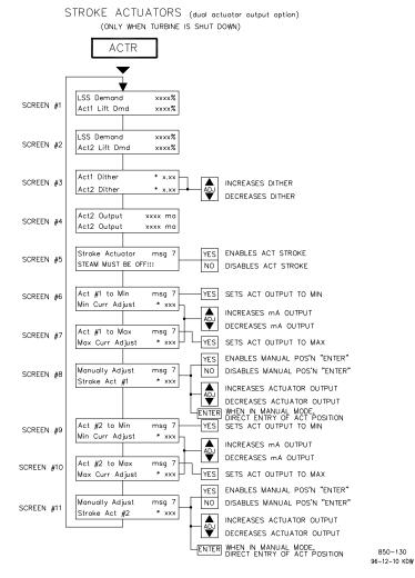
Screen 5 shown only when the unit is shut down. Screens 6-11 shown only when Stroke Actuator is set to YES.
