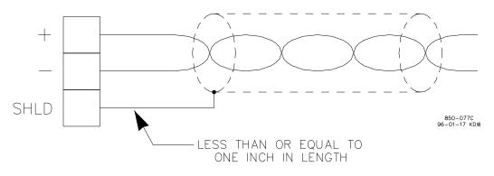
Figure 2-9. Shielded Wire Connections
