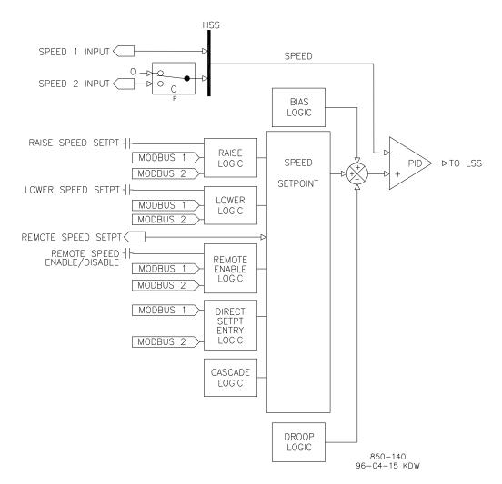
Figure 3-6. Speed Control Functional Diagram
