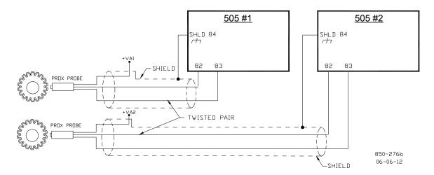
Figure 2-15e. Recommended Proximity Probe Input Diagram – Different Probes
