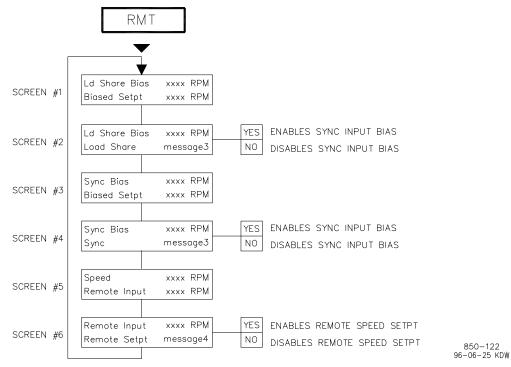
Screens 1 & 2 are shown only if Load Sharing control or Sync/Ld Sharing is configured. Screens 3 & 4 are shown only if Synchronizing is configured and Load Sharing is not. Screens 5 & 6 are shown only if Remote speed Setting control is configured.
