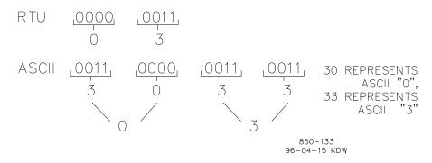
Figure 6-1. ASCII/RTU Representation of 3
