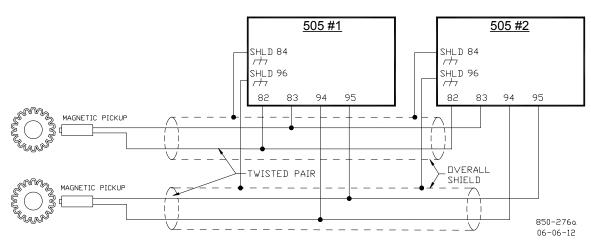
The above installation depicts individual MPU for each 505 in redundant configuration. The second input on both the 505 can be driven in the same manner utilizing separate MPU or a common MPU as desired.
