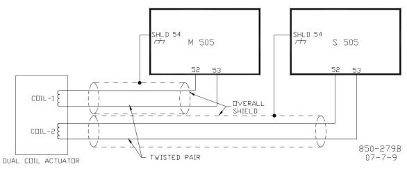
Figure 2-15I. Dual Coil Applications
