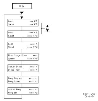
• Screen 1 shown only if a KW analog input is programmed and input is not failed.
