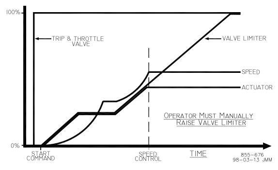
Figure 3-2. Semiautomatic Start mode Example
