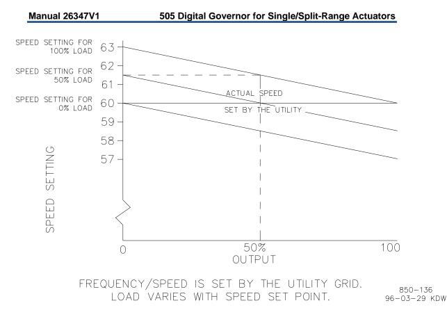
Figure 3-8. Frequency and Unit Load Relationship
