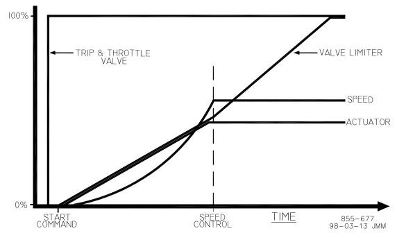
Figure 3-3. Automatic Start Mode Example
