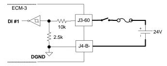
Figure 2-20. Sourcing Input Wiring Diagram
