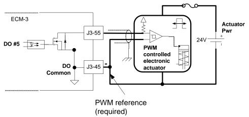
Figure 2-24. PWM Output Wiring Diagram for General Application
