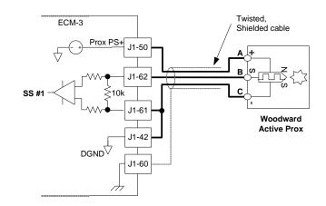
Figure 2-10. Proximity Sensor Wiring Diagram
