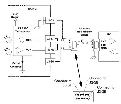
Figure 2-29. RS-232 Wiring Diagram
