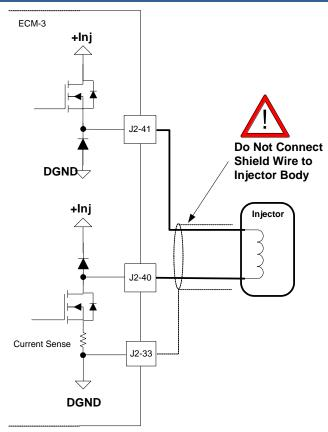
Figure 2-28. Fuel Injection Output Wiring Diagram
