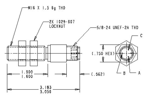
Figure C-2. Metric Proximity Sensor
