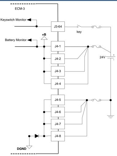
Figure 2-4. Input Power Wiring Diagram
