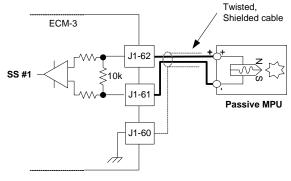
Figure 2-6. MPU Wiring Diagram
