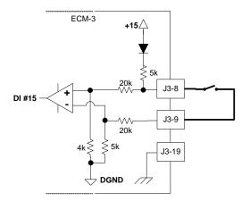
Figure 2-19. Boolean Input Wiring Diagram
