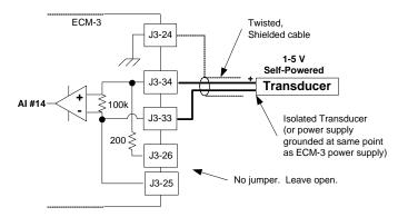
Figure 2-13. Voltage Input Wiring Diagram: Self-Powered
