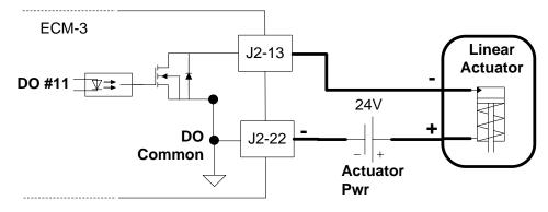
Figure 2-25. PWM Output Wiring Diagram for Linear Actuator
