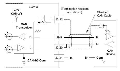
Figure 2-34a. CAN-2 and CAN-3 Wiring Diagram
