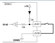
Figure 2-21. Sinking Input Wiring Diagram
