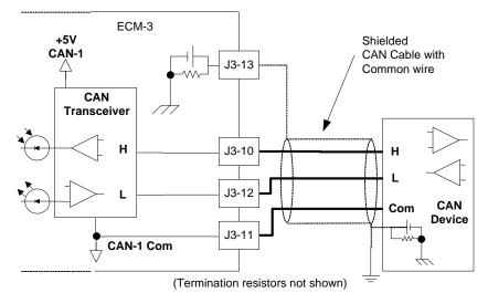
Optimal solution where appropriate wire can be used
