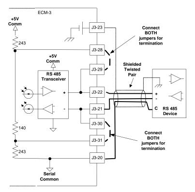
Figure 2-30. RS-485 Wiring Diagram
