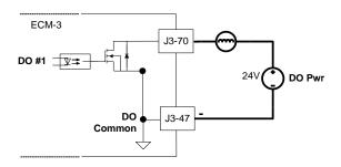
Figure 2-26. Boolean Output Wiring Diagram
