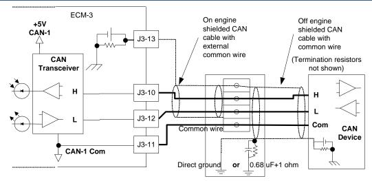
On Engine to Off Engine Cabling Interface with two shield grounding options
