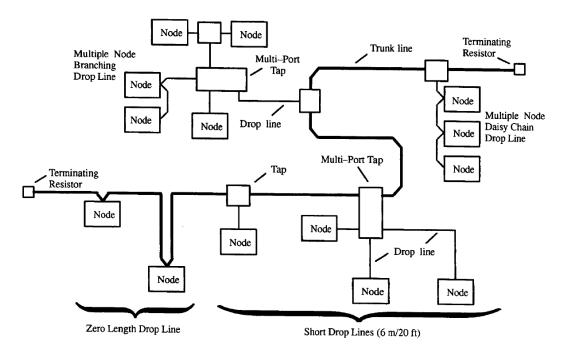
Figure 2-32. CAN System Wiring Example
