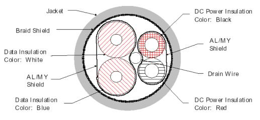
Figure 2-31. CAN Cable Cross-Section
