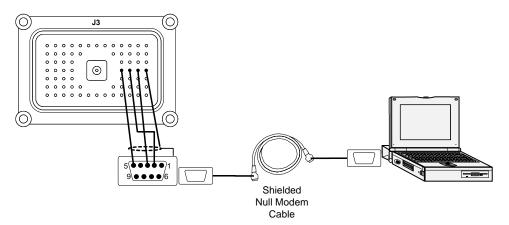
Figure 4-1. Connecting the ECM3 to a PC
