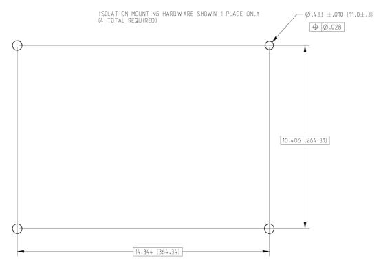
Figure 2-2. Mounting Hole Layout
