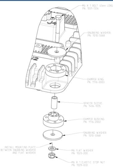
Figure 2-1. Vibration Isolator Installation
