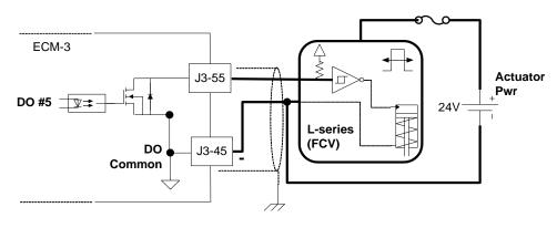
Figure 2-22. PWM Output Wiring Diagram for L-Series, FCV, Flo-Tech
