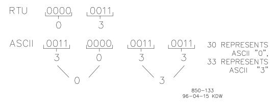
Figure 3-1. ASCII/RTU Representation of 3
