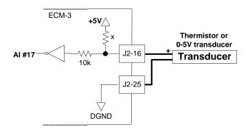
Figure 2-15. Temperature Sensor Analog Input Wiring Diagram
