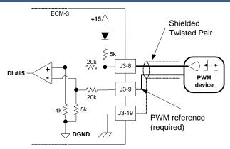
Figure 2-18. PWM Input Wiring Diagram
