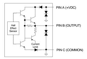
Figure C-1. Prox Sensor Schematic
