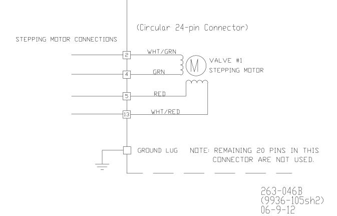
Figure 3-1. Valve Wiring Diagram
