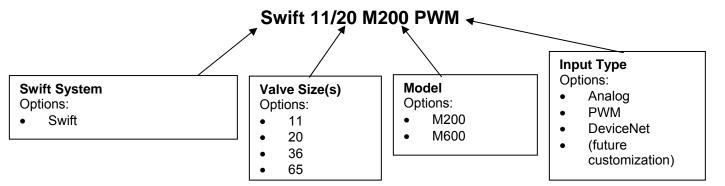
There are four parts to identify a Swift valve: the **system** (Swift), the **valve size** (11, 20, 36, 65), the **model** (M200, M600), and the **input type** (analog, PWM, DeviceNet). These are explained on the next page.
