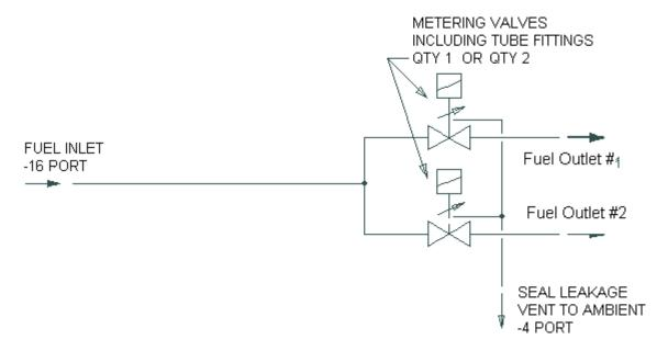
Figure 1-4. Swift Valve Schematic
