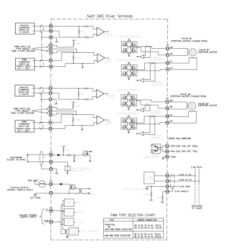
Figure 3-5. Representative I/O Schematic
