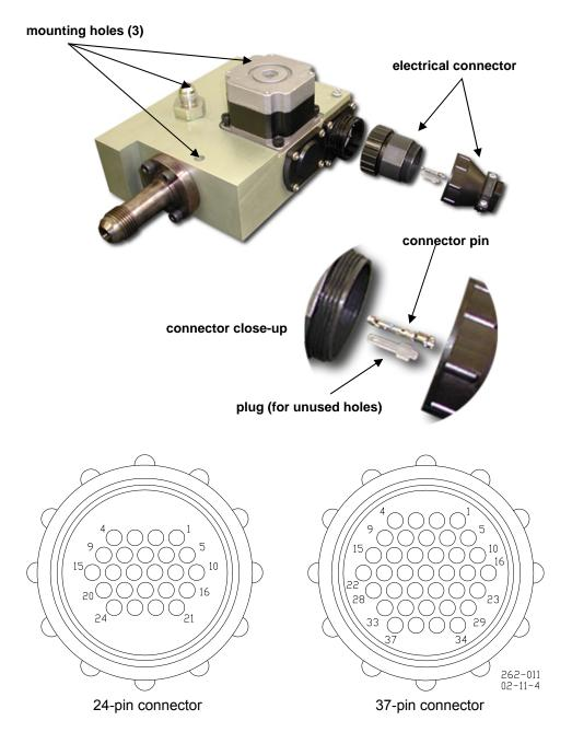
Figure 3-2. Swift Valve Wiring Assembly Overview
