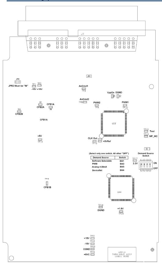
Figure 3-6. Internal Driver Test Points and Switches
