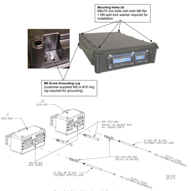
Figure 3-3. Driver Wiring Assembly Overview
