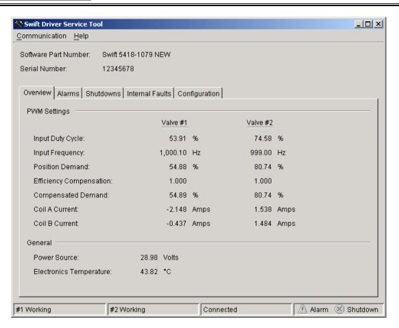
Figure 7-1. Example Service Tool Screen
