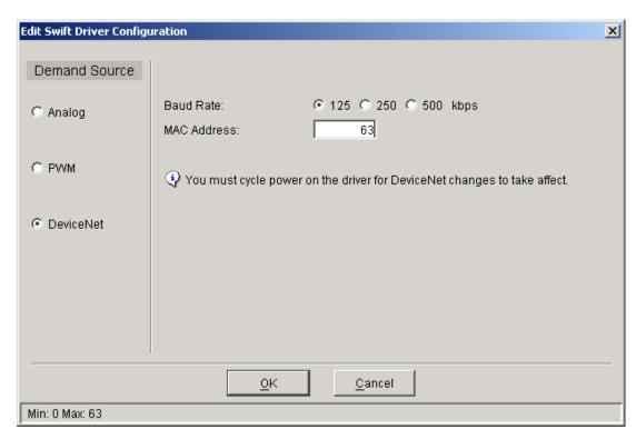
Figure 7-3c. Configuration Editor—DeviceNet Settings
