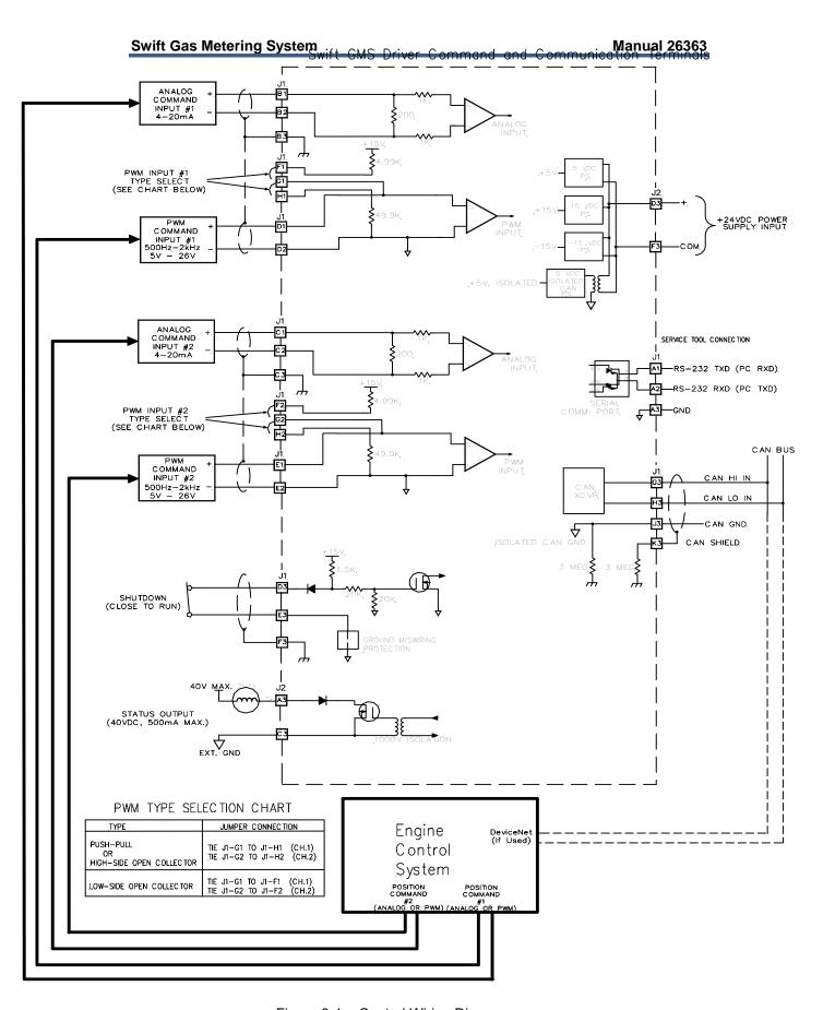
Figure 3-1a. Control Wiring Diagram
