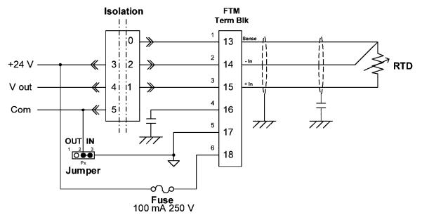
Figure 5-6. Example Wiring Diagram—RTD to Dataforth FTM
