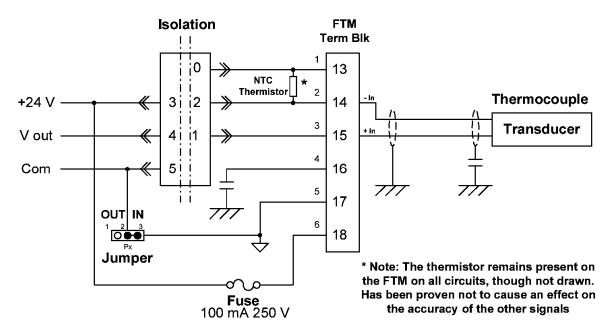
Figure 5-5. Example Wiring Diagram—Thermocouple to Dataforth FTM
