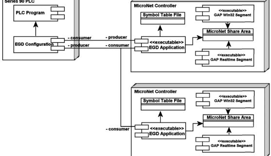
Figure 6-1. Communication Schematic
