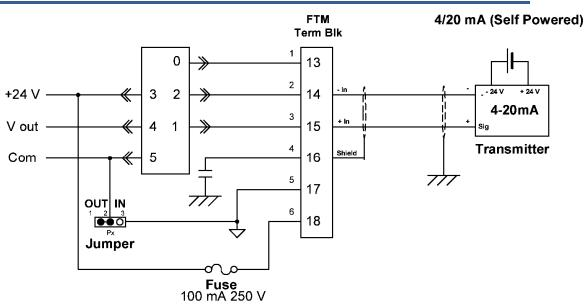
Figure 5-8. Example Wiring Diagram - Self-powered 4–20 mA Signal to Dataforth FTM
