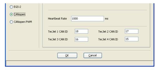
Figure 5-13c. Edit TecJet Configuration, CANopen
