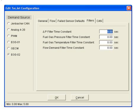
Figure 5-12. Edit TecJet Configuration, Filters
