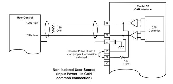
Figure 2-3. TecJet 52 CAN Wiring for Isolated/Non-isolated Systems
