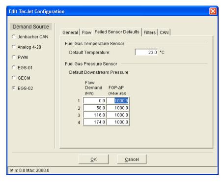
Figure 5-11. Edit TecJet Configuration, Failed Sensor Defaults
