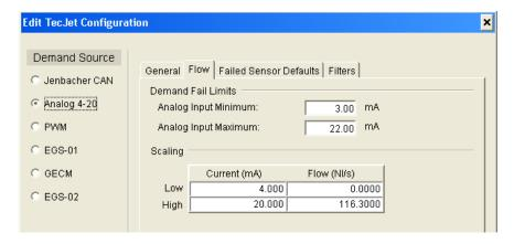
Figure 5-10b. Edit TecJet Configuration, Flow (Analog Demand)
