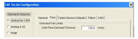
Figure 5-10a. Edit TecJet Configuration, Flow (CAN Demand)
