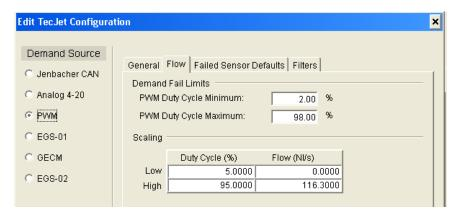
Figure 5-10c. Edit TecJet Configuration, Flow (PWM Demand)
