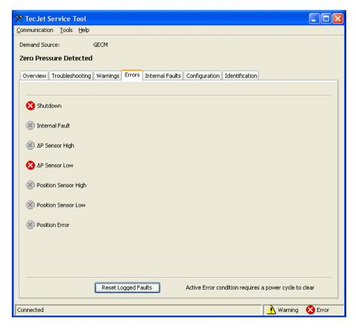
Figure 5-5a. Errors Screen Before Power Cycle
