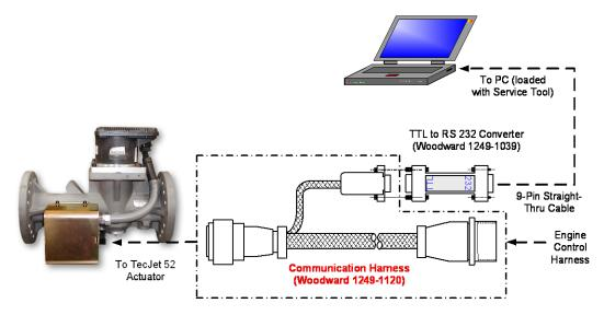
Figure 5-1. Communication- Harness Connections
