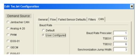
Figure 5-13b. Edit TecJet Configuration, CAN (User Configured)
