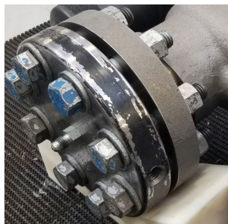
Figure 3-2. Illustration of Raised Face Style Diverging Sleeve
