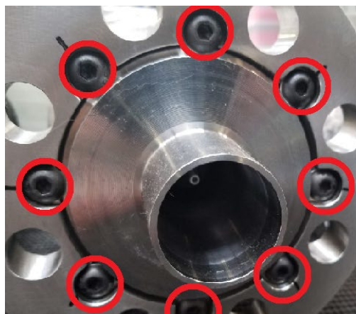
Figure 3-1. Illustration of Diverging Sleeve Screws
