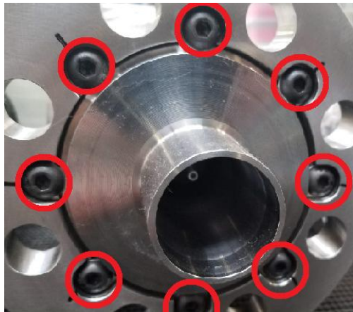
Figure 3-1. Illustration of Diverging Sleeve Screws
