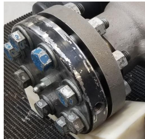
Figure 3-2. Illustration of Raised Face Style Diverging Sleeve
