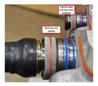
Figure 3-6. ID Module/Shaft Resolver Actuator Connector
