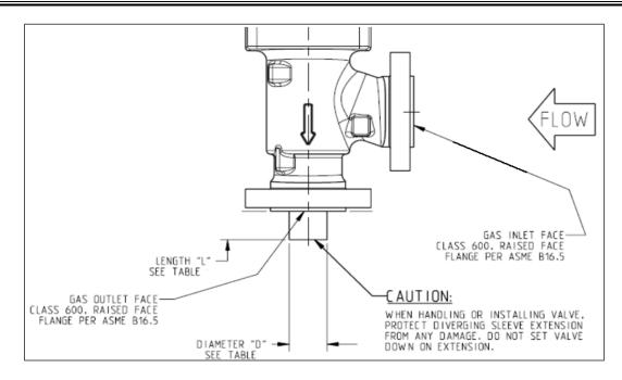
Figure 1-9. Representative Outline Deviation of High Recovery Valves
