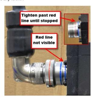
Figure 3-5. Motor Resolver Connectors
