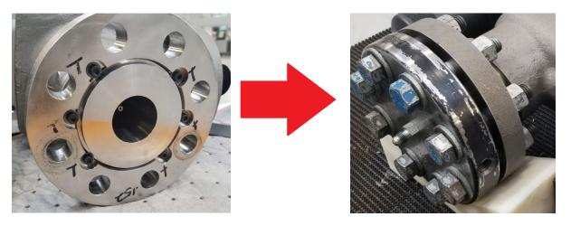
Figure 3-2. Illustration of Raised Face Style Diverging Sleeve
