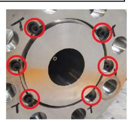
Figure 3-1. Illustration of Diverging Sleeve Screws
