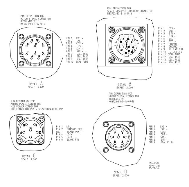
Figure 1-10. Connector Pin-outs
