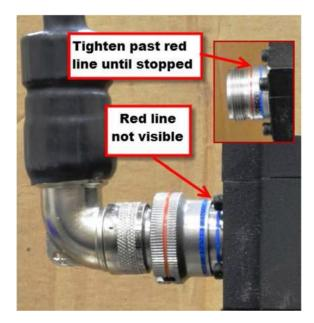
Figure 3-5. Motor Resolver Connectors
