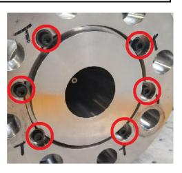
Figure 3-1. Illustration of Diverging Sleeve Screws
