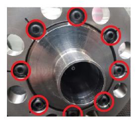
DIVERGING SLEEVE SCREWS -DO NOT PRESSURE LOAD!
