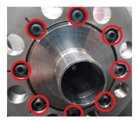
DIVERGING SLEEVE SCREWS -DO NOT PRESSURE LOAD!
