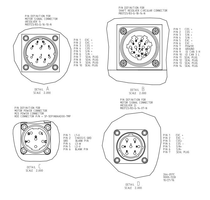
Figure 1-10. Connector Pin-outs
