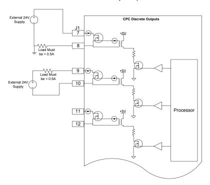
Figure 3-11. Discrete Output Connections
