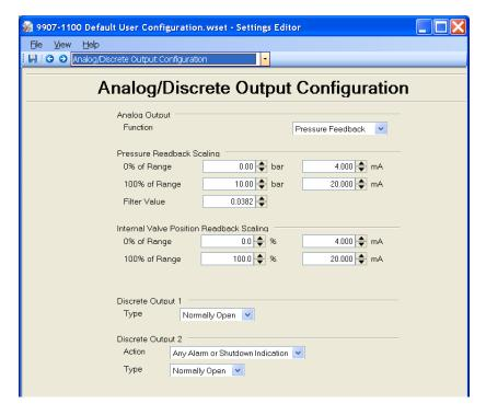
Figure 6-8. PC Service Tool Analog/Discrete Output Configuration
