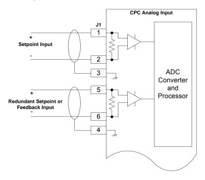
Figure 3-7. Analog Input Connections
