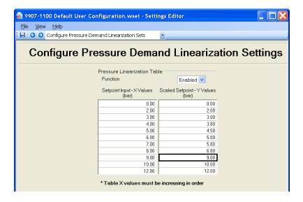
Figure 6-10. PC Service Tool Demand Linearization Configuration
