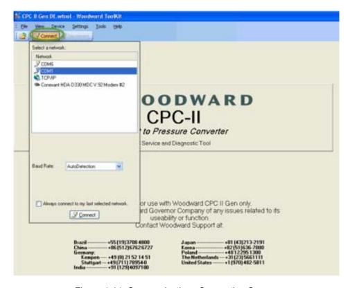
Figure 4-14. Communications Connection Screen
