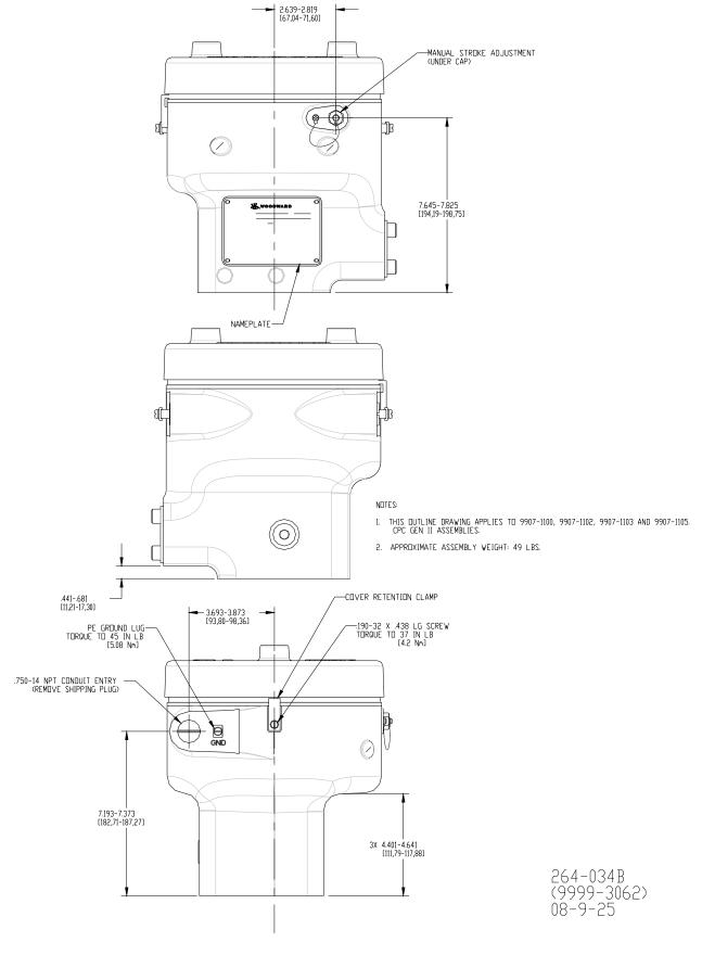
Figure 2-3b. Installation Drawing
