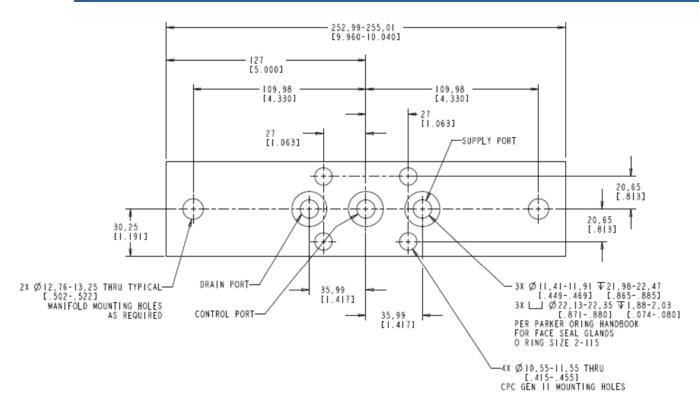
Figure 3-1. Example CPC-II Manifold Dimensions
