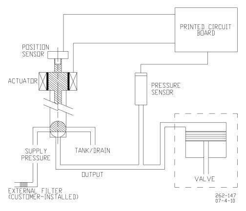
Figure 1-2. Example System Schematic
