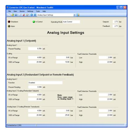
Figure 5-5. PC Service Tool Analog Input Settings
