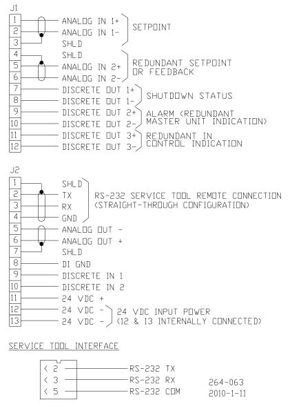
Figure 3-2. Wiring Diagram
