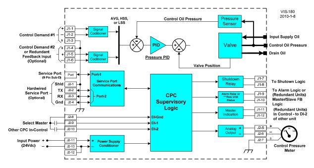
Figure 1-3. Example Functional Diagram (CPC electronics)
