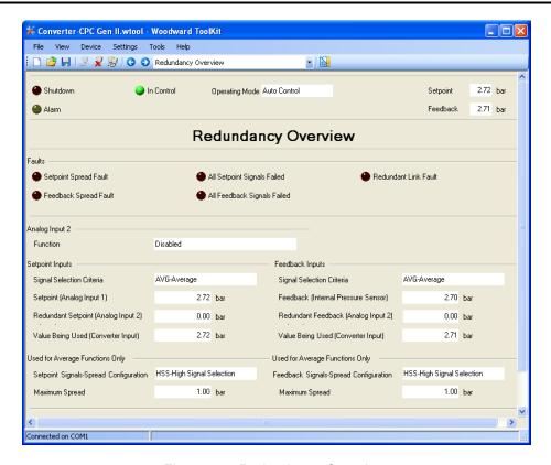
Figure 5-4. Redundancy Overview
