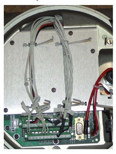
Figure 3-6. Recommended Wiring Strain Relief
