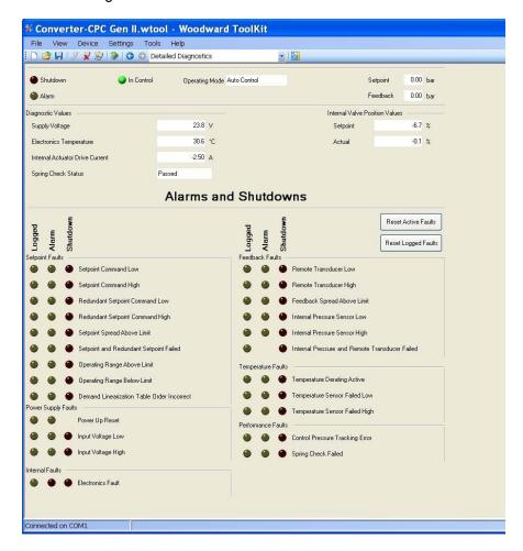
Figure 5-8. PC Service Tool Detailed Diagnostics Screen
