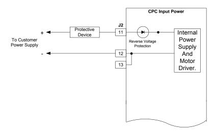
Figure 3-4. Power Supply Input Connections
