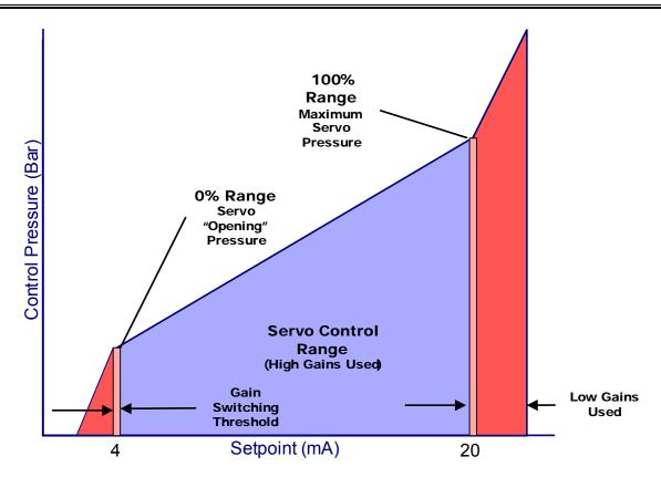
Figure 6-7. Analog Input Setpoint Scaling
