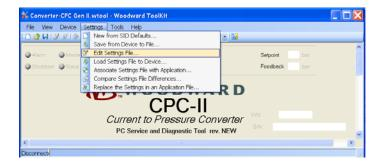
Figure 6-2. Loading the Settings File to the Device
