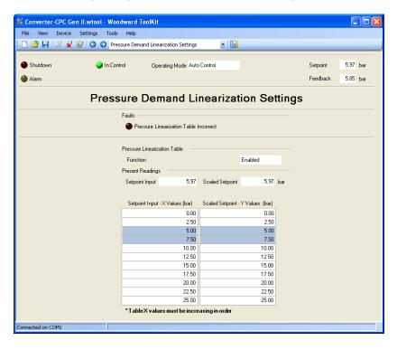
Figure 5-7. PC Service Tool Demand Linearization Settings
