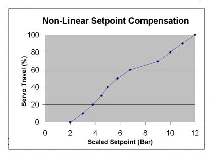
Figure 6-9. PC Service Tool Demand Linearization Configuration
