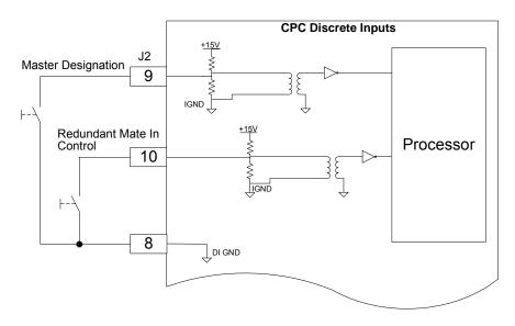
Figure 3-10. Discrete Input Connections
