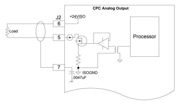
Figure 3-9. Analog Output Connections
