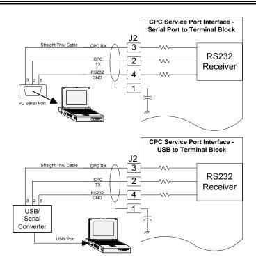
Figure 4-1. Service Port Connections
