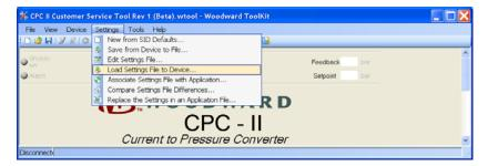
Figure 6-3. Loading the Settings File to the Device
