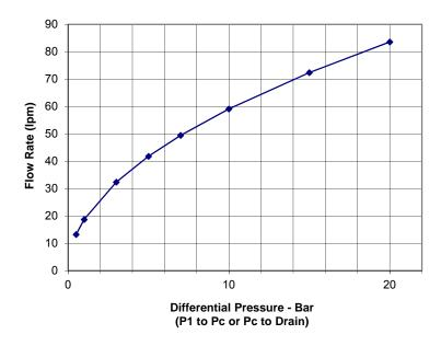
Figure 2-2. Maximum Flow Capacity
