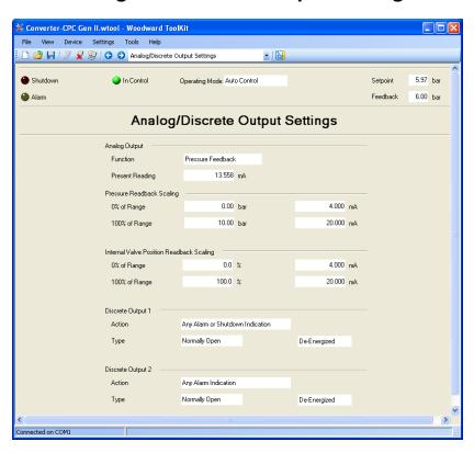
Figure 5-6. PC Service Tool Analog/Discrete Output Settings
