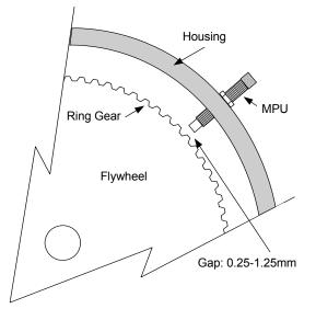
Figure 4-10. Magnetic Pickup Mounting in Flywheel Housing
