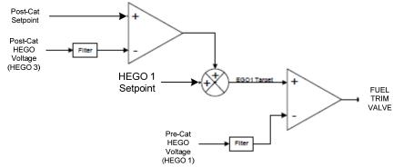
Figure 2-4. Basic Control Logic for Post-Catalyst HEGO Control
