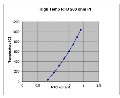
Figure 3-49. Catalyst RTD Voltage vs Temperature (°F)
