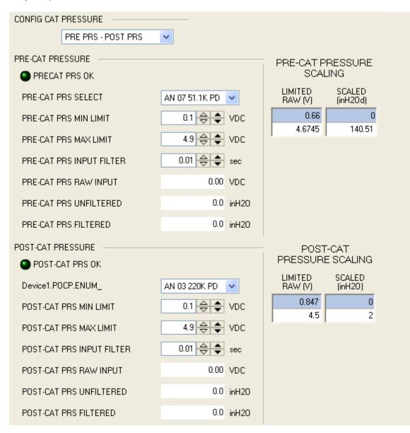
Figure 3-51b. Catalyst Pressure Monitoring & Protection Settings (PRE PRS – POST PRS Option, HMI Screen 6.13)
