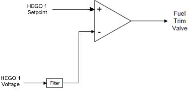
Figure 2-3. Basic Control Logic for Pre-catalyst EGO Control
