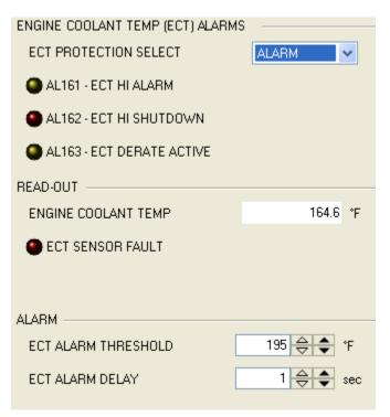
Figure 3-45a. Example HMI Settings for ALARM Protection (HMI Screen 4.6)
