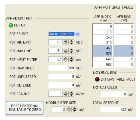
Figure 3-22. AFR Bias Signal Configuration (HMI Screen 6.11)
