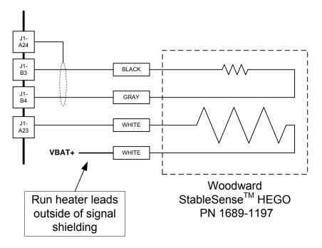
Figure 4-15. StableSense HEGO Sensor Wiring Diagram
