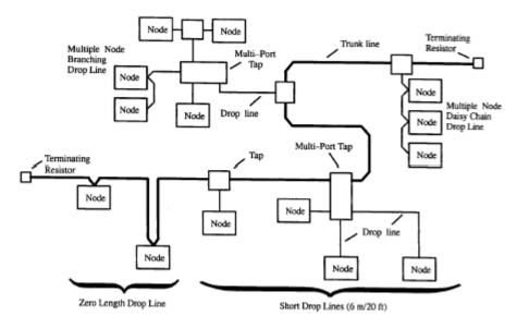
Figure 4-8. CAN System Wiring Example
