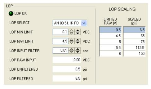
Figure 3-13. LOP Signal Configuration (HMI Screen 6.10)
