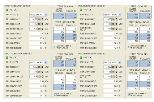
Figure 5-1. HMI Settings for TPS and FTPS (HMI Screen 6.9)
