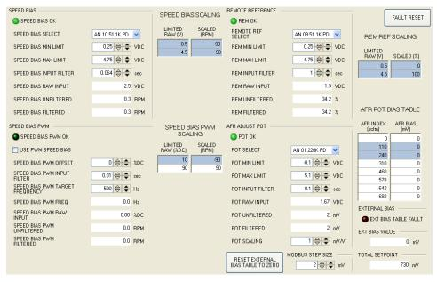
Figure 5-4. HMI Settings for EXTERNAL BIAS (HMI Screen 6.9)
