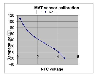
Figure 3-10. MAT Sensor Calibration
