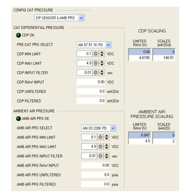
Figure 3-51c. Catalyst Pressure Monitoring & Protection Settings (DP SENSOR & AMB PRS Option, HMI Screen 6.13)
