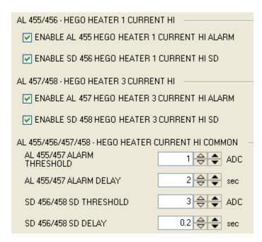
Figure 3-55. HEGO Heater Alarm & Shutdown Settings AL 455 – AL 458 (HMI Screen 7.8)
