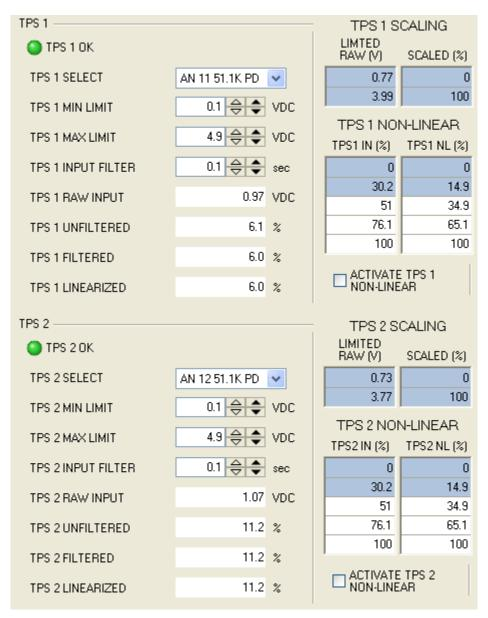
Figure 3-15a. TPS 1 & TPS 2 Signal Configuration (HMI Screen 6.8)
