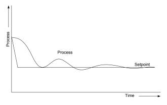
Figure 5-22b. Integral Action Optimum Curve
