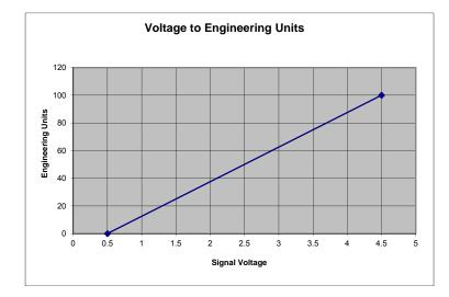
Figure 3-4. Input voltage to Engineering Units
