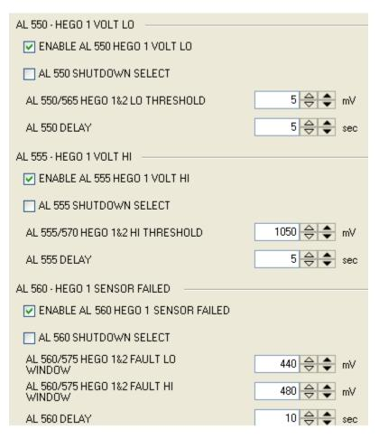
Figure 3-56a. HEGO Alarm & Shutdown Settings AL 550 – AL 560 (HMI Screen 7.10)
