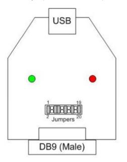
Figure 4-6. EasySync RS-485 to USB Adapter
