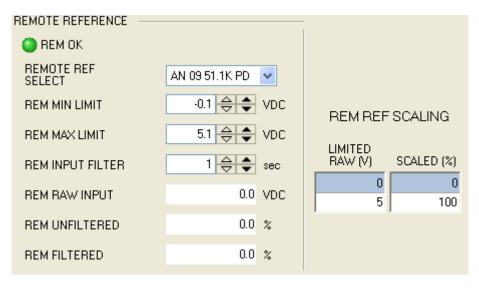
Figure 3-3. Remote Reference Signal Configuration (HMI Screen 6.11)
