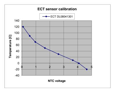
Figure 3-12. ECT Sensor Voltage vs Temperature (°C)
