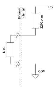
Figure 3-9. Analog Input Circuit – Resistance Temperature Sensors
