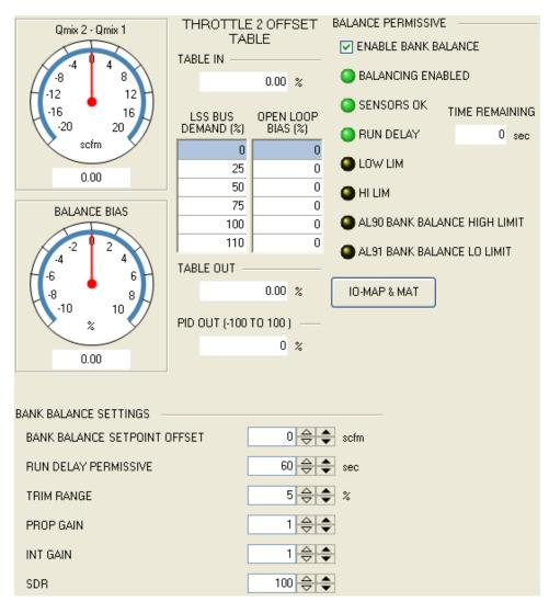
Figure 3-40. Bank Balancing Settings (HMI Screen 2.0)
