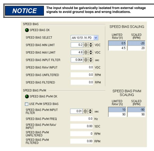
Figure 3-14. Speed Bias Signal Configuration (HMI Screen 6.11)
