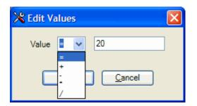
Figure 3-71. Selecting an Operator to Modify Table Values
