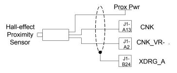
Figure 4-12. Proximity Sensor Wiring – Speed Sensor
