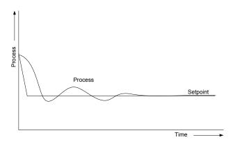
Figure 5-23b. Derivative Action Optimum Curve
