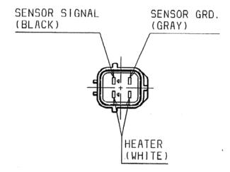
Figure 4-16. StableSense HEGO Sensor Connector Wiring Diagram looking into the connector.
