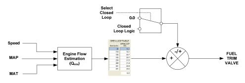
Figure 2-5. Basic Control Logic Open Loop Feed-Forward
