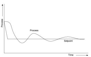
Figure 5-22a. Integral Action Too High Curve
