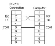
Figure 5-14. IC-900 Series Service Tool Connection Schematic
