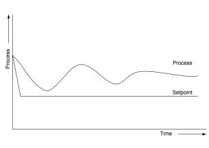
Figure 5-21b. Proportional Gain Optimum Curve
