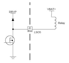
Figure 4-17. LSO Wiring Output Diagram (Alarm Relay shown)
