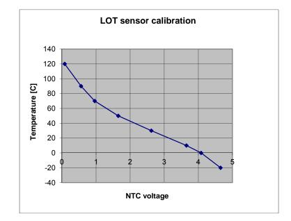
Figure 3-19. LOT Sensor Voltage vs Temperature (°C)
