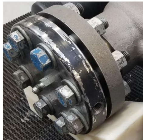
Figure 3-2. Illustration of Raised Face Style Diverging Sleeve
