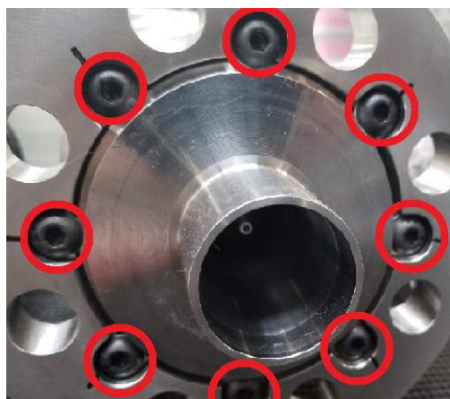
Figure 3-1 Illustration of Diverging Sleeve Screws
