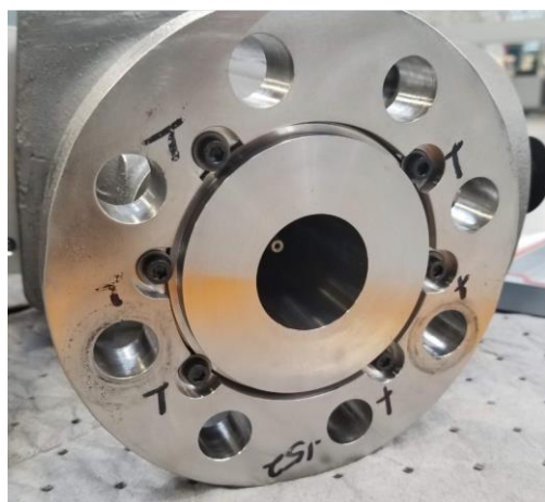
Figure 3-2. Illustration of Raised Face Style Diverging Sleeve
