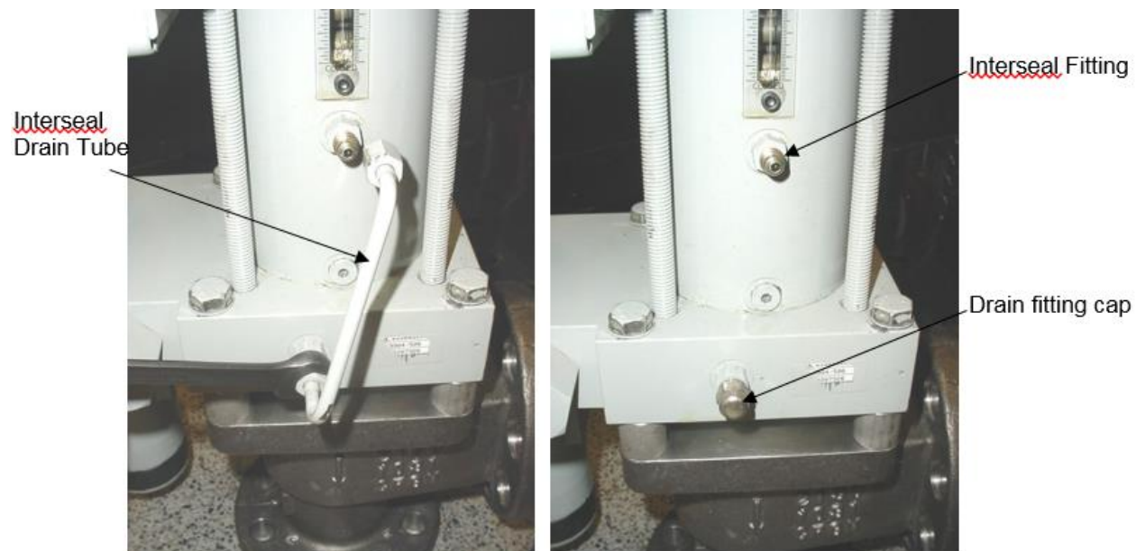
Figure 4-2. Location of Hydraulic Interseal Drain and Cap for 2 Inch Valves
