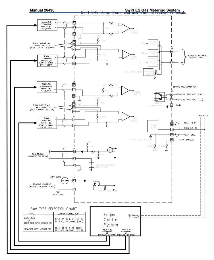
Figure 3-1a. Control Wiring Diagram
