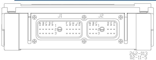
Figure 3-4. Driver Connector Pin Locations (viewed looking at the driver housing)
