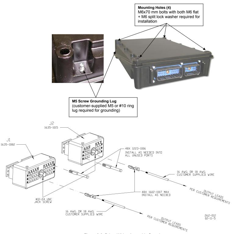
Figure 3-3. Driver Wiring Assembly Overview
