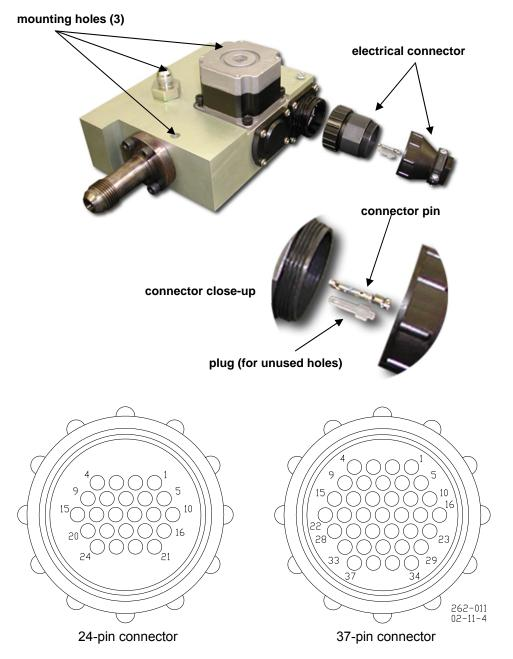
Figure 3-2. Swift Valve Wiring Assembly Overview
