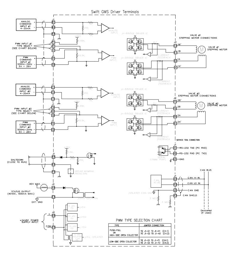
Figure 3-5. Representative I/O Schematic
